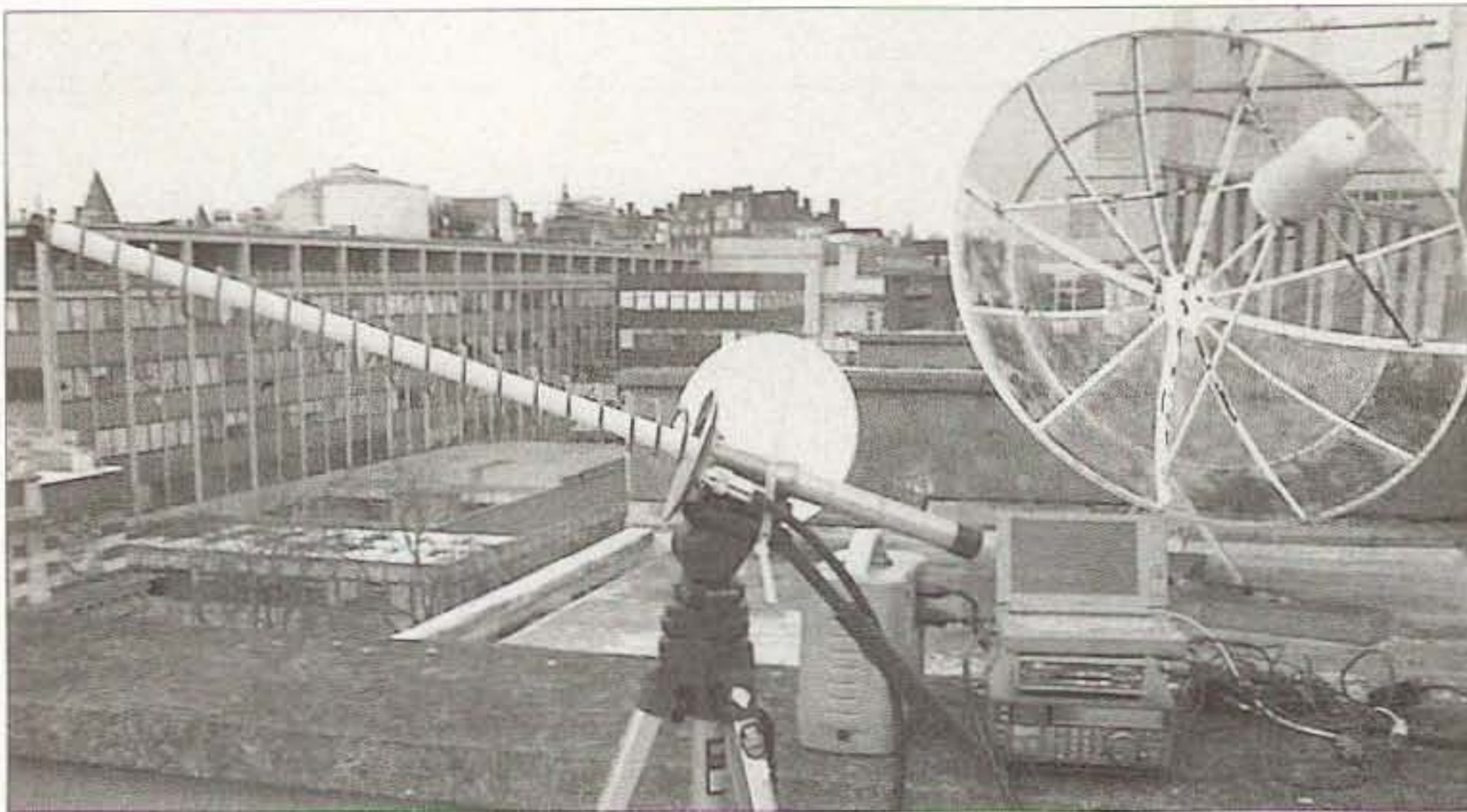
Photo B. The helical antenna has only one active element which is wound in a spiral fashion. A small reflector is mounted at the rear of the antenna to radiate the RF wave forward and in a circular motion around the shape of the helical.
