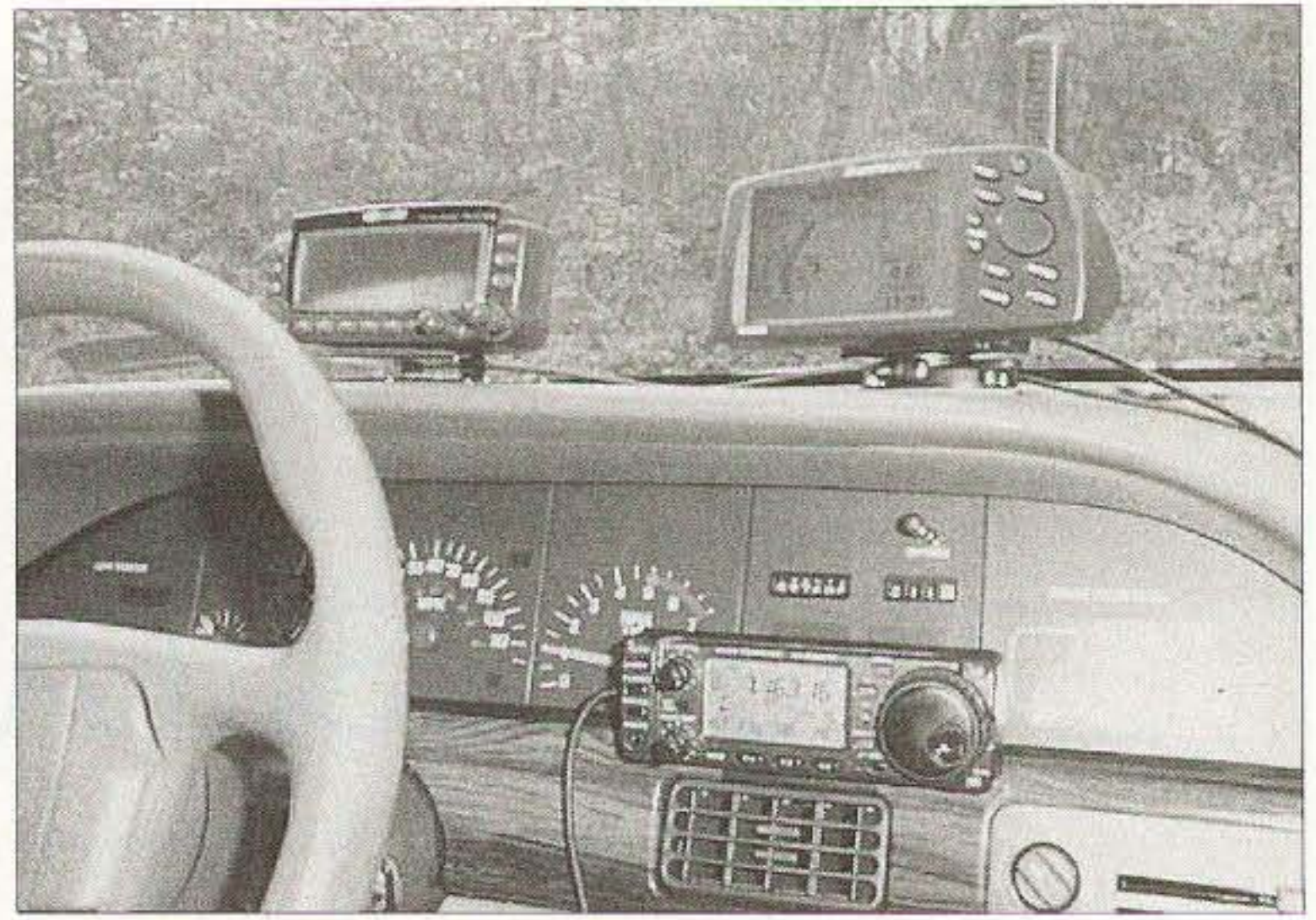
Photo D. Chas Richard W4HFZ's mobile APRS satellite capability (including HF). With an APRS satellite, he can send and receive brief text messages anywhere on the planet a few times a day.
