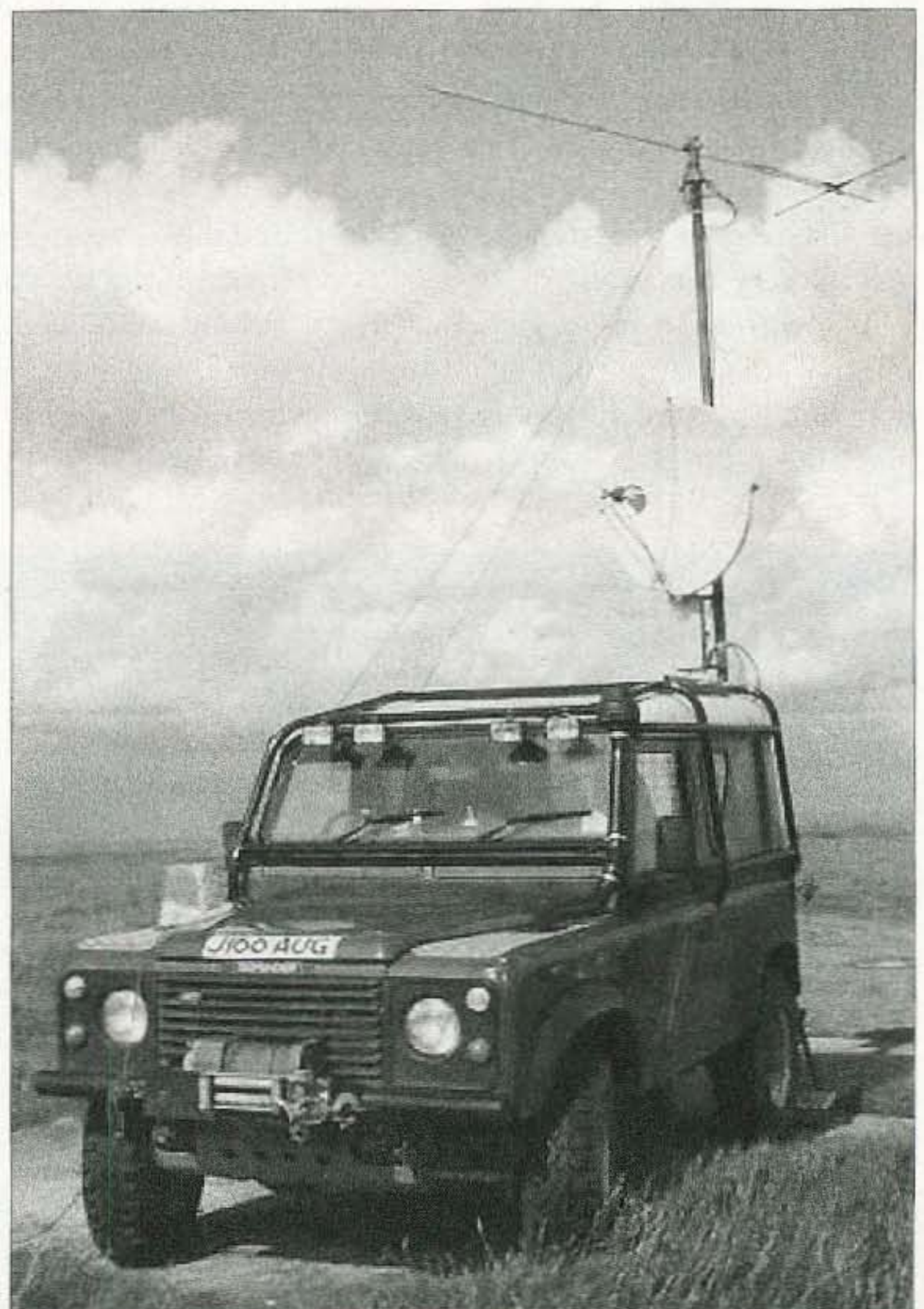
Photo A. Paul G6UAI's 144 MHz yagi and 10 GHz 1.2m Landrover dish array.
