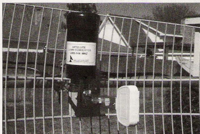
Photo B. Close-up view of the Parabolic downconverter on the small center antenna.
