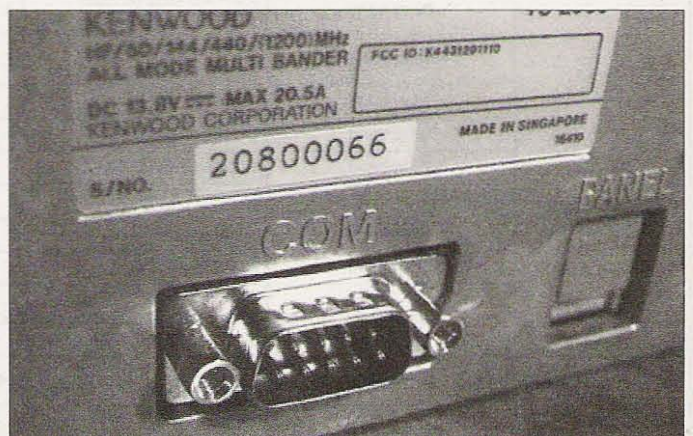
Photo E. The com port, which doubles as the rig control and TNC interface, is a DB-9. The "panel" port to the right is the interface for the RC-2000 remote head.
