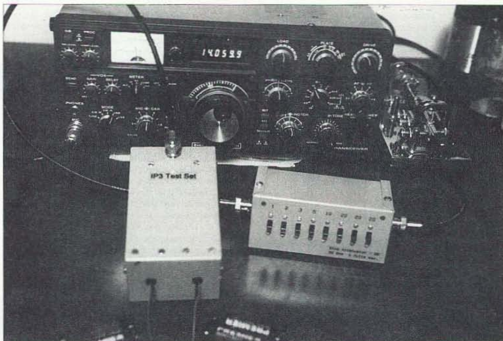
Photo A. Measuring intercept performance of a receiver.
