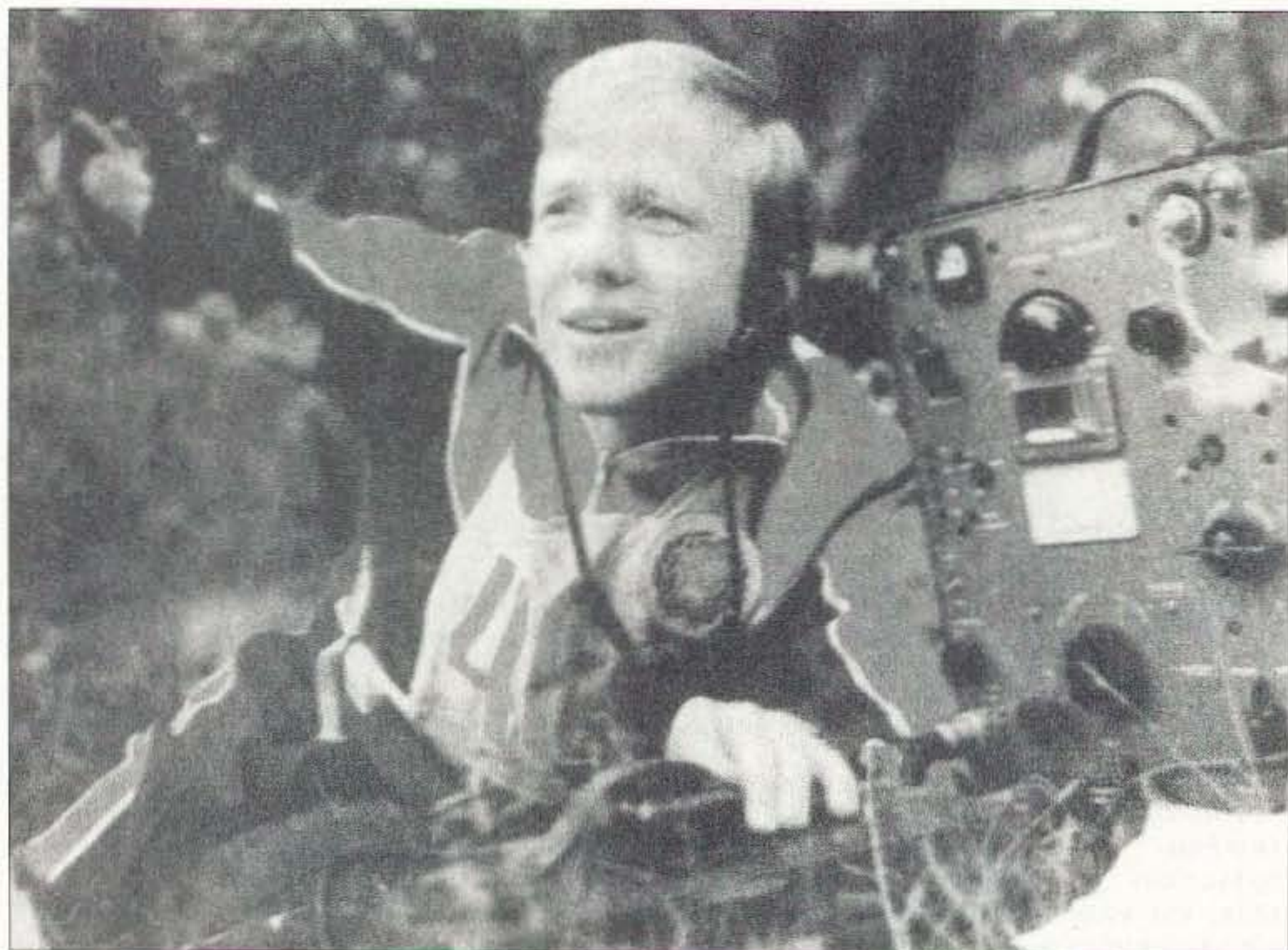
Photo A. In the early days of ARDF in Europe, fox transmitters were just like the ones used in USA T-hunts of the 1950s — big, bulky, and keyed by hand.
