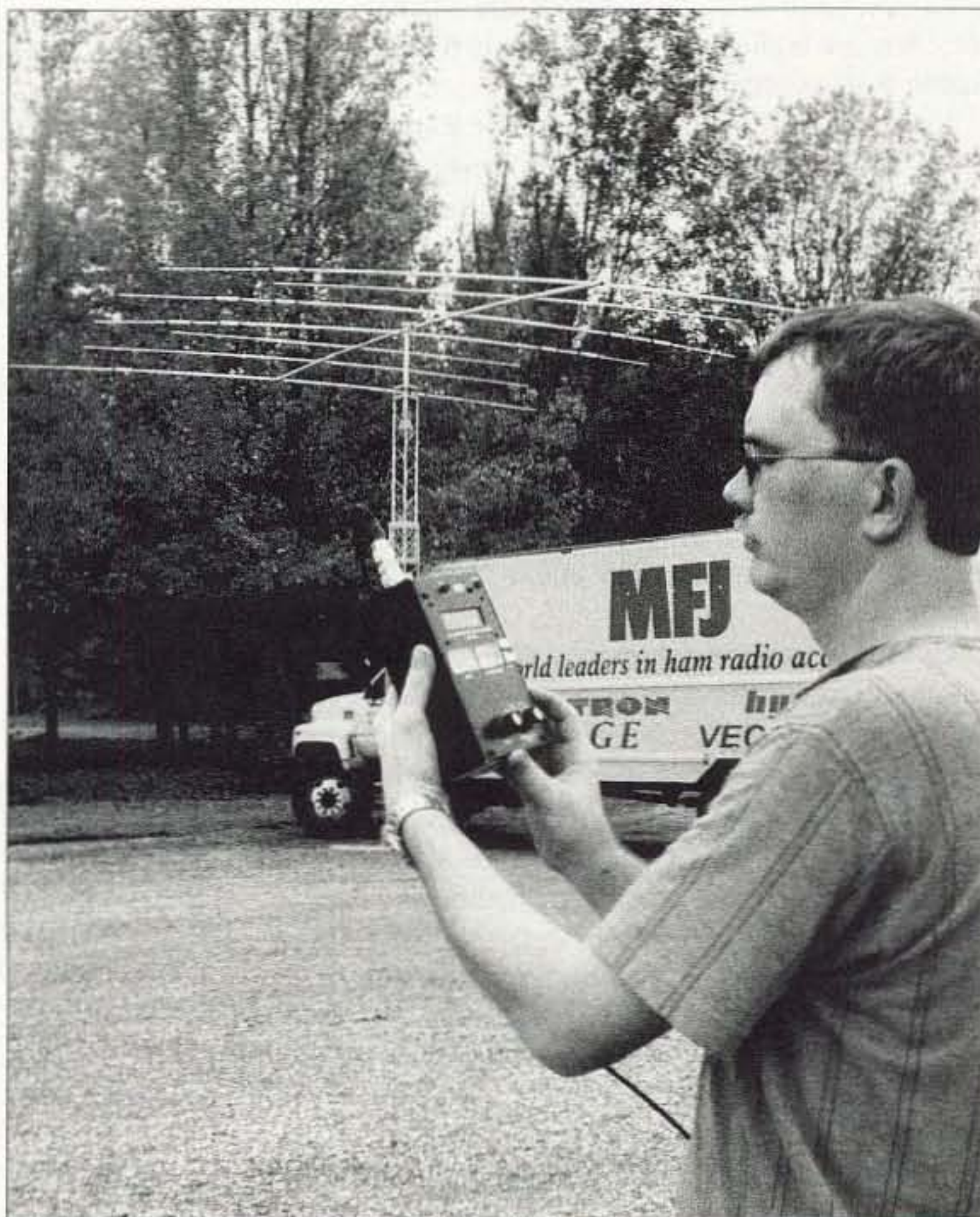
Photo B. Randy Nash KC5NIS, Hy-Gain's antenna production specialist, tunes and tests a new Mississippi-made TH-7DX Hy-Gain antenna with an MFJ-269 SWR Analyzer.
