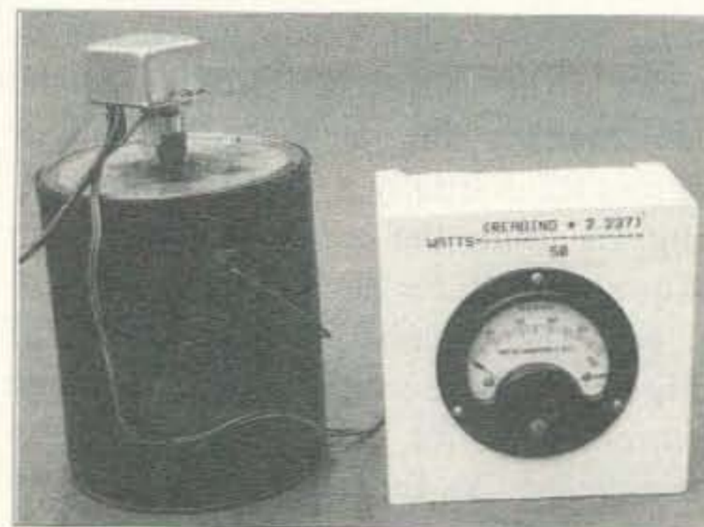
Photo C. The meter can be placed at a convenient distance from the rectifier circuit. The legend on the meter box which reads "WATTS = (READING x 2.237) 2 /50," results in the following correlations: 10 \mu A = 10 W; 20 \mu A = 40 W; 40 \mu A = 160 W; 80 \mu A = 640 W; and full scale = 100 \mu A = 1000 W. RMS voltage equals 2.237 multiplied by the reading. The box covering the rectifier assembly is a Mouser #537-MO18-PLTD.
