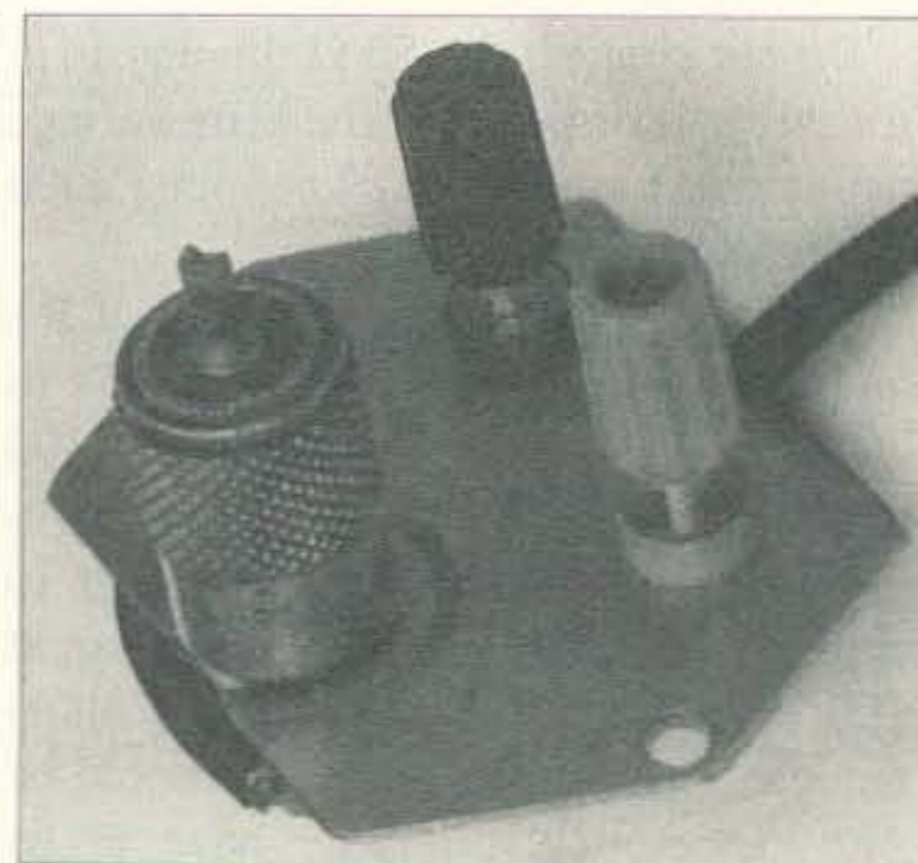
Photo B. A PL-259 connector and two binding posts allow convenient connections to the load and meter leads.
