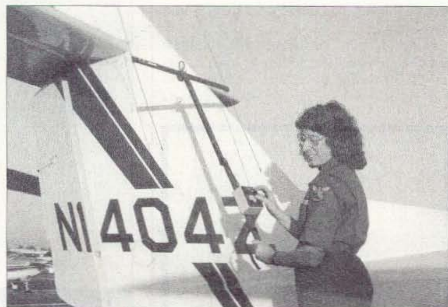
Photo C. The L-Per dual-antenna and receiver set by L-Tronics is designed for on-foot tracking of aircraft emergency beacons as well as hidden ham transmitters. Cathy Livoni KD6CYG is using this one at the Fullerton Airport.
