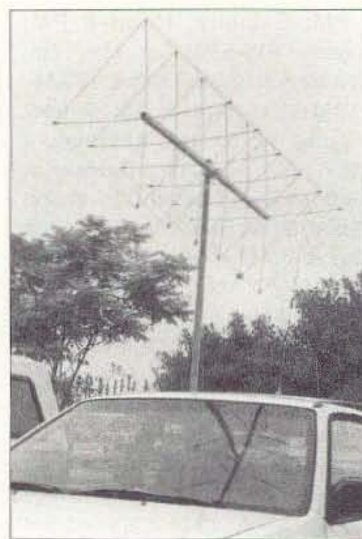
Photo B. Bandmaster quads for two meters are available with two, four or six elements. Note the SO-239 coax connector at the lower corner of the driven element.
