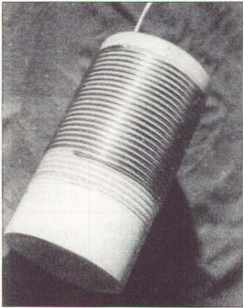
Photo A. The six-inch length of PVC piping, threaded at 6 tpi, with the coil temporarily wound on the form.
