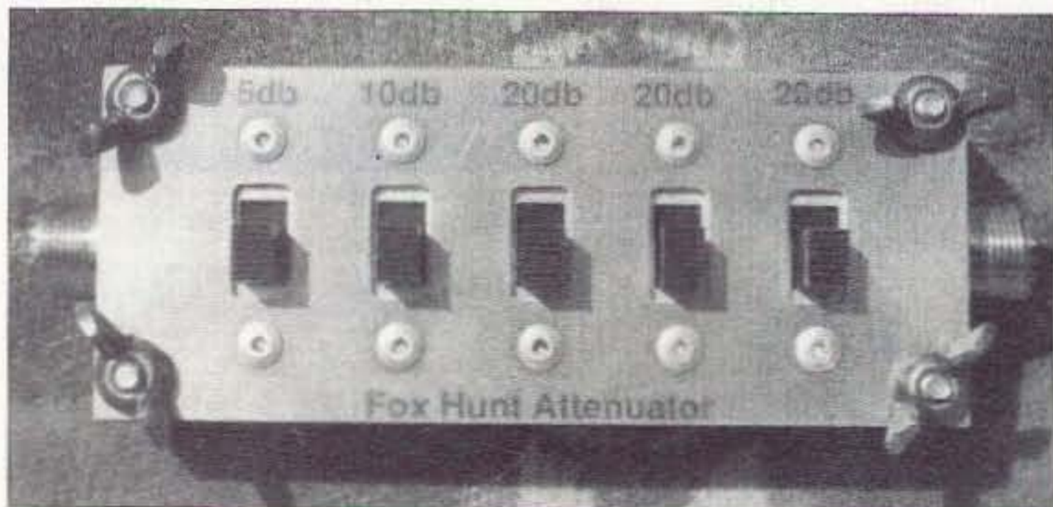
Photo A. You will need an RF attenuator for closing in on the transmitter with your beam or quad. This resistive unit was made by Arrow Antenna.
