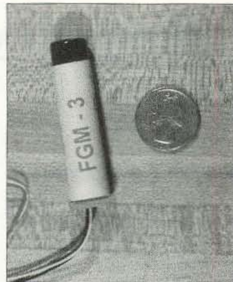
Photo A. The Speake FGM-3 magnetic field sensor.
