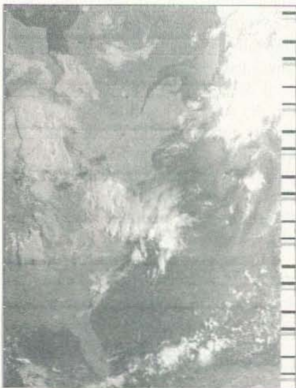
Photo B. A sunny day in New Hampshire. This infrared image stretches from the tip of Florida all the way north to the bottom of Hudson Bay. The bars on the right border are the synchronization signals that are transmitted at the beginning of each line.
