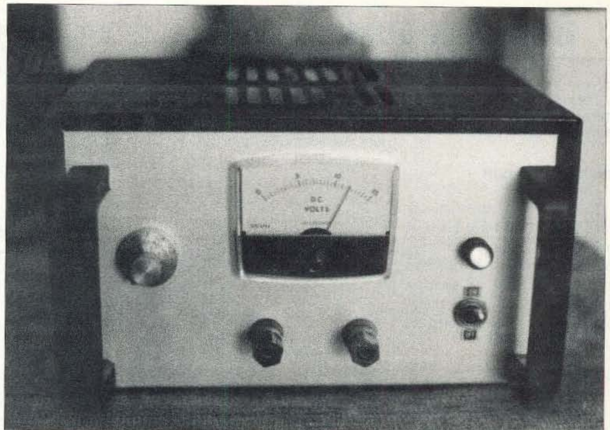
Photo A. K8KWD's variable-voltage utility power supply.
