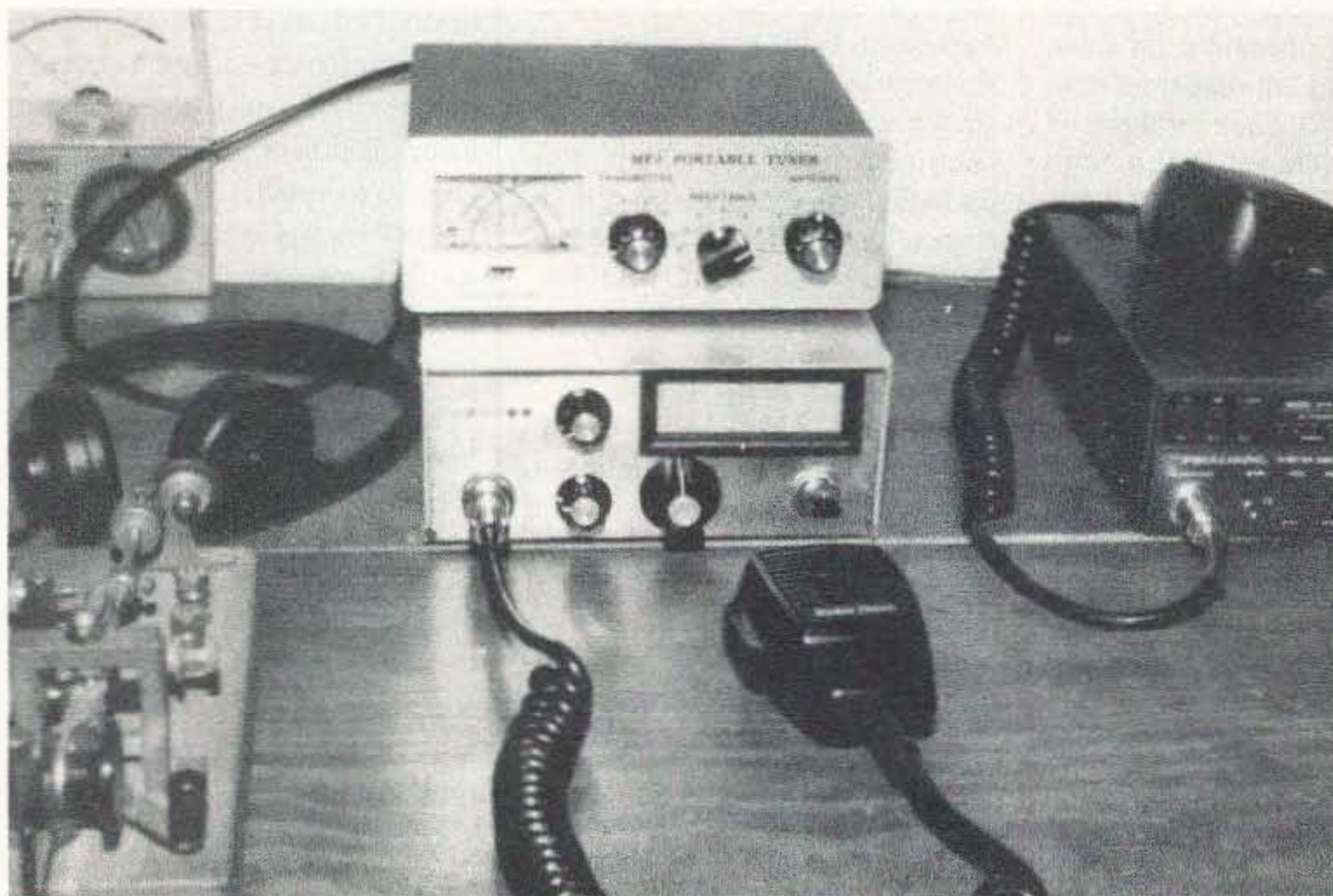
Photo A. The author's QRP station. In the center of the photo is a home-brew 5 watt SSB transceiver that operates on the 17 meter band.
