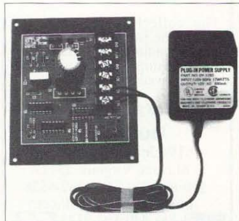
Photo A. The completed power supply unit. (Photo by John Jacobs, Independence WV 26374.)
