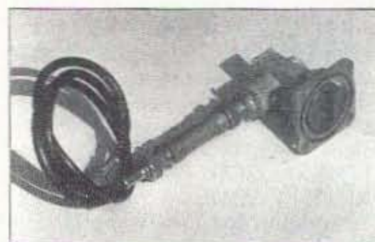
Photo A. A signal marker for 10 GHz use driven by a 2 meter HT. It produces a calibrated harmonic in the 10 GHz band for calibration purposes.
