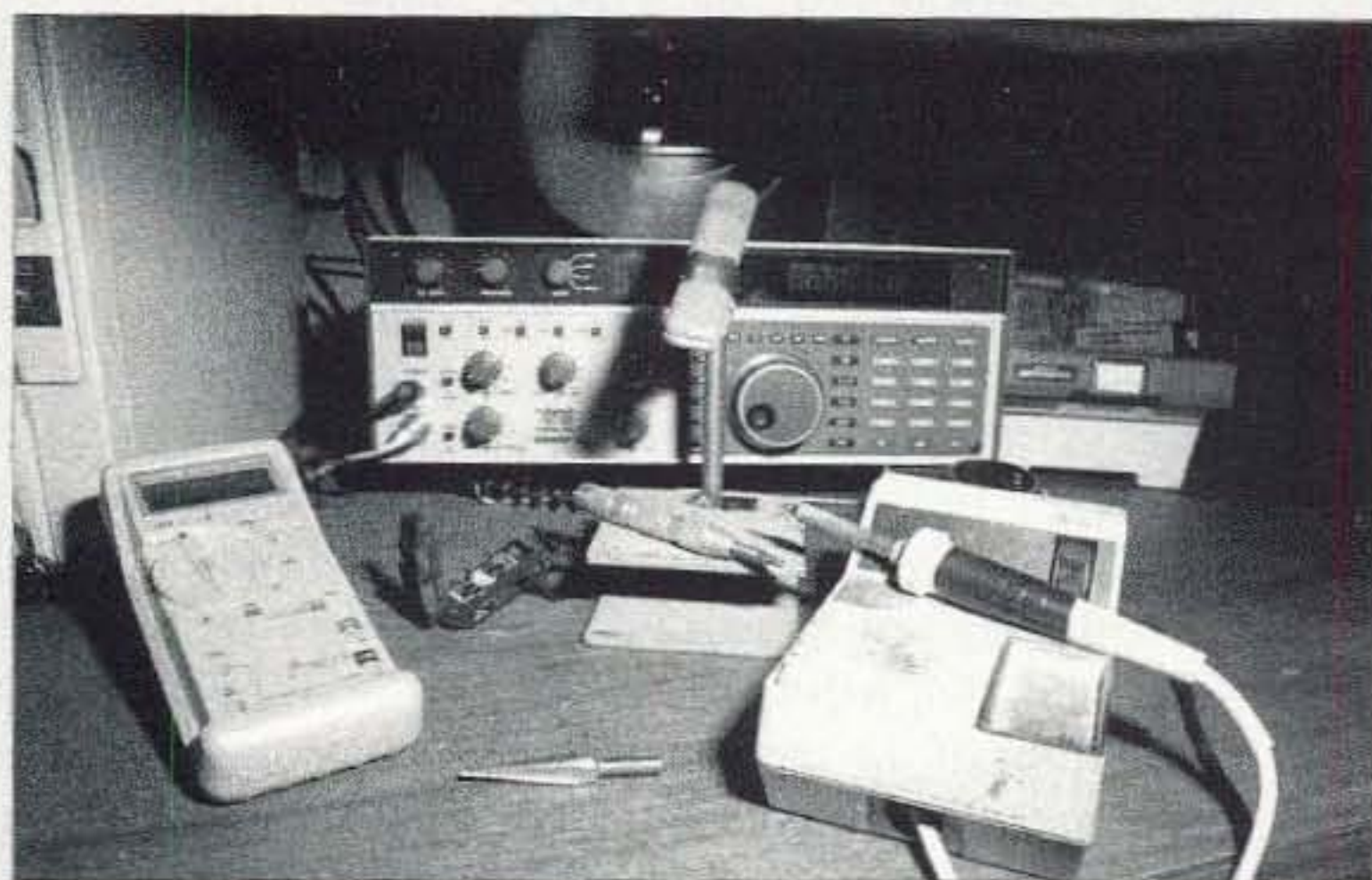
Photo D. The workbench, with a meter, soldering iron, center punch, an equipment clamp, and bits.
