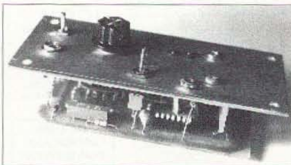
Photo E. The board mounted on the front panel, ready for paint and labeling.
