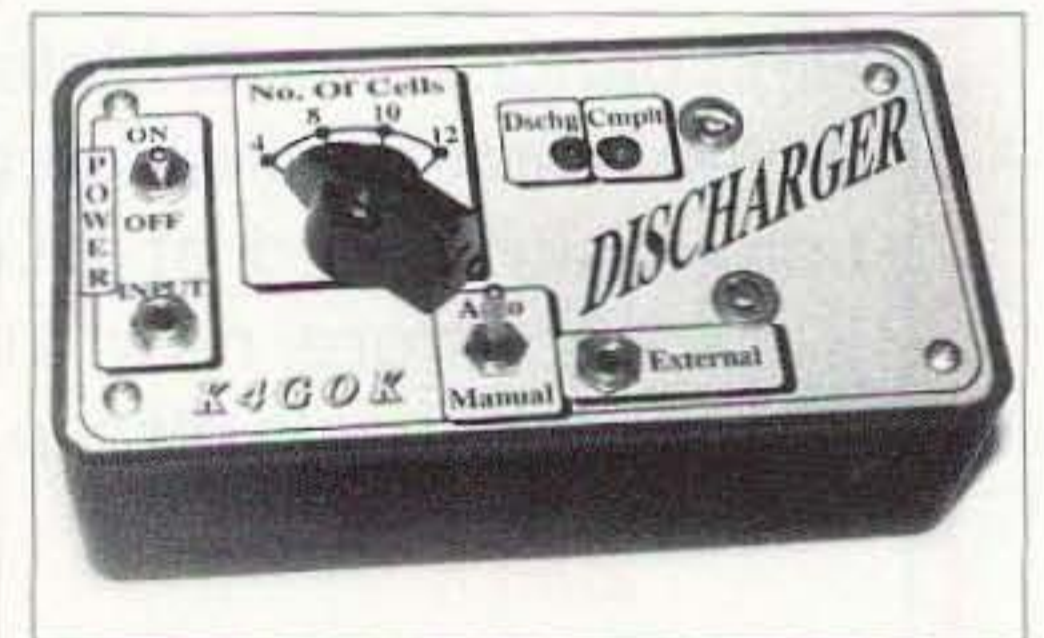
Photo A. The completed discharger (prototype unit).
