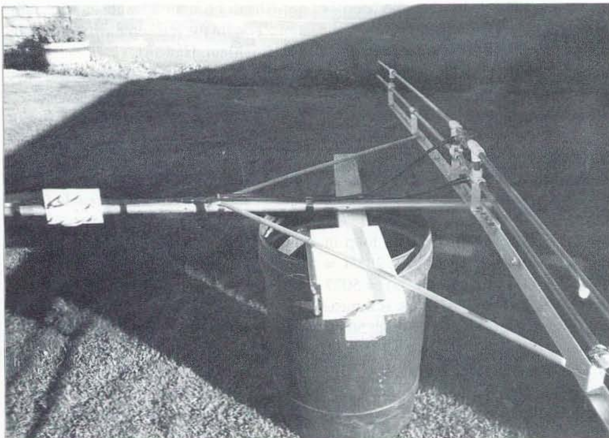
Photo B. To drill the bolt holes for mounting, flatten 1" of the ends of your 1/2" tubing, creating a support angle stabilizing wishbone.
