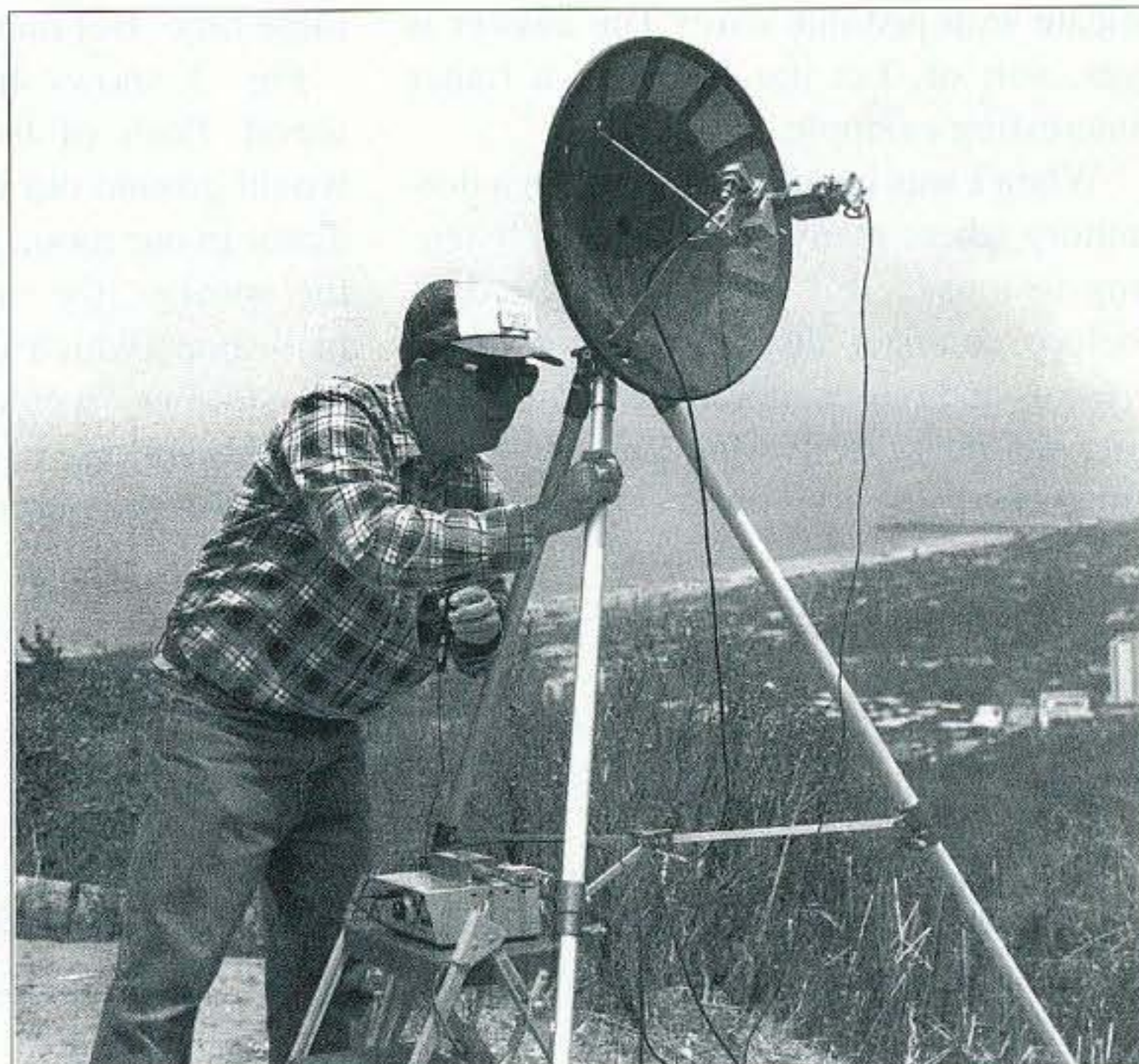
Photo A. Ed Munn W6OJY operates an early WBFM full-duplex transceiver used to win the first ARRL 10GHz contest. The San Diego Microwave Group helps keep us at the cutting edge of this kind of technology.
