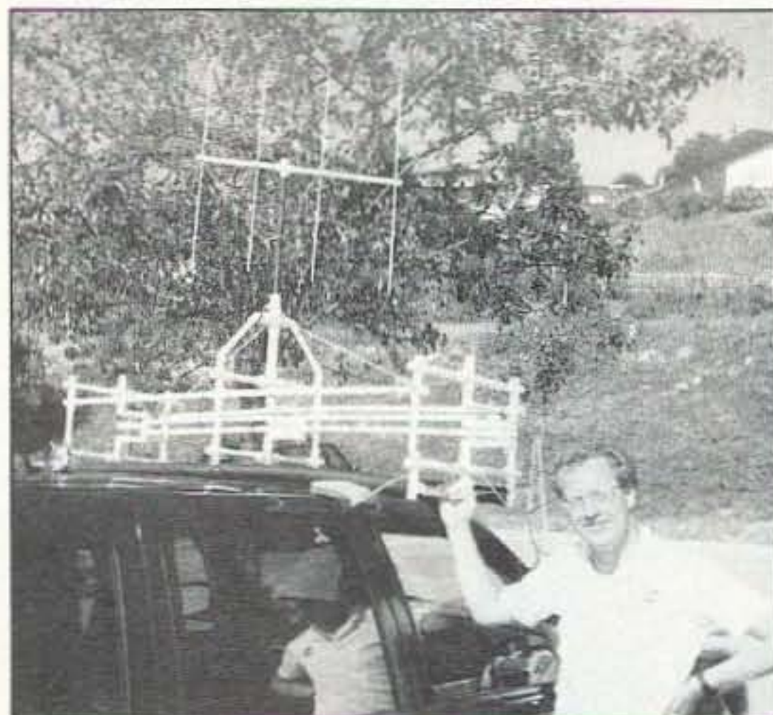
Photo D. James Swenson KC6YSV figured out a clever way to mount his yagi atop the car roof without drilling a big hole. Handles at each end of the PVC pipe framework allow both driver and passenger to rotate the yagi.
