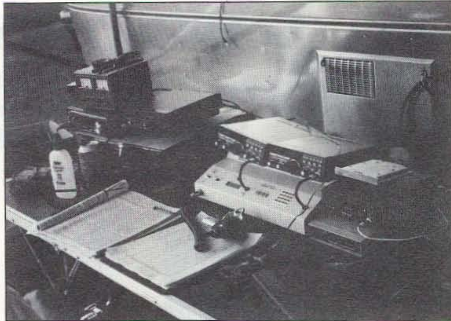
Photo C. The hamsat station at N5EM was ready for everything from Mode "K" through Mode "S," including 9600-baud digital activity.
