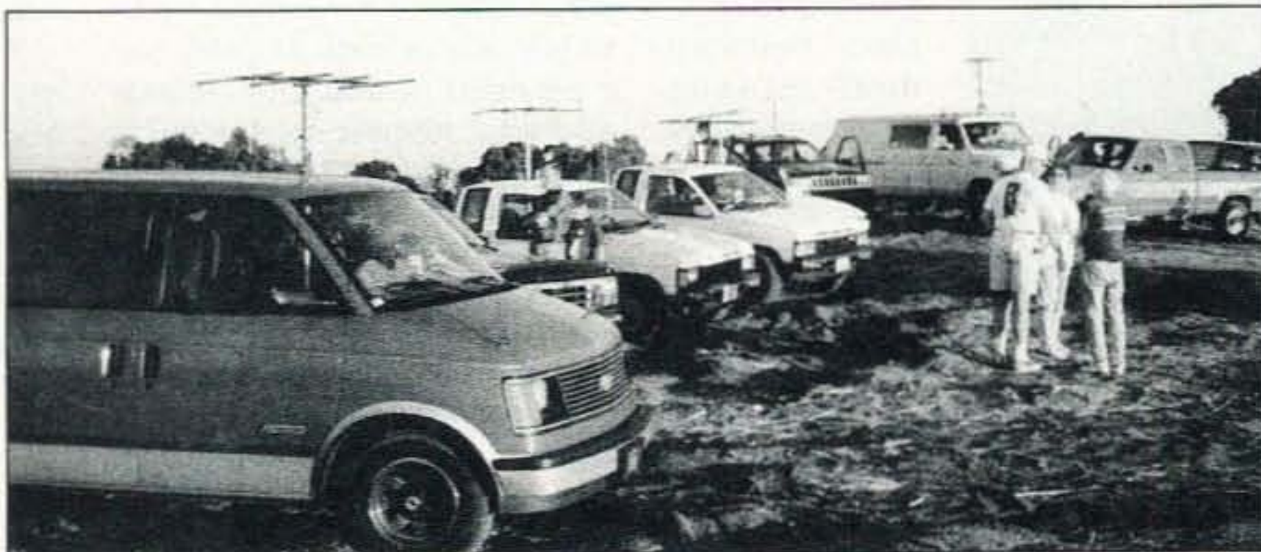
Photo A. At sunset on a summer Saturday, southern California T-hunters gather on a hilltop to have their odometers read before the hidden transmitter comes on the air. Most have yagis or quads on rotatable masts extending through their vehicle roofs.
