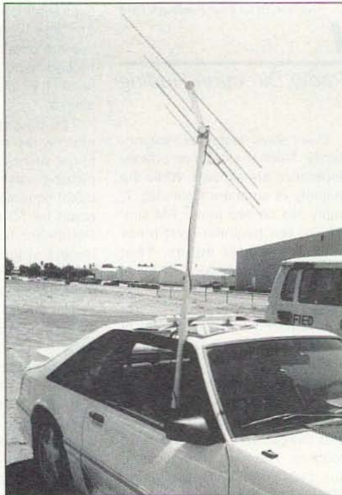
Photo C. With a little thought, you can come up with a simple no-holes way to mount a rotating beam through the passenger window of almost any car. Put some sort of thrust bearing in the armrest at mast bottom for easy turning at highway speeds. Mount the beam so that a twist of the boom changes polarization.
