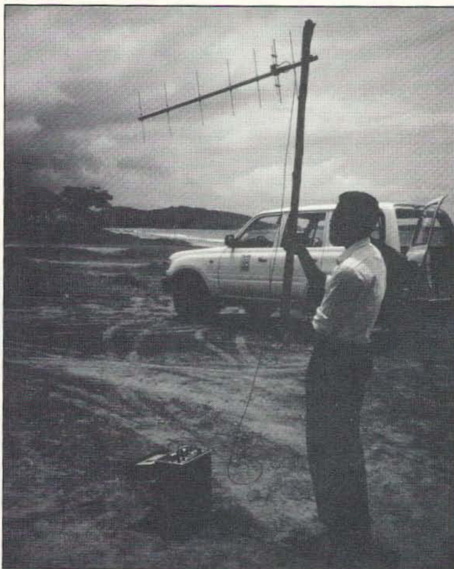
Photo B. Using a spectrum analyzer, attenuator and yagi, KD6KQ and helper Desmond Cole ended up at the beach, with the signal still appearing to come from the airport across the bay.
