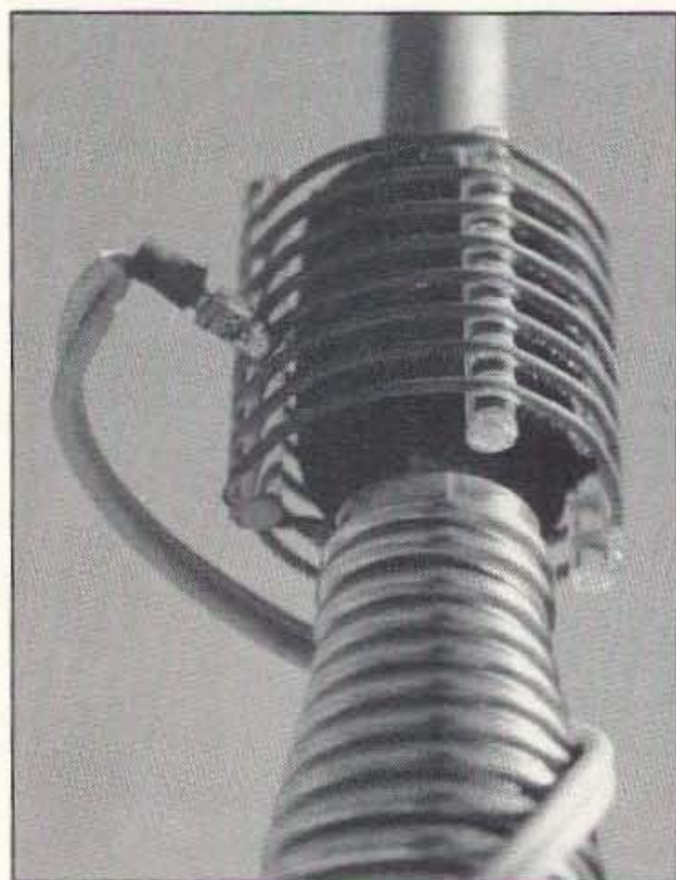
Photo D. It may take a coil to resonate the 75m and 40m whips on some vehicles.
