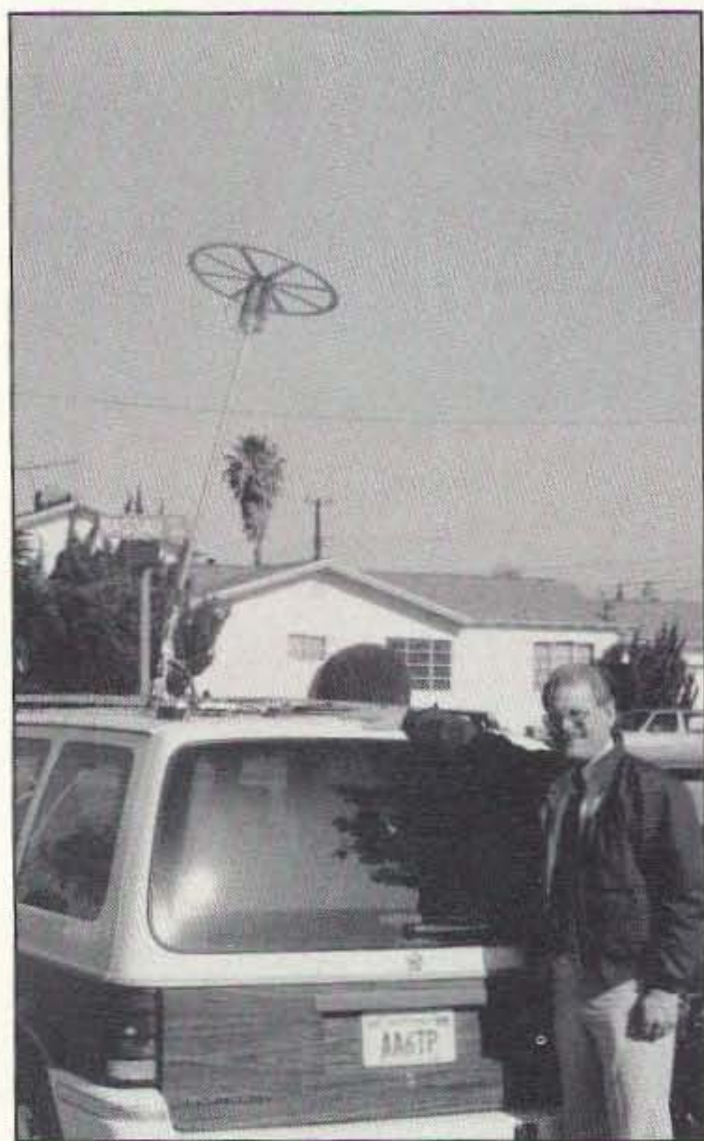
Photo B. A capacity top hat extends the resonant points on a 40 meter antenna, so no tuner is needed!
