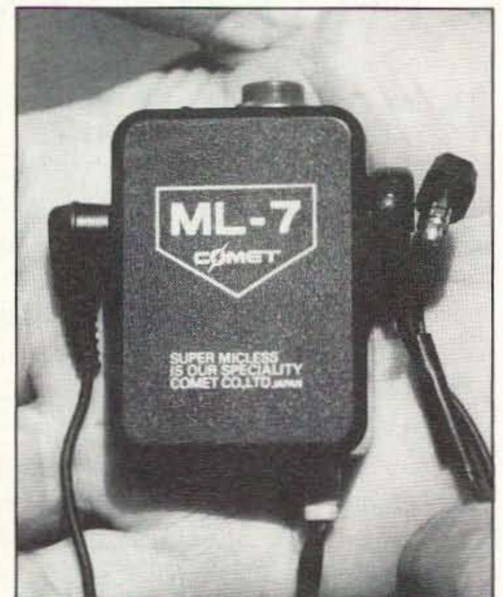
Photo B. The ML-7 miniature speaker/mike accessory from Comet allows you to easily adapt your HT for motorcycle mobile use.
