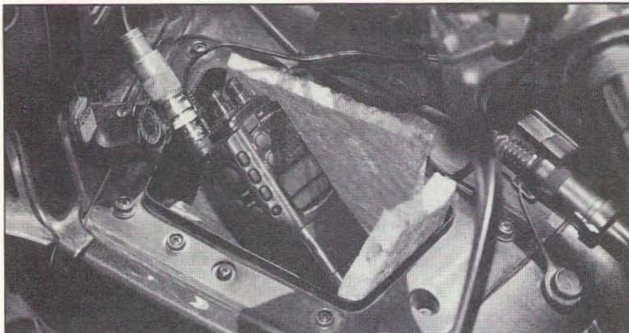
Photo C. This simple handheld installation can be easily removed to prevent theft.
