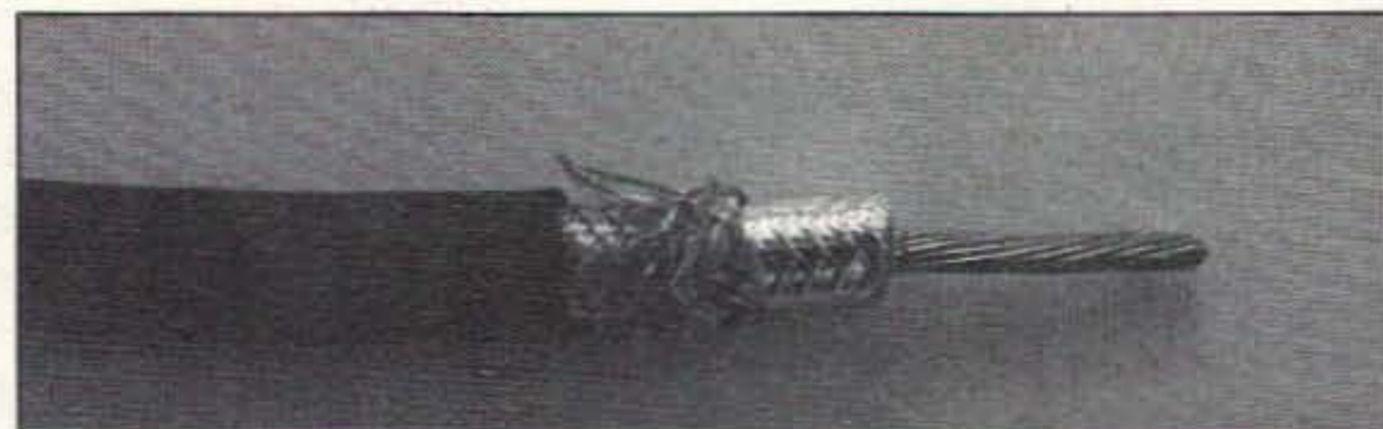
Photo B. A piece of 9096 with an end stripped and the tinned copper braid pulled back to reveal the aluminum-mylar film shield. You would not normally do this to install connectors. That #9 stranded center conductor is a healthy bunch of copper.
