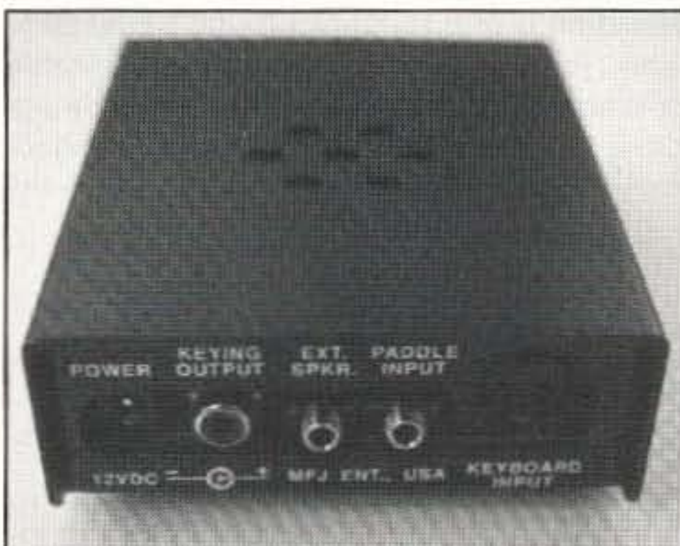
Photo B. The rear panel of the MFJ-451 keyer box contains I/O ports for: 12 VDC in; keying output; external speaker; paddle input; and keyboard input.
