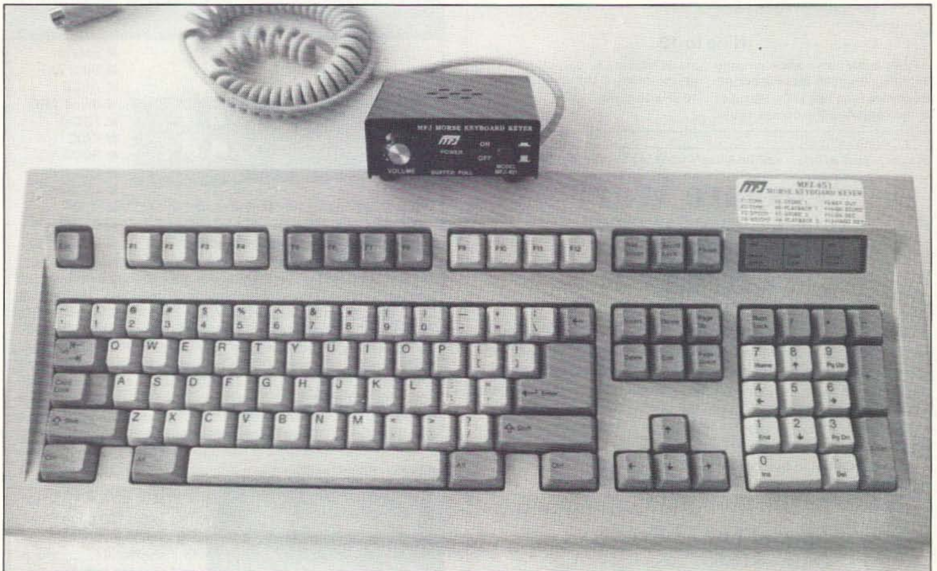
Photo A. The MFJ-451 Morse Keyboard Keyer is primarily a keyboard, as you can see. The keyer electronics is all inside the tiny black box. The front panel contains only a volume control, status indicator LED, and sidetone volume control.
