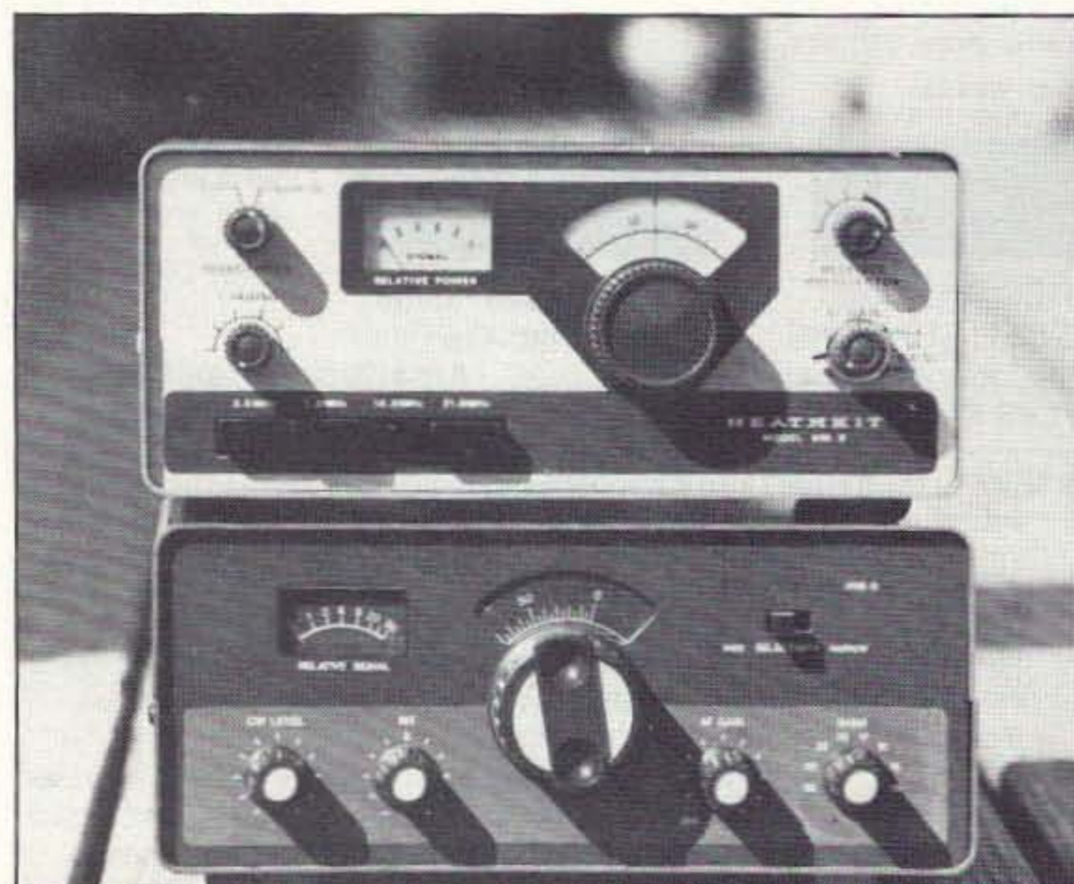
Photo D. The popular Heathkit HW-8 and HW-9 CW-only QRP transceivers. These are great fun!
