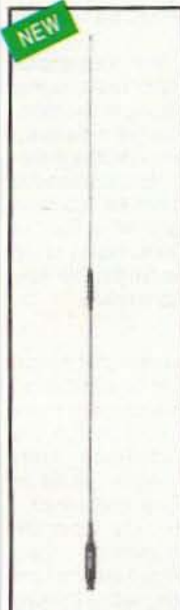
NEW CH-722SA 146/446MHz HT Antenna Gain & Wave: 146MHz 3.0dBi 1/2 wave 446MHz 5.5dBi 5/8 wave x 2 Max Power: 50 watts Length: 36" Weight: 3.9 ozs. Connector: BNC
