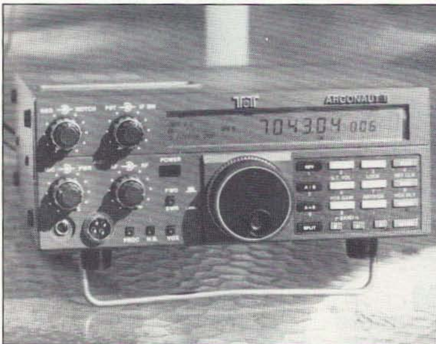
Photo A. The Ten-Tec Argonaut II is a full-featured QRP transceiver.
