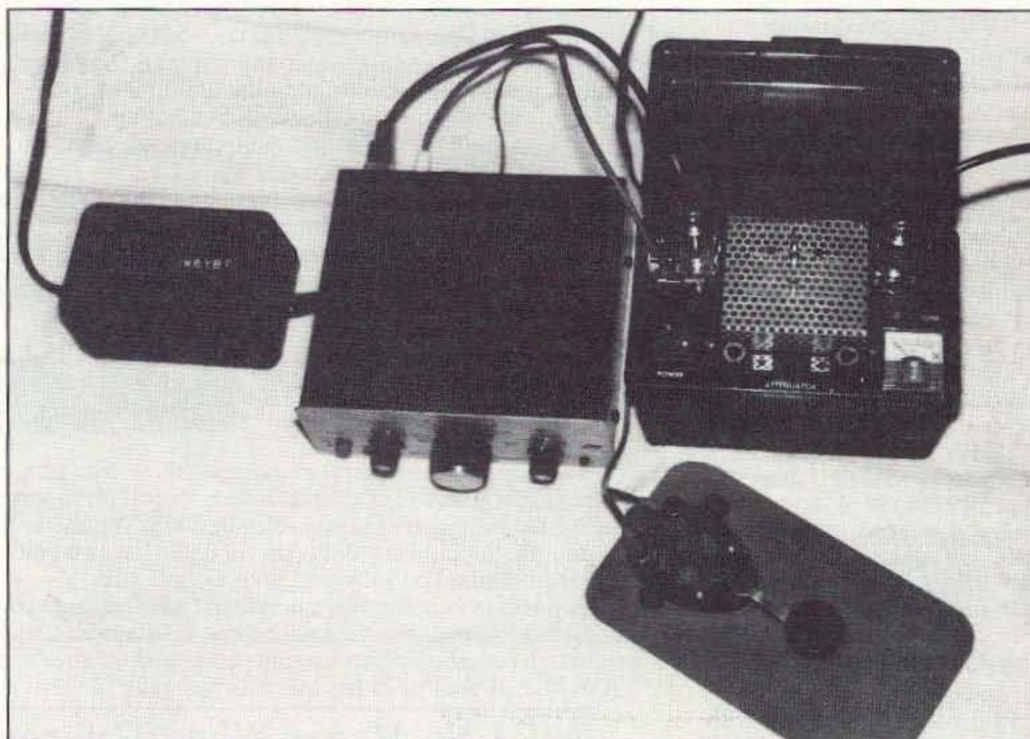
Photo C. Ready to go. The portable station was completed by the addition of a two-pound power supply (left) and a two-pound RF amplifier. Note the old reliable J-37 key mounted on a piece of circuit board.
