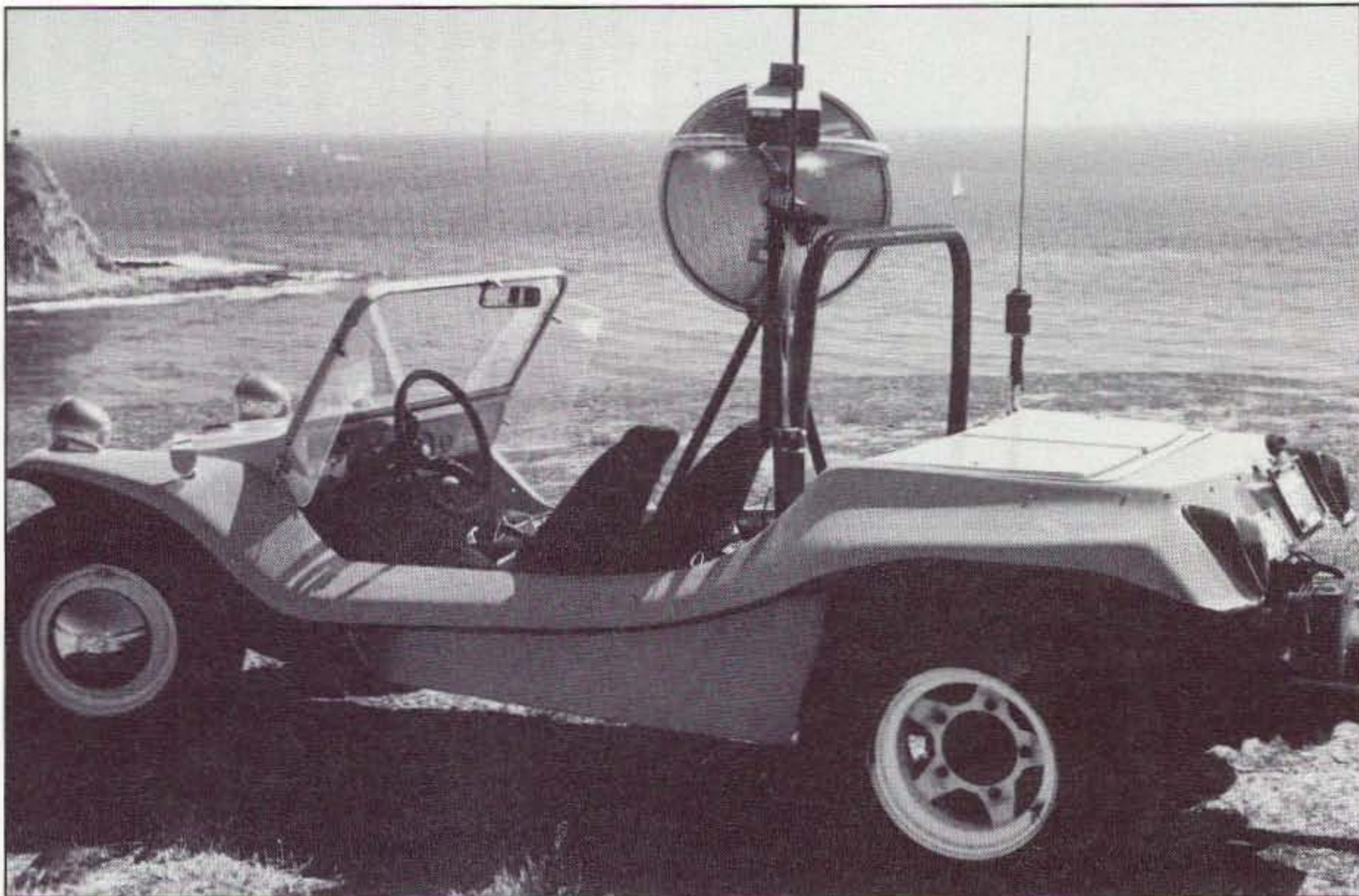
Photo A. The ARR 10 GHz FM system makes an ideal mobile microwave station.
