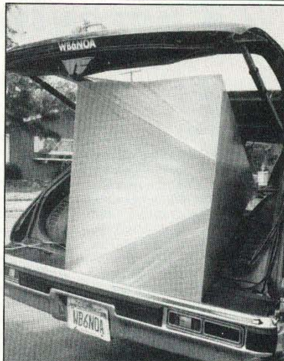
Photo H. Side view of the Super Horn antenna. The two halves are joined at the top and bottom for maximum strength (i.e. each half has two bends in it).
