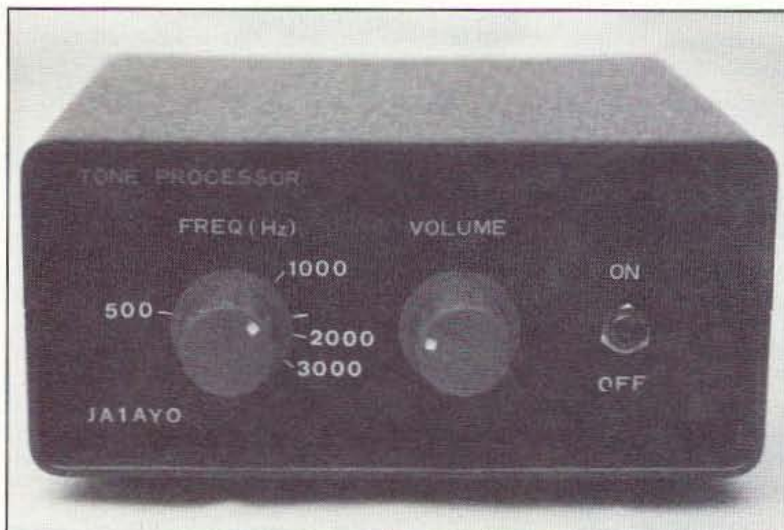
Photo A. Remove interference with this versatile switched capacitance audio filter.
