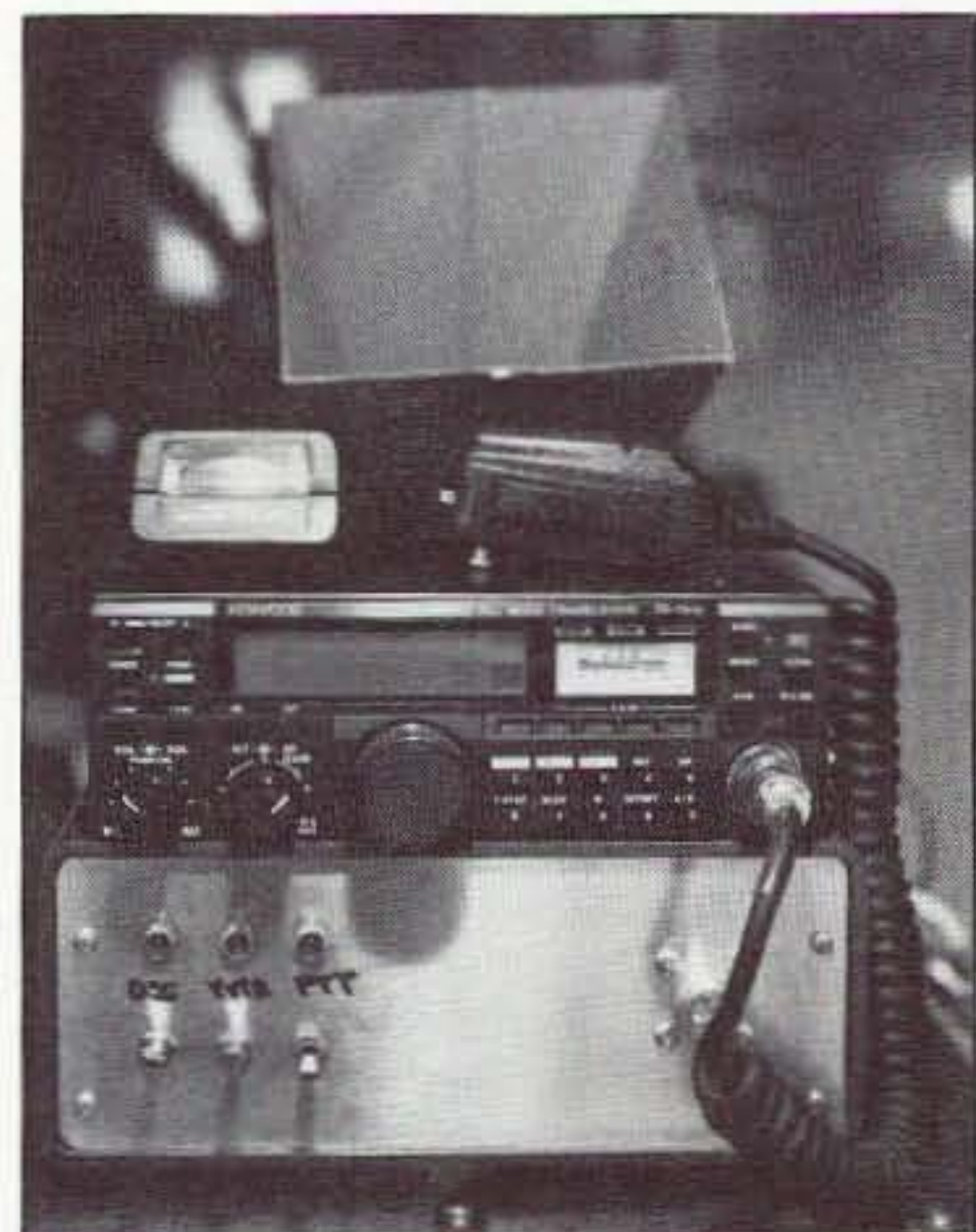
Photo B. A completely portable 10 GHz SSB station (200 mW output) can be easily assembled through the use of the SSB Electronic USA 10 GHz transverter, a 2m multimode rig and a horn (or dish) antenna.
