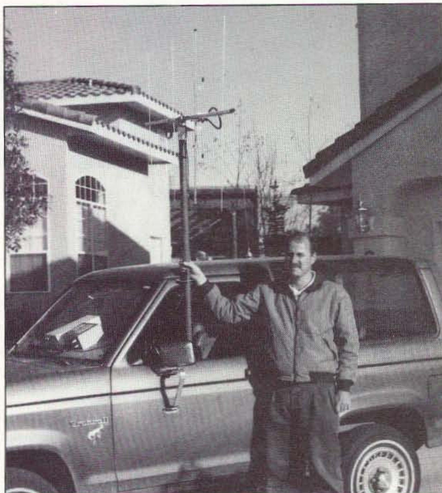
Photo A. Jerry Boyd WB8WFK is ready to go T-hunting with his yagi connected to a digital bearing display system. His analog display and interface box are on the dashboard.
