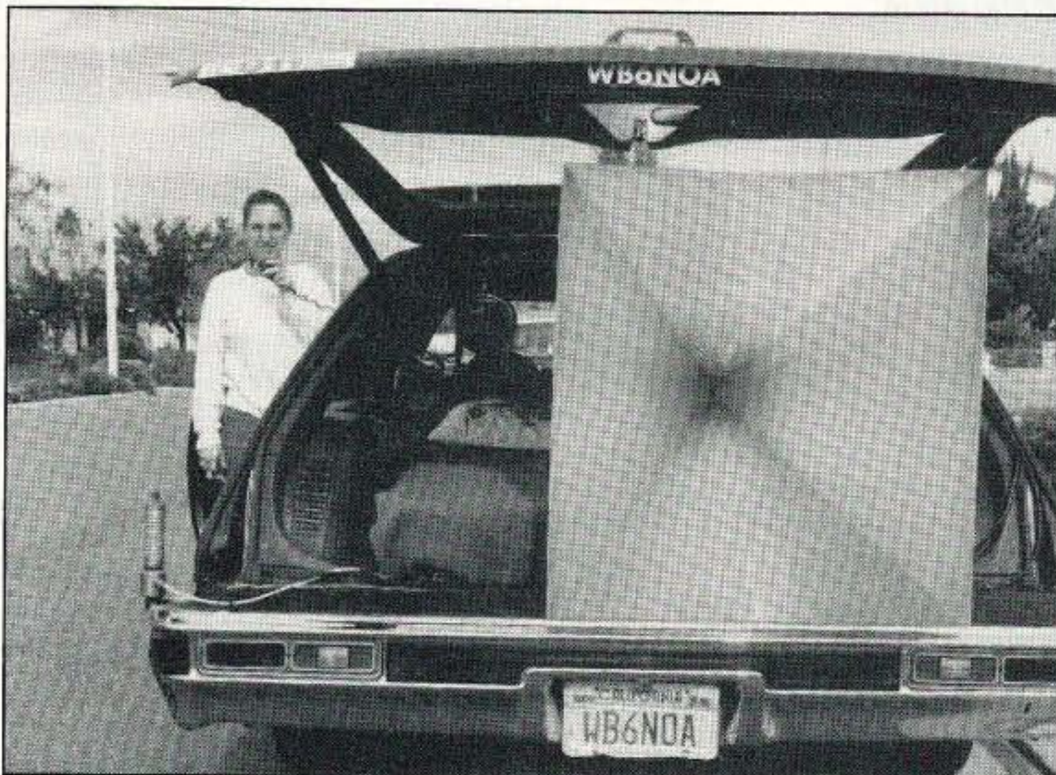
Photo G. No, this is not a rocket-assisted station wagon. Suzy N6GLF operates portable 10 GHz SSB using the Super Horn antenna.
