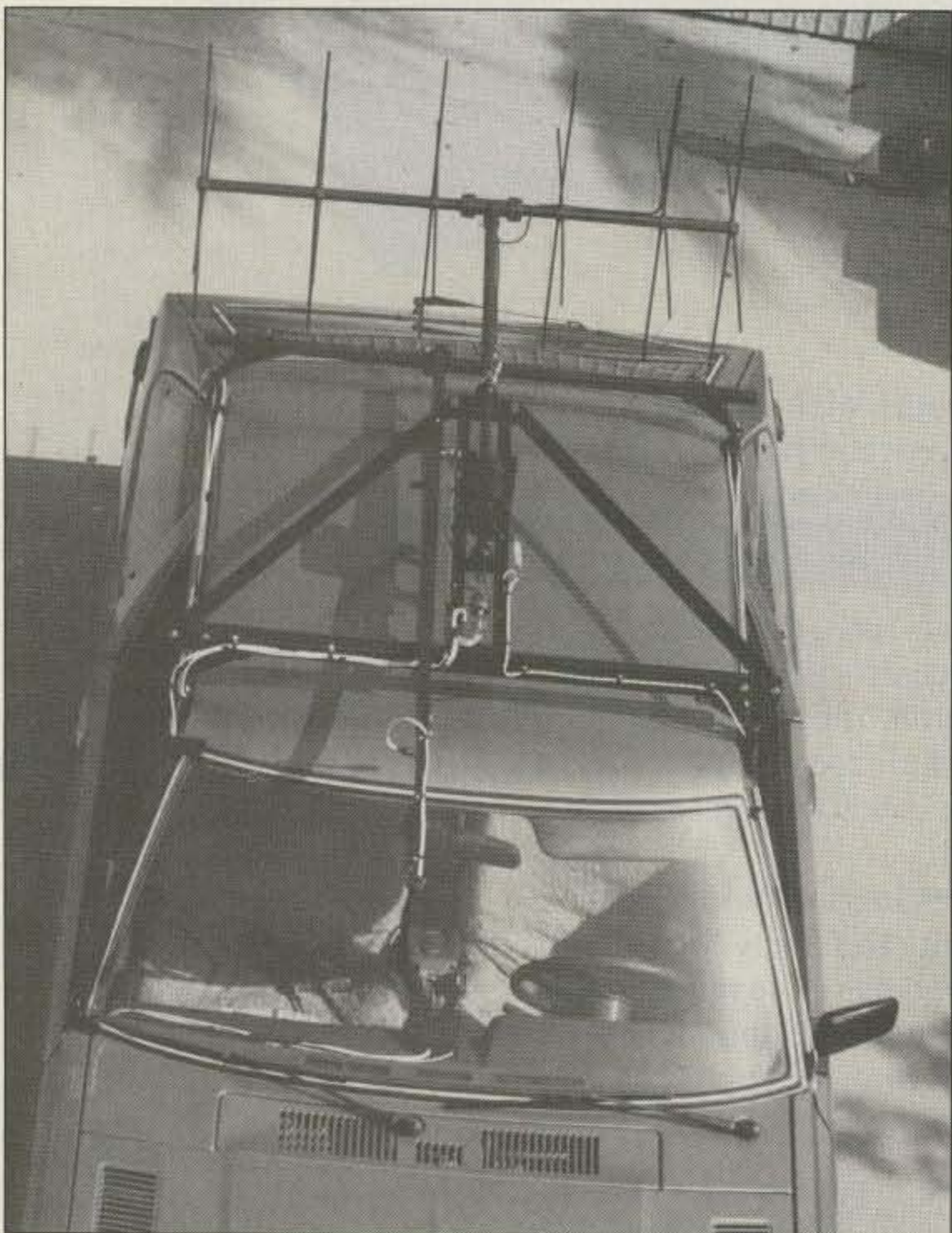
Photo C. JaMi can fold the entire antenna assembly down on the car top for low-clearance situations.
