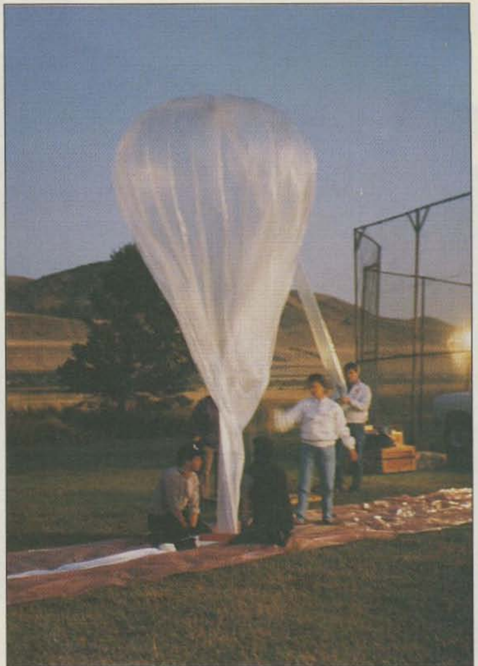
Photo A. Inflating the zero-pressure balloon for payload test flight #8. Photo by Gil Moore N7YTK.
