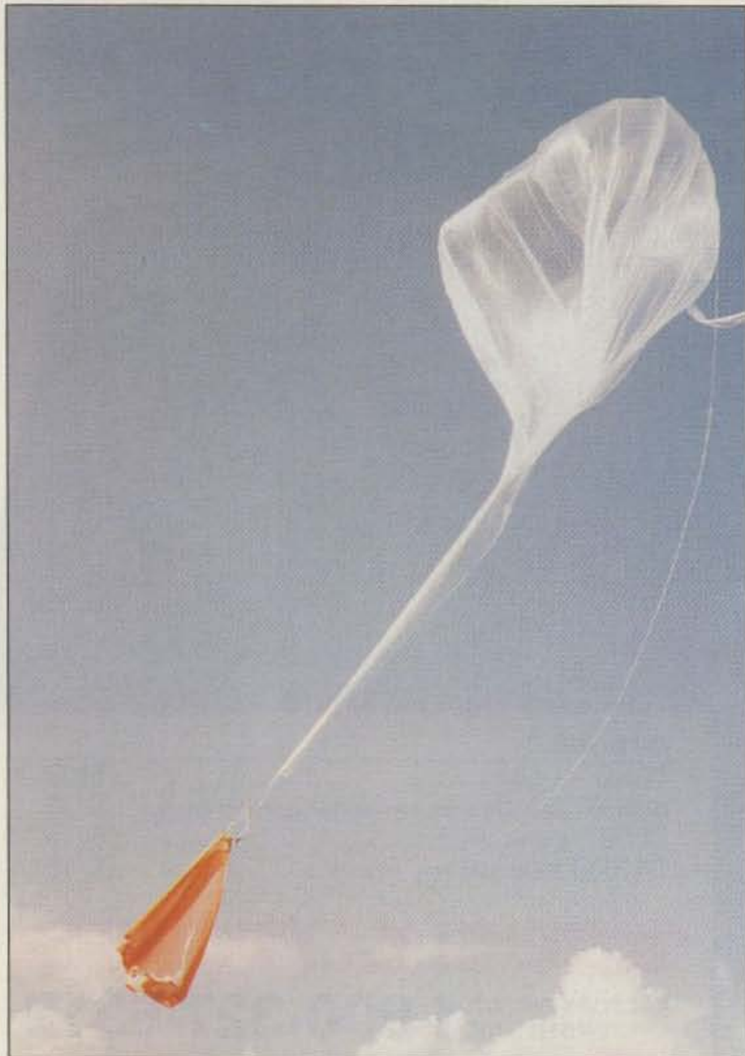
Photo B. Liftoff of flight #7 using a zero-pressure balloon. Photo by Harl Goodsell W7LTH.
