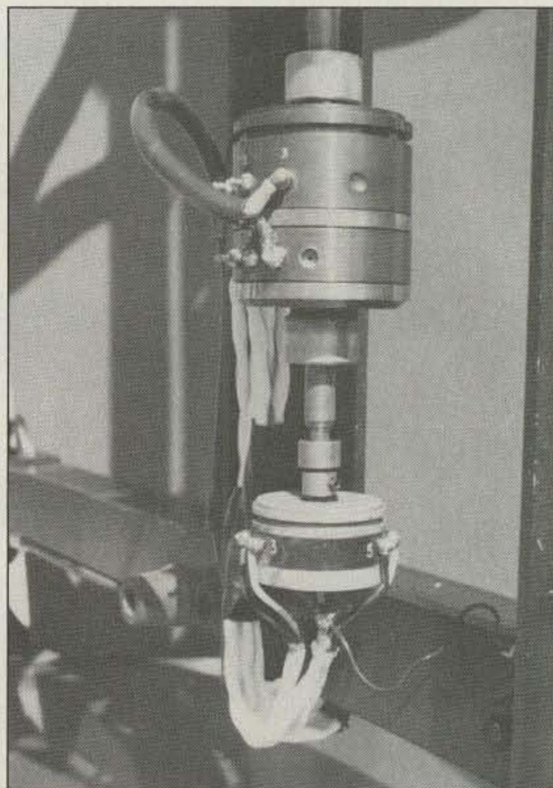
Photo D. Close-up of the two-stage pot modified into a coax rotary coupler (above) and the special sine-cosine pot (below) on the mast bottom.
