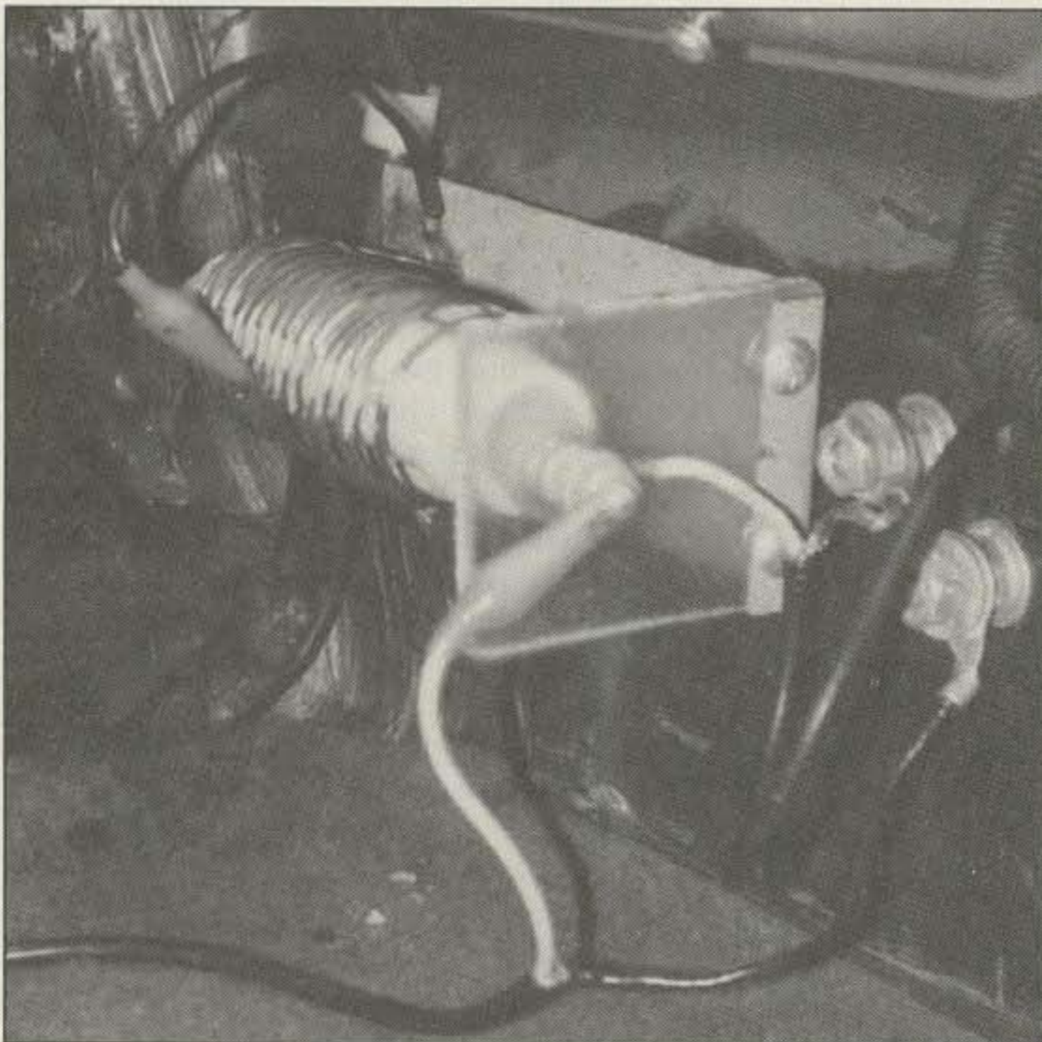
Photo D. The matching coil assembly mounts inside of the vehicle. Grounding and feedline alligator clips allow for fine tuning of the resonance and impedance of the antenna.
