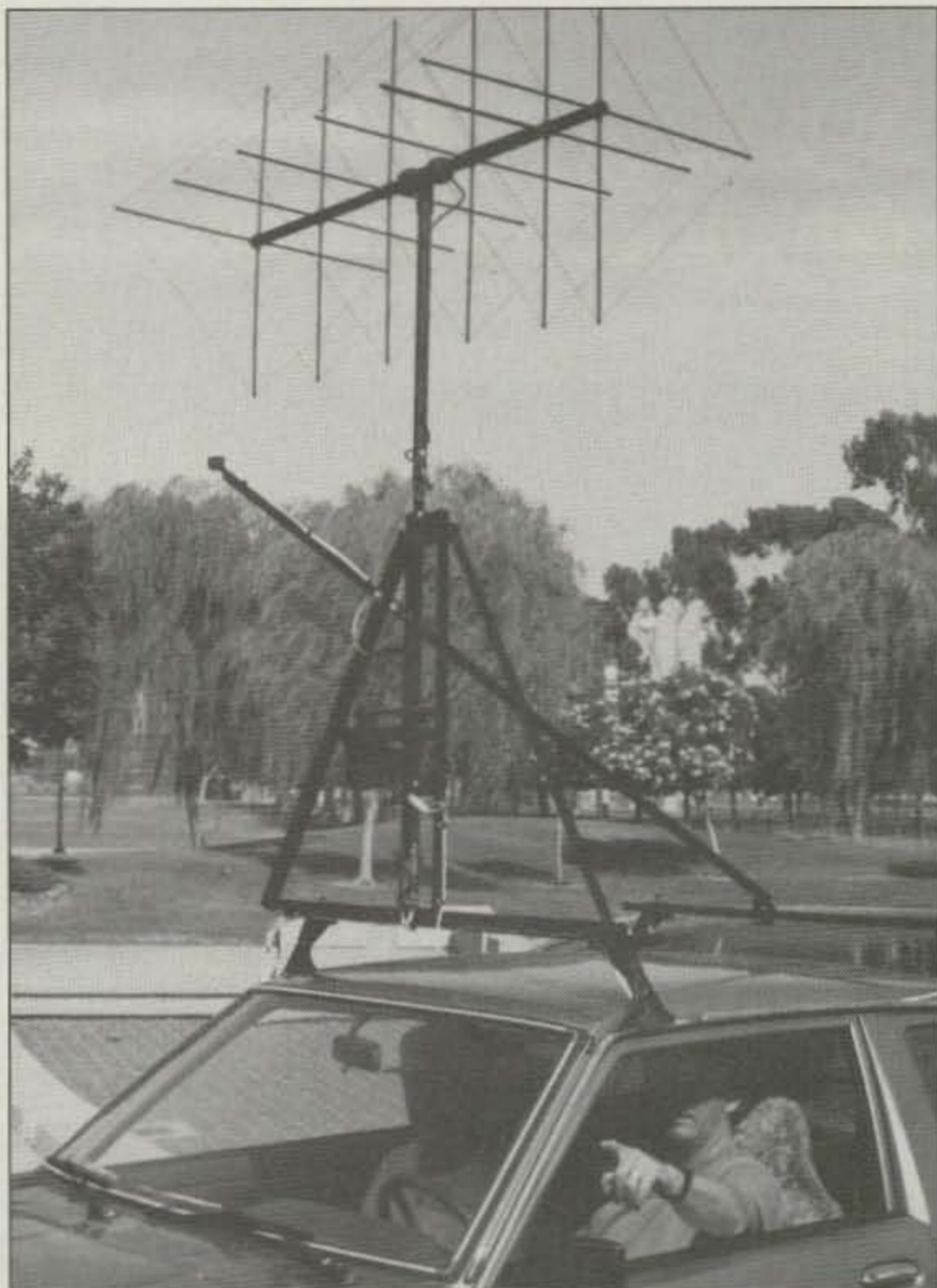
Photo A. Heads turn when JaMi Smith KK6CU goes on foxhunts with this array. It spins at 40 RPM and displays bearings on a storage oscilloscope.
