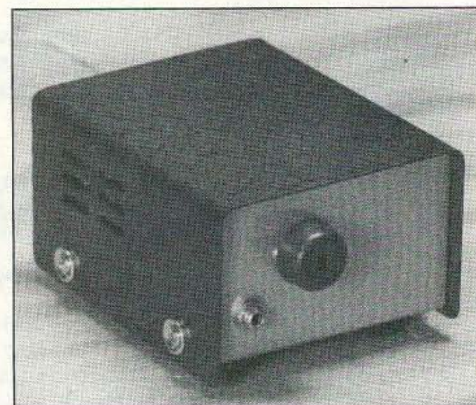
Photo A. This well-dressed Rock Bender sports a black-and-gray cabinet from Mouser Electronics (part number 4OUB101). The key jack is near the lower left corner of the front panel. The tuning knob is a black rubber cabinet foot.
