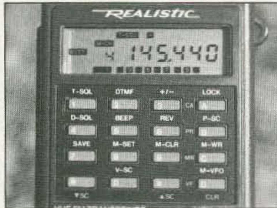
Photo B. The LCD screen is easy-to-read in daylight, but too poorly back-lit for nighttime viewing. The big keyboard makes it easy to push the buttons.
