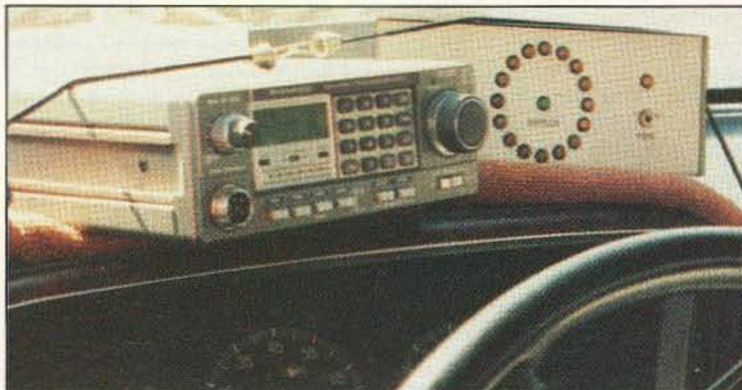
Photo A. Doppler RDF sets are "standard equipment" on Phoenix area hunts. Bob and Jackie Neve (WB7SMU and WB7SMT) strap their home-brew readout to the top of the dashboard.
