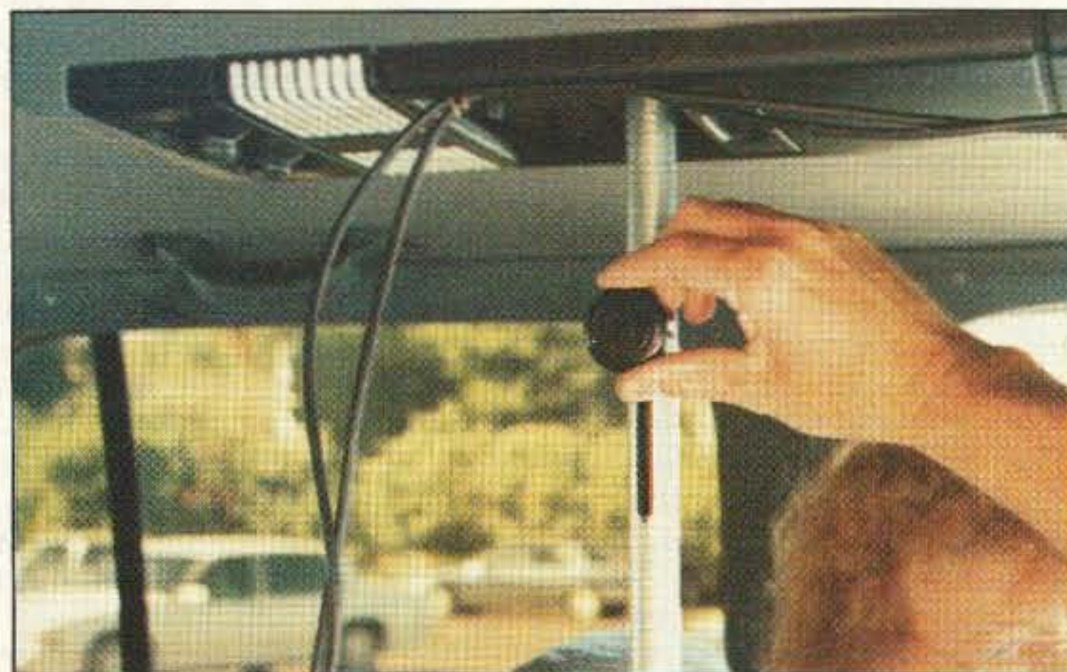
Photo C. It's easy for Bill and Boni Pineups (KC7VV and WT7Z) to change polarization on their yagi from inside by sliding this lever on the mast up and down. These clever hunters have a Doppler on board, too.
