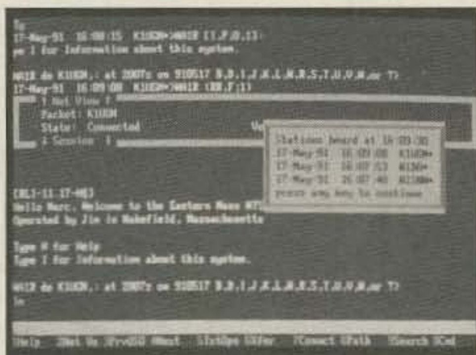
Photo A. While you're connected to another station, Pkt-GOLD's versatile features allow you to monitor all of the channel activity. All activity is displayed at the top of the screen (Net View); your connect session is displayed at the bottom portion (Session). Pop-up screens are available at any time. For example, pressing <ALT> F2 gives you the current MHEARD list.
