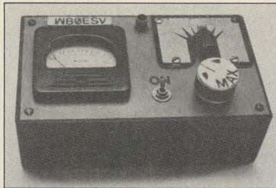
Photo A. The UHF field strength meter.
