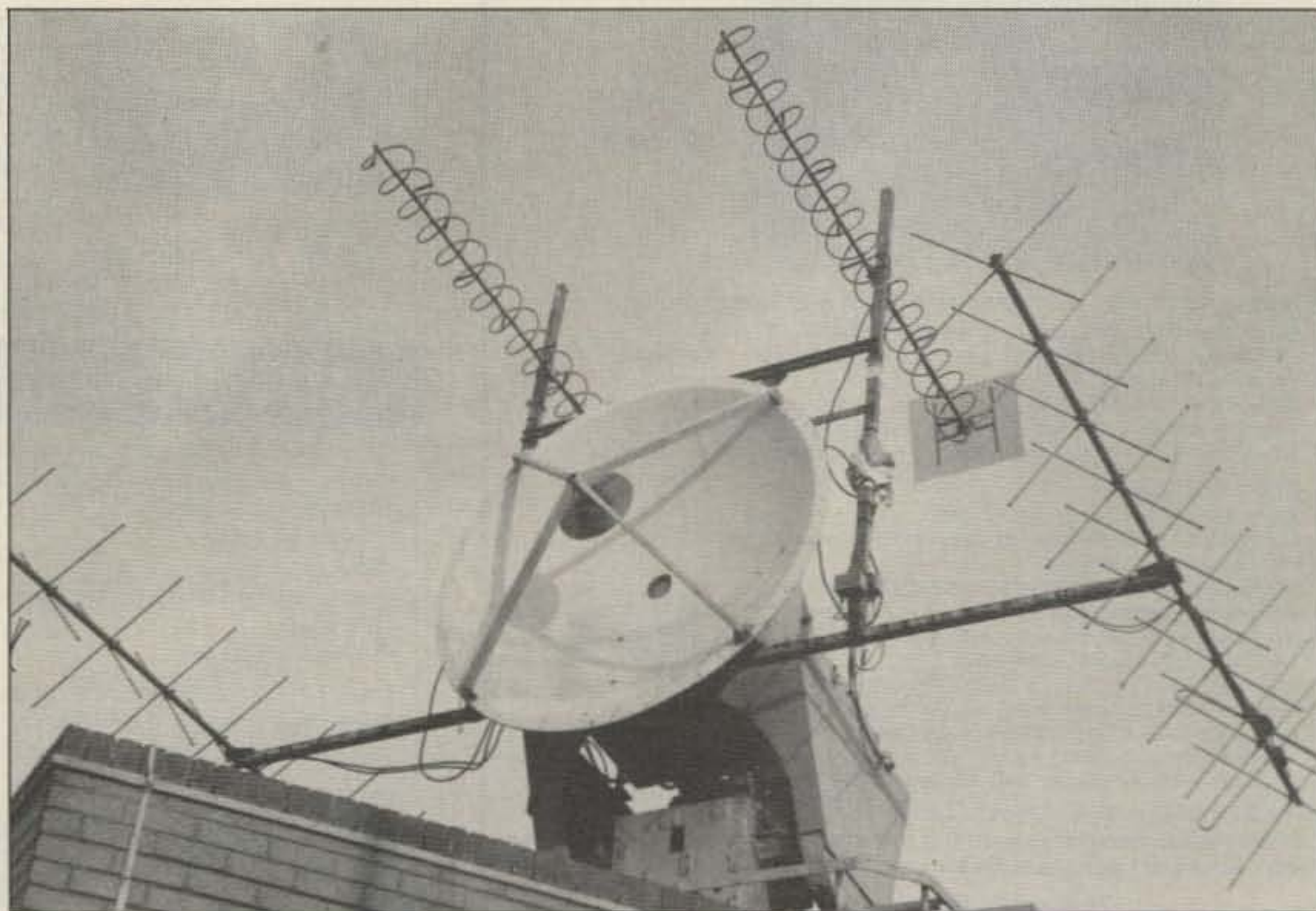
Photo C. Main University of Surrey satellite tracking antennas on a modified anti-aircraft gun mount. (N5FVM photo)
