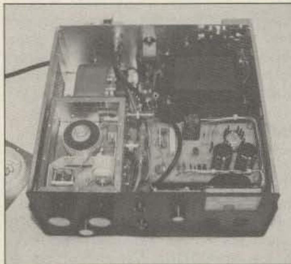
Photo B. Under the cover, a quiet fan keeps things cool.
