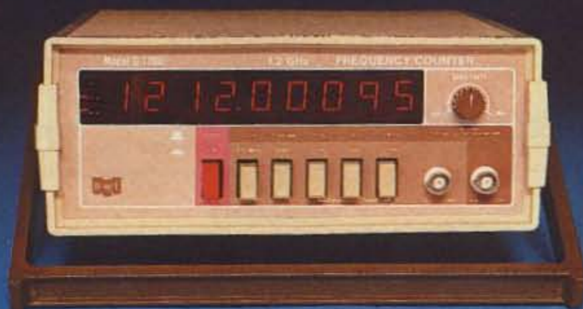
10 MHz Oven Oscillator 9 X 8 1/2 X 3 1/4 10 Hz to 1.2 GHz, 1 PPM ACCURACY
