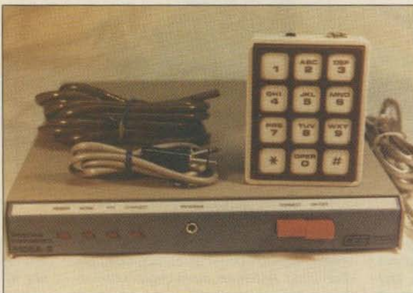
Photo A. View of the Smartpatch II with enclosed DTMF encoder and hook-up cables.
