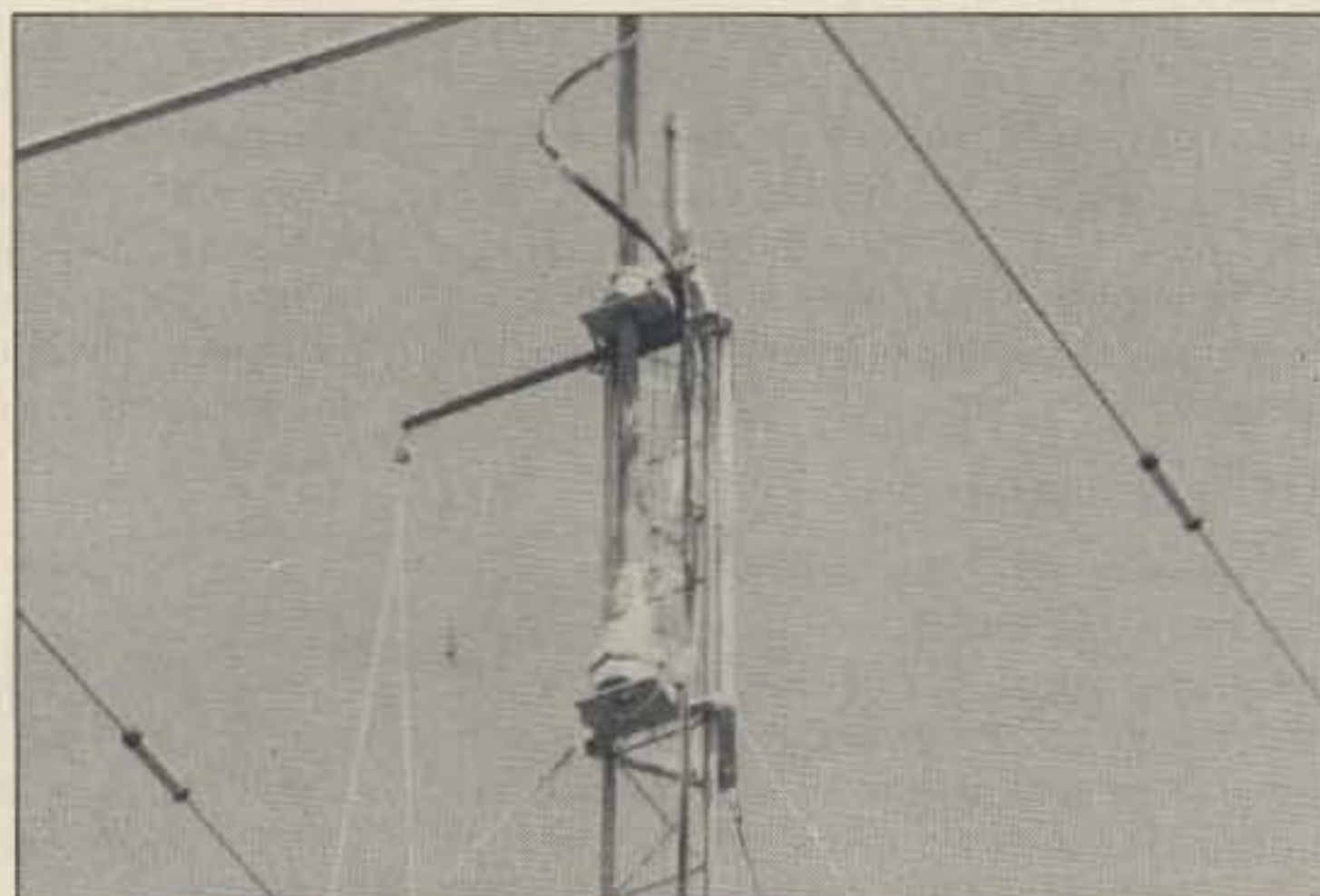
Photo E. The Hazer in action at the top of the tower.
