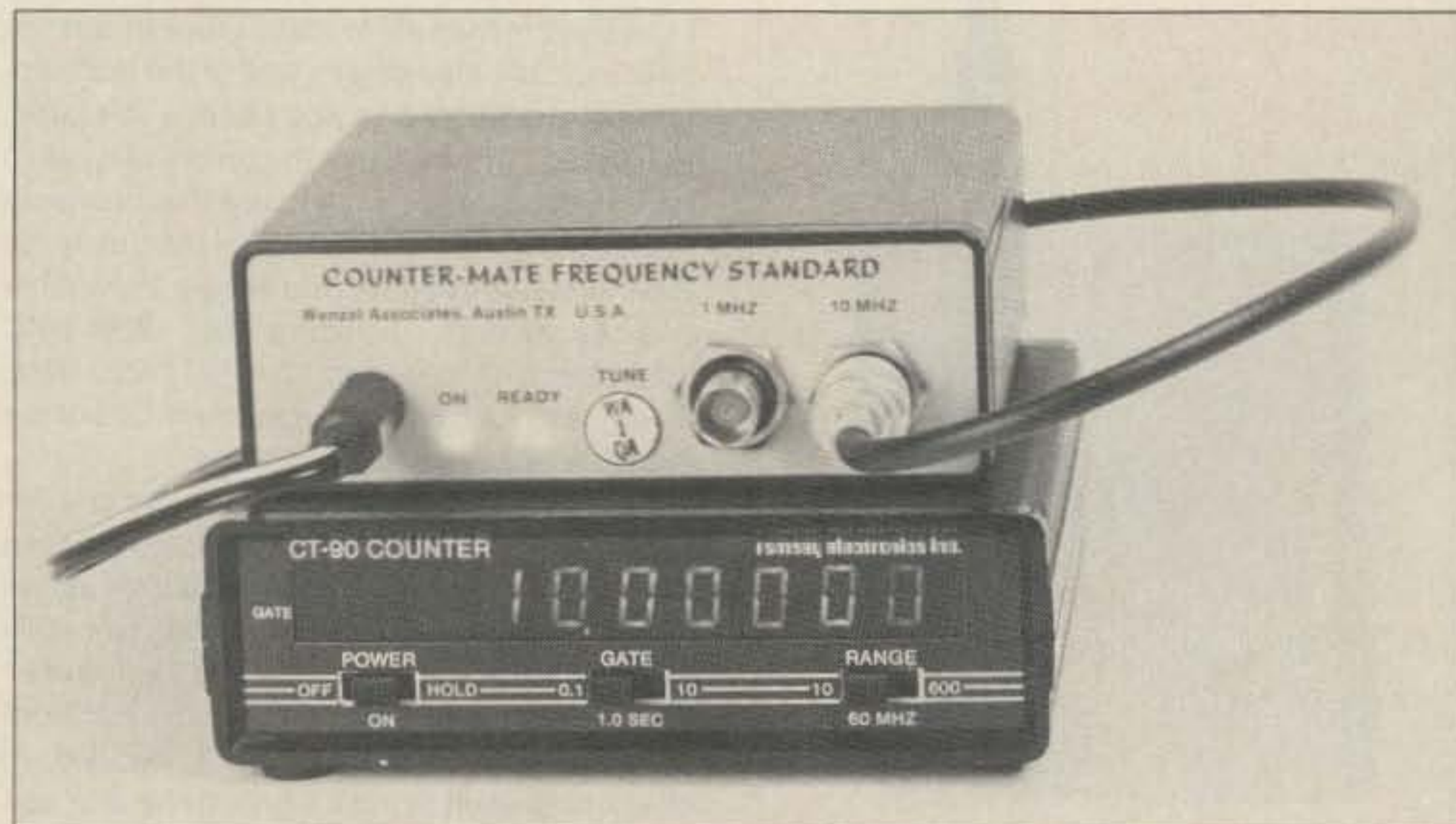
Photo B. Wenzel Associates Counter-Mate frequency standard (top) hooked up to a Ramsey frequency counter.
