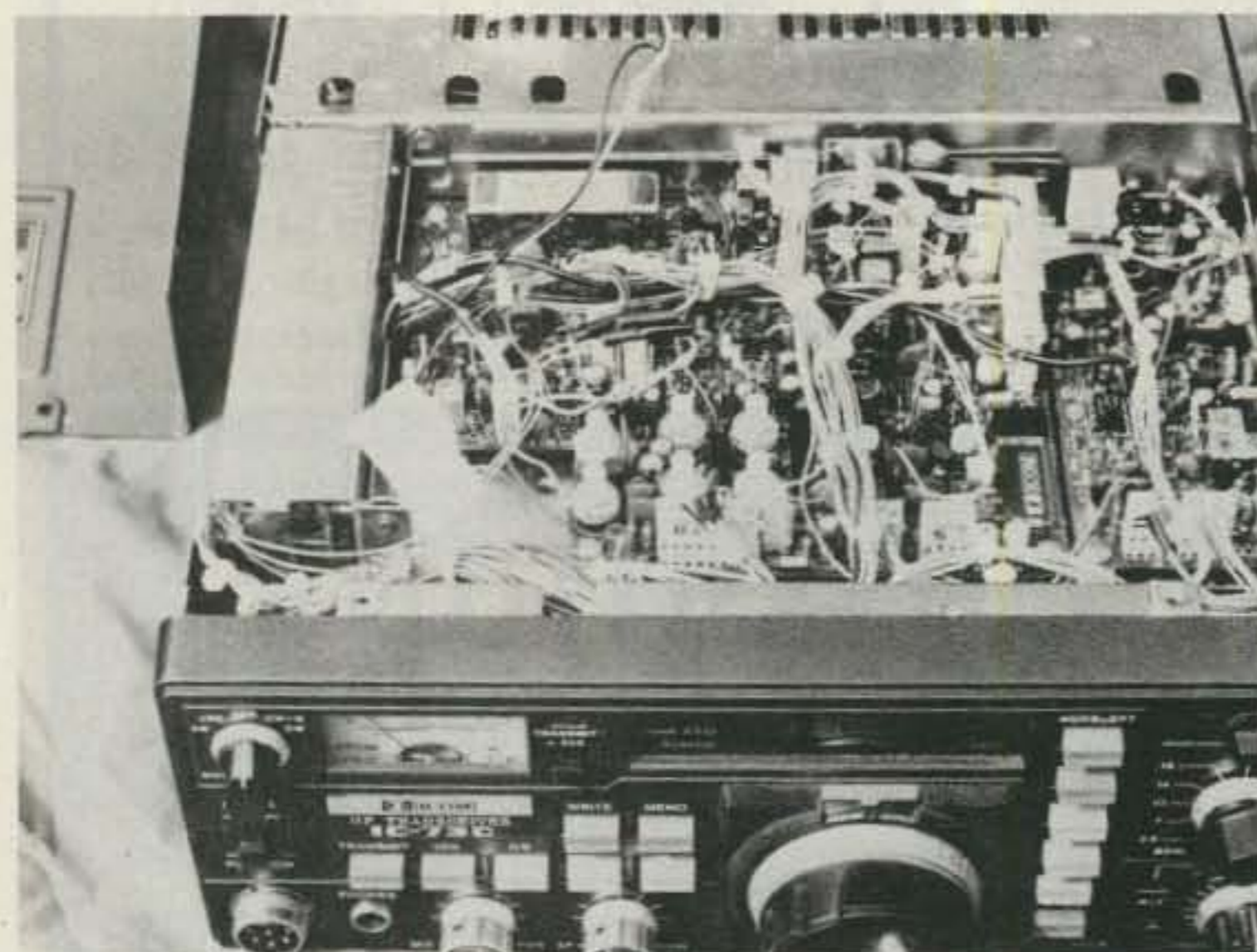
Top view: The wires for my modification are identified with white tape, here shown going to the pad 1 and pad 2 locations under the calibrate pot on the main board.
