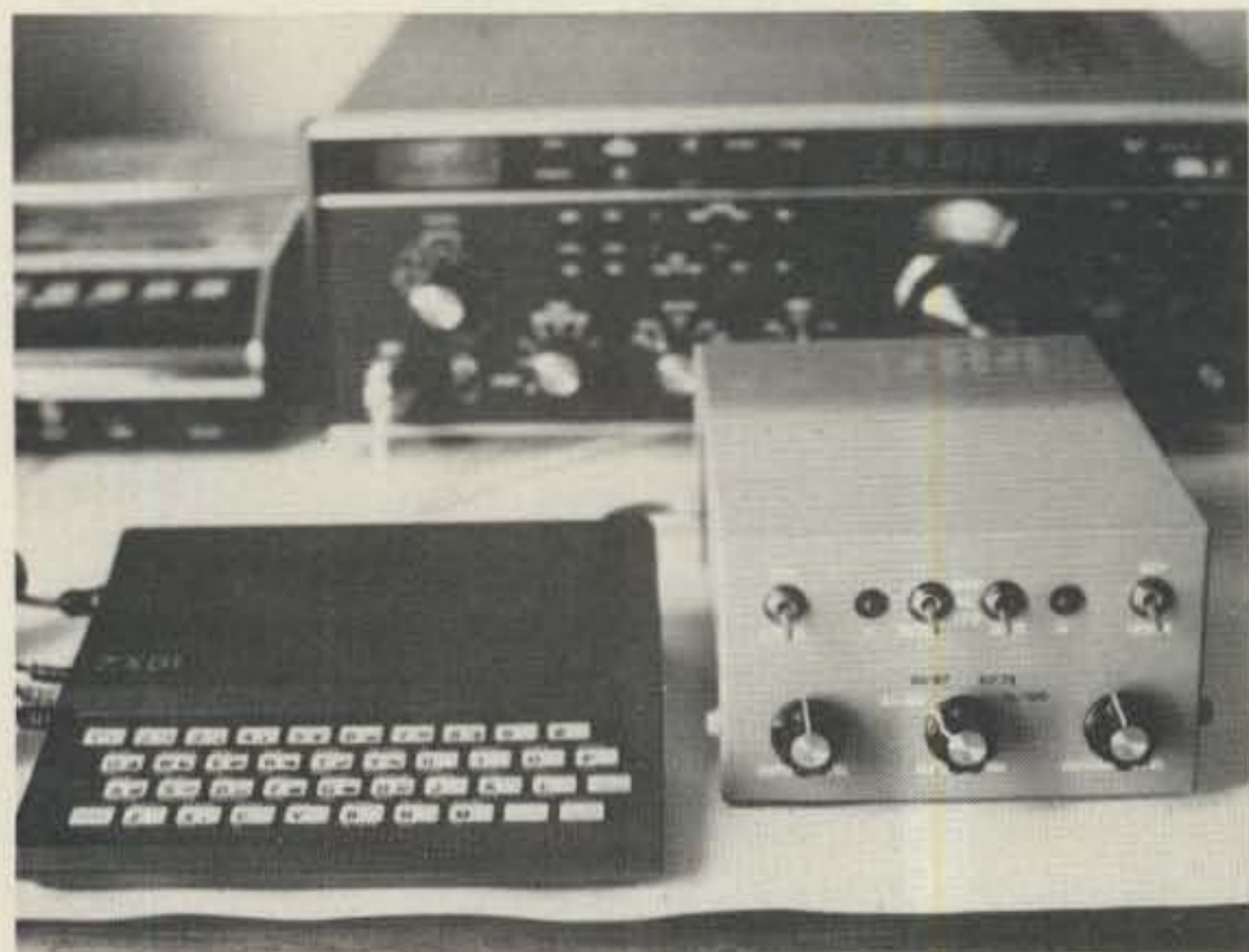
Photo A. The Timex/Sinclair computer, along with a TV, cassette recorder, interface unit, and a transceiver, make up the complete RTTY station.
