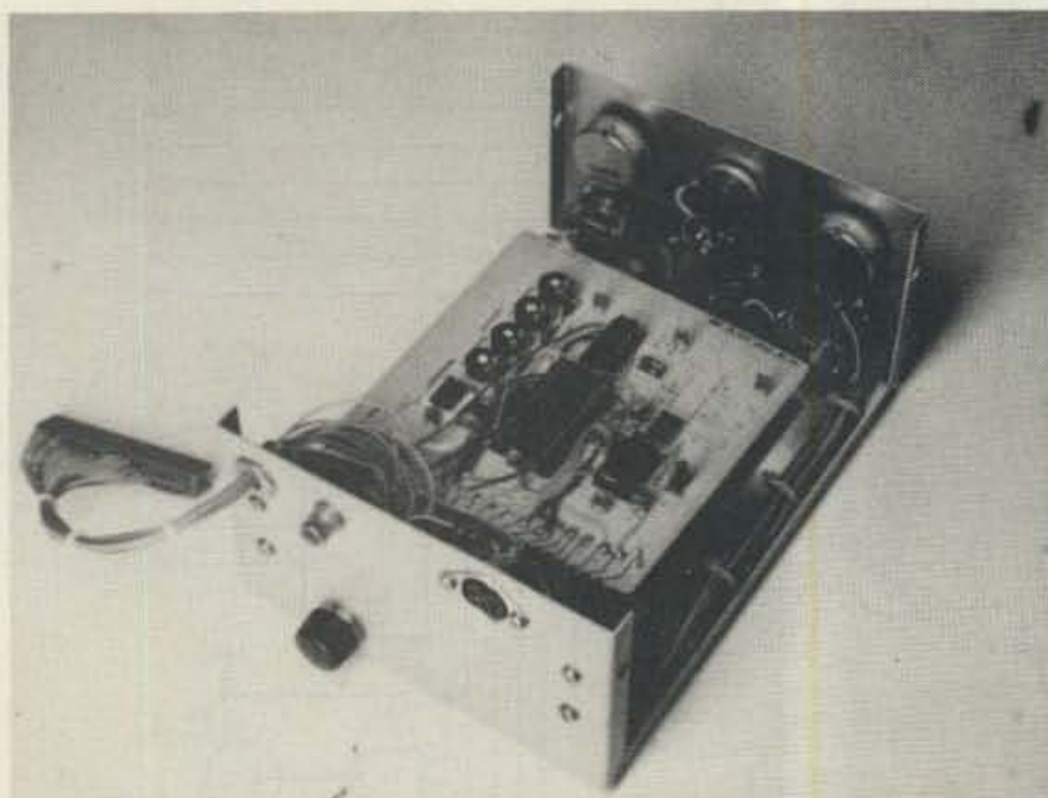
Photo C. The interface circuit was built on proto boards available at Radio Shack. The top board (shown) contains the digital portion of the circuit while the lower board contains the filters and tone generator and decoder chips. No printed circuit board is available. The DIN socket is used for the cable to the mike jack on the transceiver, and a standard phono patch cord connects receiver audio to the phono jack. Both of these cables should also have toroid chokes attached to prevent RFI. The knob on the rear panel controls the audio-monitor volume.
