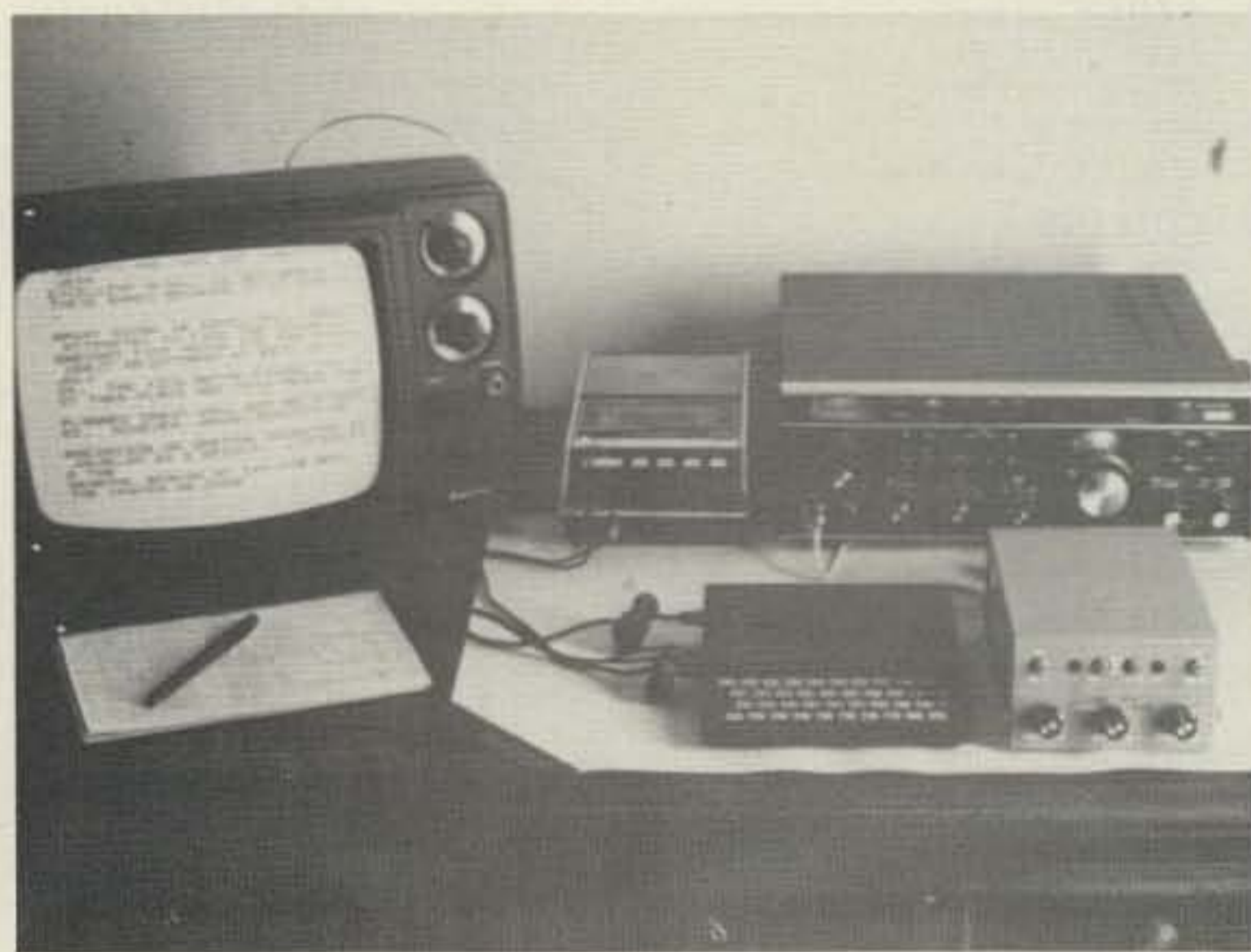
Photo B. The interface unit is versatile enough for the various amateur and commercial RTTY code-reception schemes, as well as 170-Hz and 850-Hz transmission using standard mark and space frequencies. Note the toroid rf chokes on the computer power and video cables.
