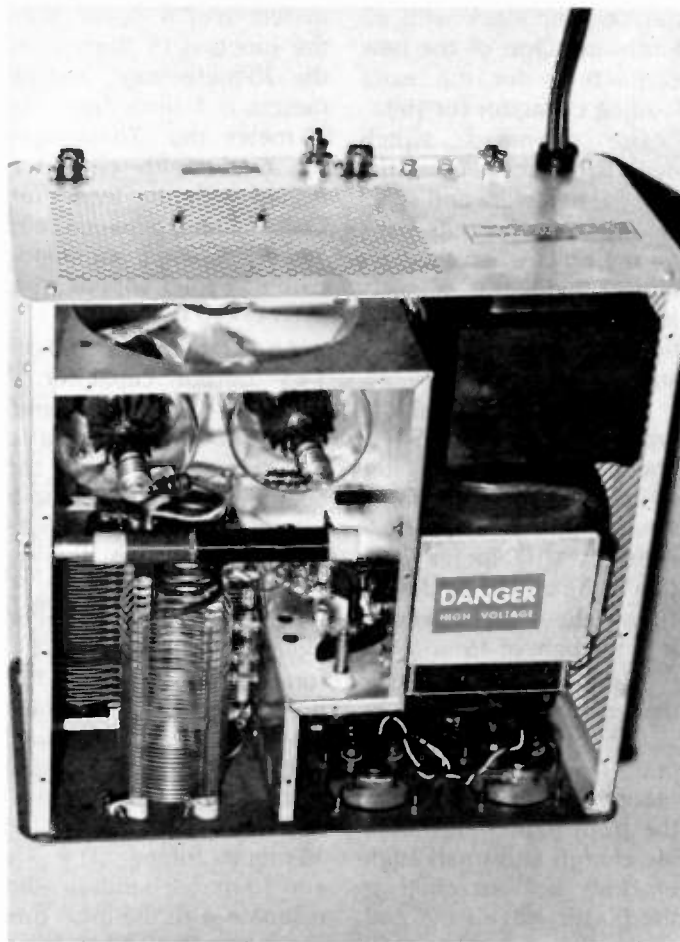
Photo B. The SB-221 converted for operation on 160 through 10 meters. The new tank coil is mounted on the front panel, using two holes that previously held a plastic Heathkit label. The new larger plate choke is mounted on the wall at left, using the original plate-choke standoff. The bandswitch is removed from the partition wall, modified, and replaced.
