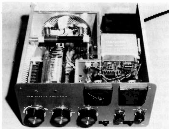
Photo D. Front top view of the modified SB-221. The two screw heads above the capacitor knobs are the only outward change in the appearance of the amplifier. The 160-meter position on the bandswitch is the one to the left of the 80-meter position; it need not be marked. Similarly, the 10-meter position is the one to the right of 15 meters.
