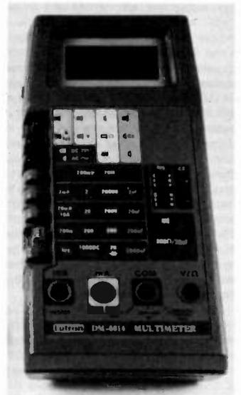
The MCM Electronics DMM/DCM meter.
