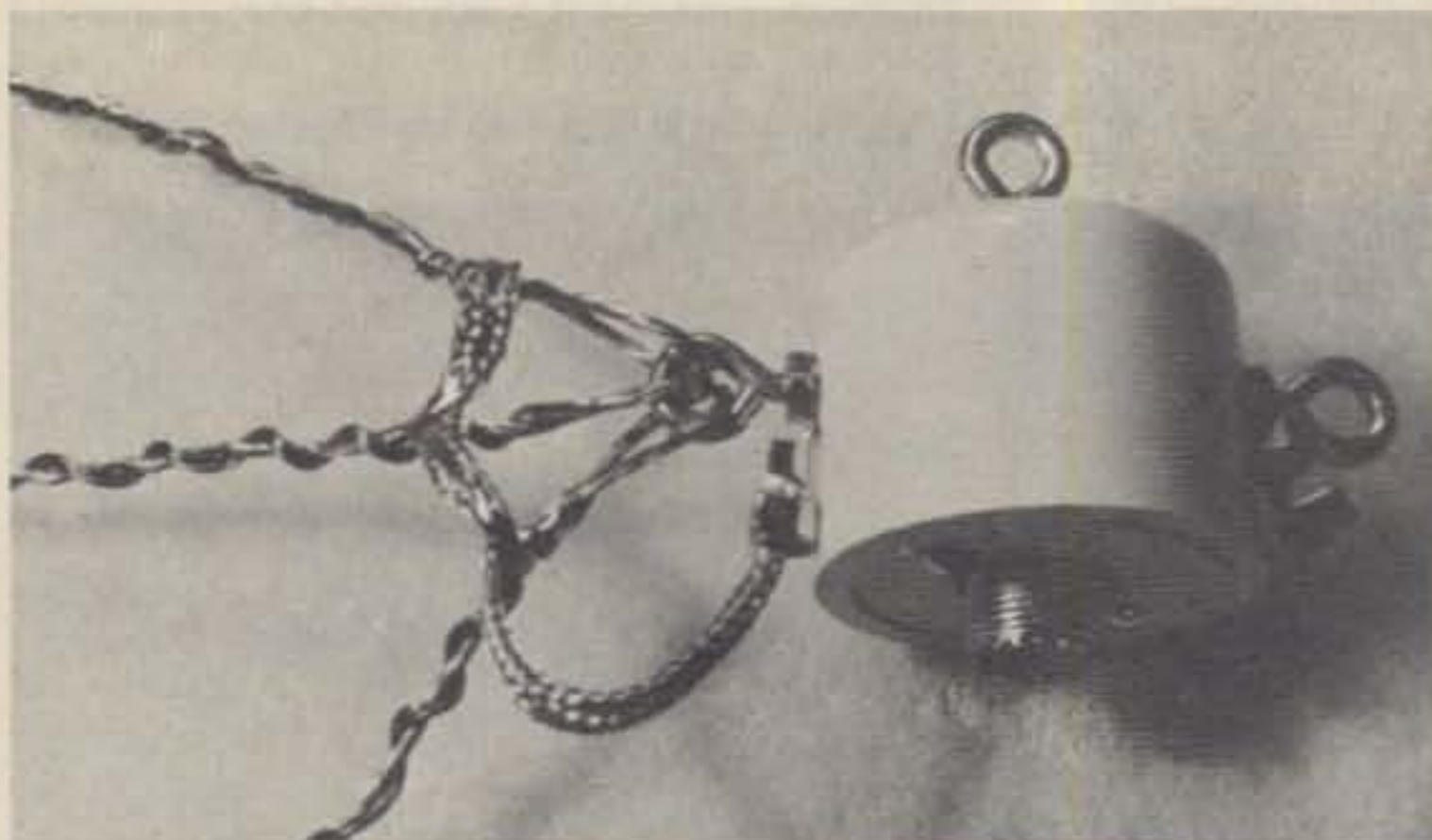
The center insulator with the left side of a 3-band antenna installed. Notice the use of the braid as a flexible connector line from the antenna itself to the center insulator lug.
