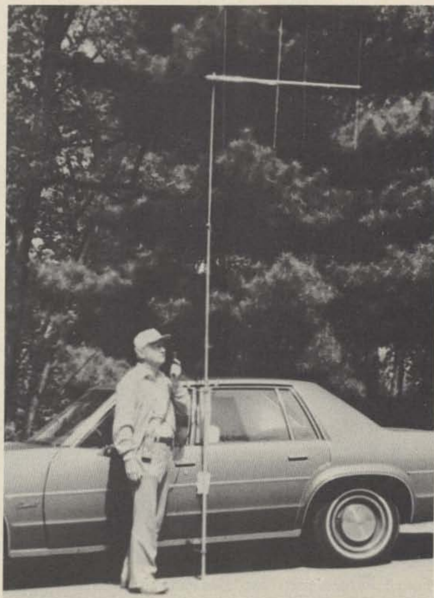
Photo D. Mast fully extended. Beam being used with HT.
