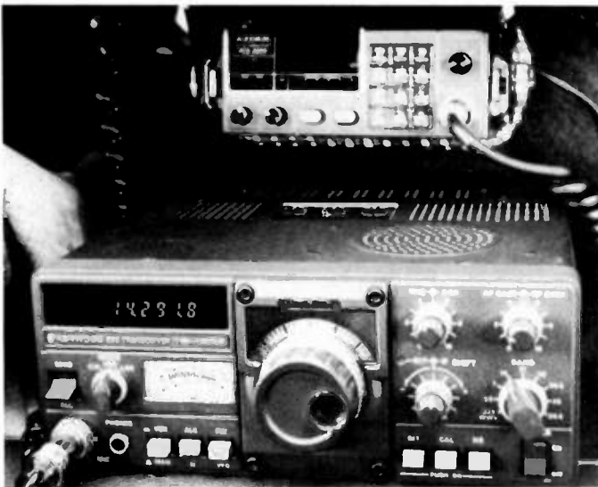
Fig. 7. Mobile installation of traveling amateur W4CEC consists of an Azden 2-meter rig and Kenwood TS-120. The 120 is merely propped on the auto's seat; its tilt-down front bail secures the unit and eliminates the need for a tie-down strap. The Azden is secured, complete with bracket, by a tie-down strap hooked under the dash. Clever and convenient, and both rigs can be removed in a snap.
