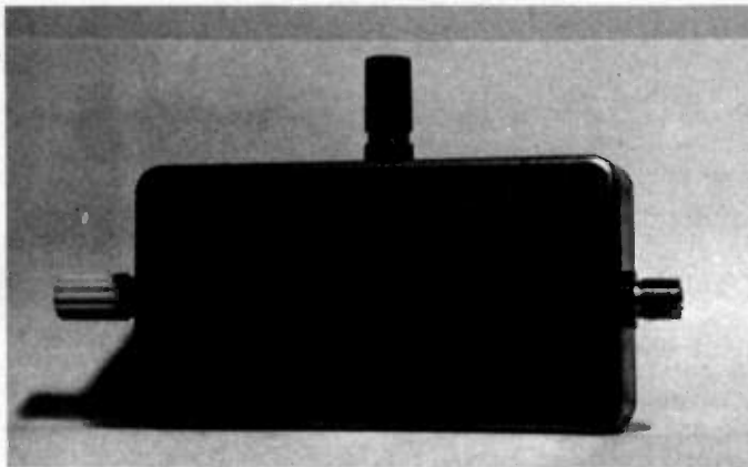
Photo C. Assembled and sealed Beverage Box. The system of three reversible Beverages at K1VR required six of these boxes.
