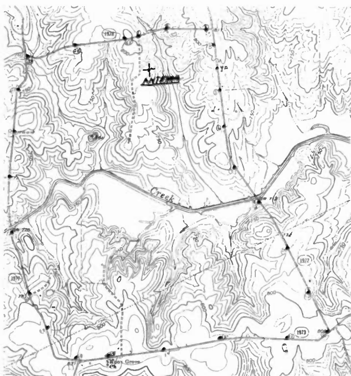
Fig. 1. Survey map showing antenna location and points where measurements were taken.
