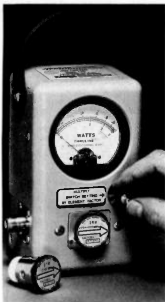
The Thruline® directional wattmeter.
