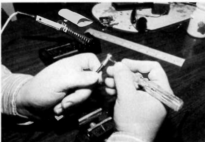
The next step in preparing coax is carefully debraiding the outer shield. For this you will need a sharply pointed scribe, ice pick, or other pointed tool.
