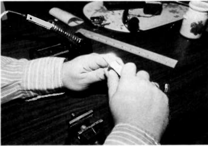
Cutting the outer covering of a piece of coax requires a sharp knife and a firm but gentle score around the plastic covering. If you cut too deeply, you risk cutting the outer braid of the coax.
