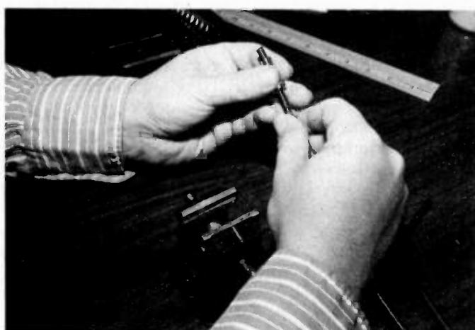
The first step in preparing this RG-58 cable for cutting is sliding the UG-175 adapter over the cable. This allows the use of a PL-259, which is actually sized for RG-8/U coax.
