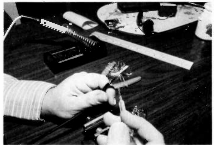
When you have finished debraiding the outer coaxial shield, it should look like this. Notice it is fanned at roughly a 90° angle. This fanned braid is then smoothed over the adapter and trimmed.
