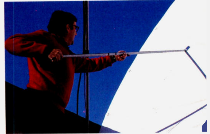
Fig. 3. A long pole or length of wall molding will reach anywhere on a dish and is safer. Tape the mirror to the pole like a hinge so it rests flat on the dish. Very few inexpensive dishes will pass this test. When you find one that does, buy it!
