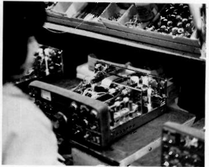
The empty chassis starts at one end and comes out with everything ready for testing.
