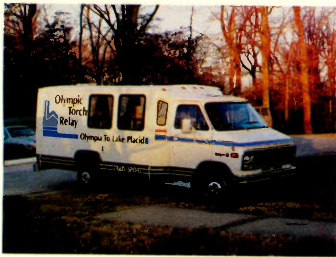
Photo C. One of the Chevy Trans-Sport custom vans used for Ceremonial, Command, and other positions. Having a fiberglass body, it required our own ground-plane metallic base with 19-inch radials attached to the body with duct tape.
