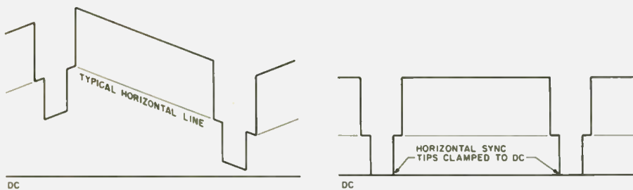
Fig. 4. (a) Video demodulator output showing video riding on energy dispersal wave. (b) Energy dispersal wave eliminated by dc clamp circuit.
