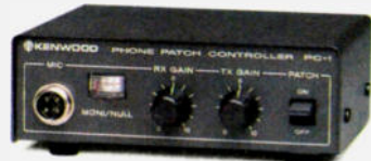
PC-1 phone patch with hybrid circuit and VU meter for null and audio gain measurements.
