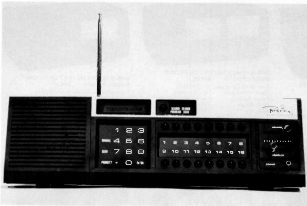
Photo C. The Digital Flight Scan is a programmable 108-to-136-MHz AM scanner for aircraft buffs.
