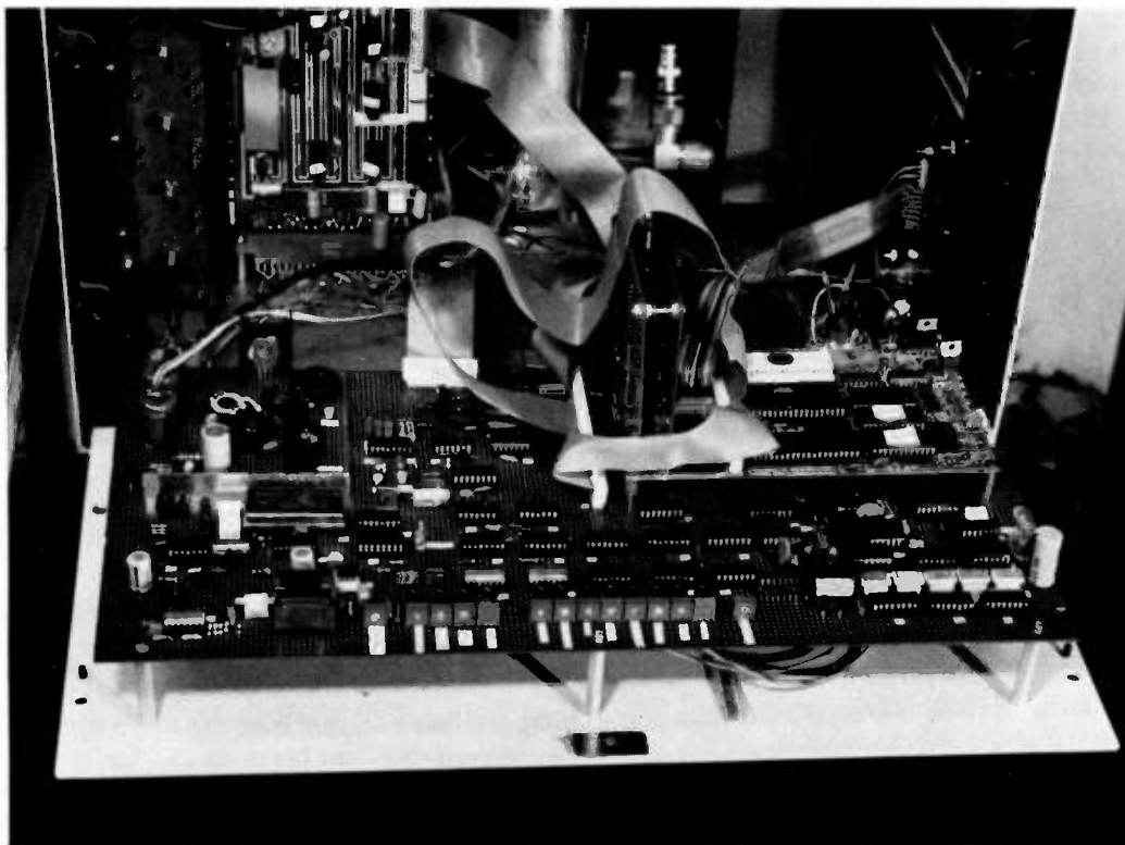
Photo C. Repeater control board. Main board mounts on the cabinet's "front door." Clockwise from upper right are CPU-1A microcomputer, audio delay line, audio mixers, phone patch, and dc-dc converter.
