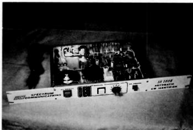
Spectrum's new ID 1000 CW station identifier.
