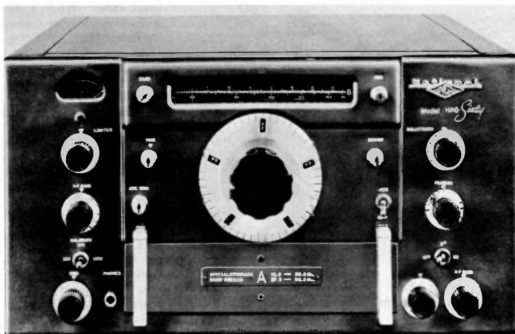
Fig. 5. The National HRO receiver. The first HRO, a 9-tube superhet, was introduced in 1934. All featured the famous "PW" HRO precision-ganged tuning condenser. The HRO-Sixty, shown here, came out in 1953. Photo courtesy of National Radio Company.
