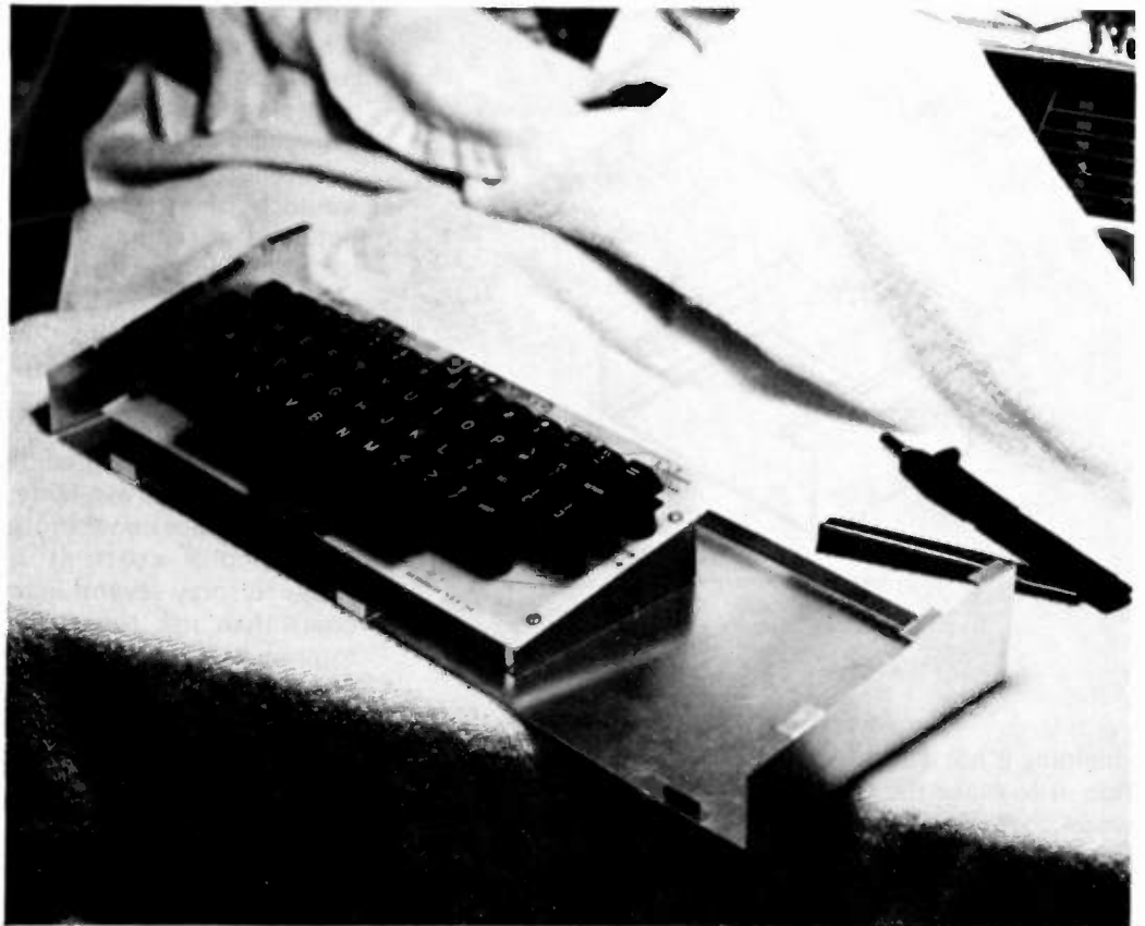
Photo C. The keyboard is placed in the base and positioned so that the top fits over it correctly; it then is glued down.
