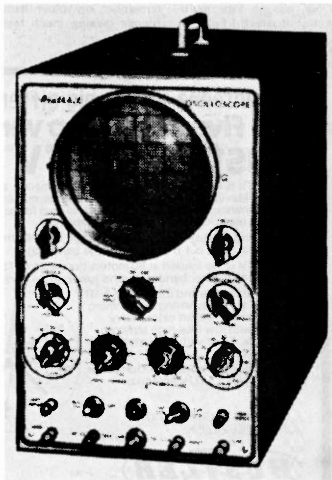
Fig. 6. Heathkit model "0-8" 5-inch oscilloscope, dc to 1 MHz, $43.50 in kit form in 1953. Drawing courtesy of Heath Company.
