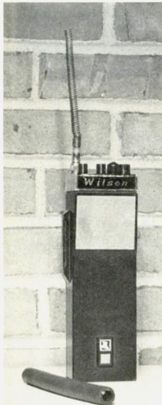
Photo A. Before. The beat-up rubber ducky before installing the replacement covering.
