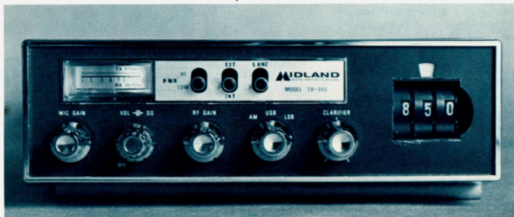
Photo A. The Midland, showing the BCD switch in place of the rotary switch. Notice that the switch is reading 850, which is an operating frequency of 28.50 MHz.
