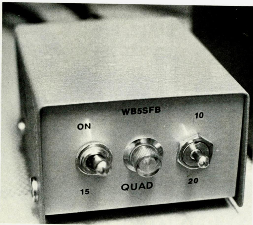
Photo A. Power supply unit.
