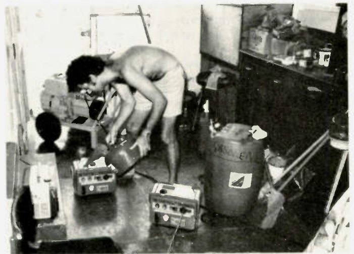
Photo S. The author refueling a portable standby generator of the type used by the Bajan (Barbadian) hams, in Dominica, to power their equipment. These small 300-Watt Honda generators allowed continuous radio operation for about six hours on a half gallon of gas. They were used for about a week prior to Barclays Bank providing a 1.6-kVA diesel generator, shown in the background. This larger generator allowed the operation of a refrigerator and lights at night, in addition to radio equipment.
