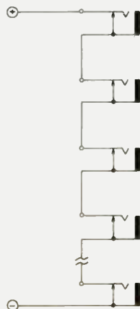
Fig. 3. Jack strip wiring.
