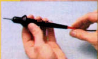
X10 DCV probe adapter available for protecting input jack 10KV.
