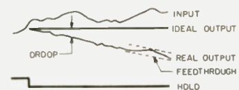
Fig. 6. Representation of the linearity, droop rate, and feedthrough. (Courtesy of Analog Devices, Inc. 3 All rights reserved.)
