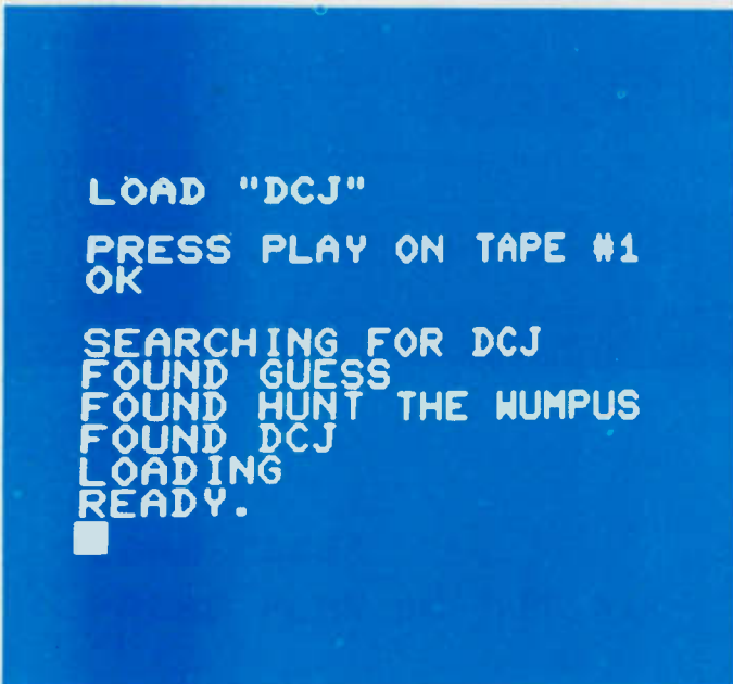
Photo 4. Video display showing sequence of operations to load a program "DCJ." Programs preceding it on the tape are listed, but not loaded. Sequence is fully automatic after user presses "PLAY."
