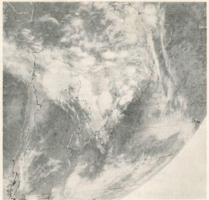
Fig. 8. A SE IR quadrant from GOES E showing most of South America. In the IR format, cold objects (space, high clouds) appear white with warmer objects appearing darker. The Andean uplands show noticeably whiter (cooler) than the lowlands. Low cloud cover over the Atlantic off the coast of Brazil is quite close to sea temperature and thus does not show strongly.
