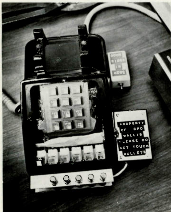
Five lines control the telephone ready to be operated by blind persons.
