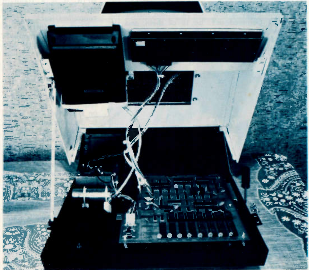
Photo 2. View of interior case. Note single-board CPU, simple power supply, cassette recorder mounted by a bracket, and general ease of access.
