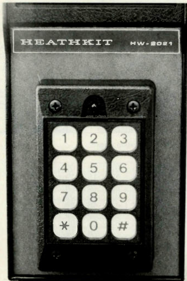
The HWA-2021-3 autopatch encoder modified for crystal frequency control.
