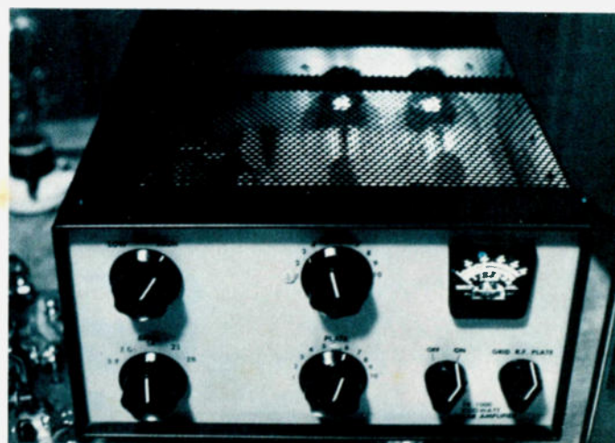
Classic amplifier in service and operating normally. The 4 811As add a soft glow to any ham shack. Room is dimly illuminated for slow scan TV operations.
