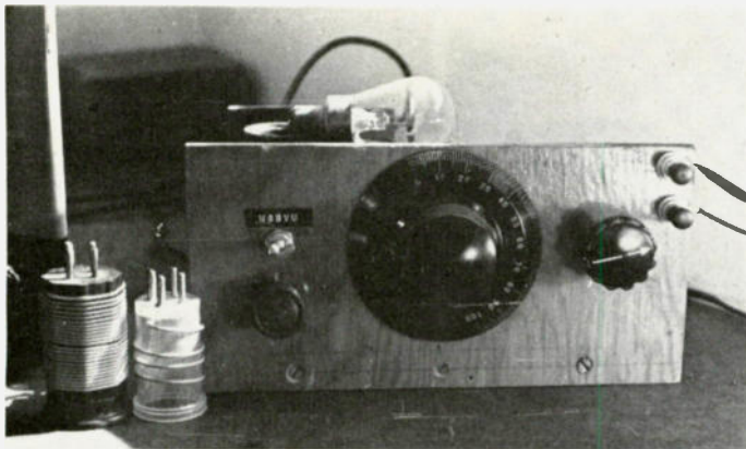
"Old reliable" antenna tuner — front view. This shows the neon tube and the 80 and 15-10 meter coils.
