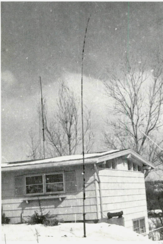
"Vertical zepp" antenna for 20 meter CW.
