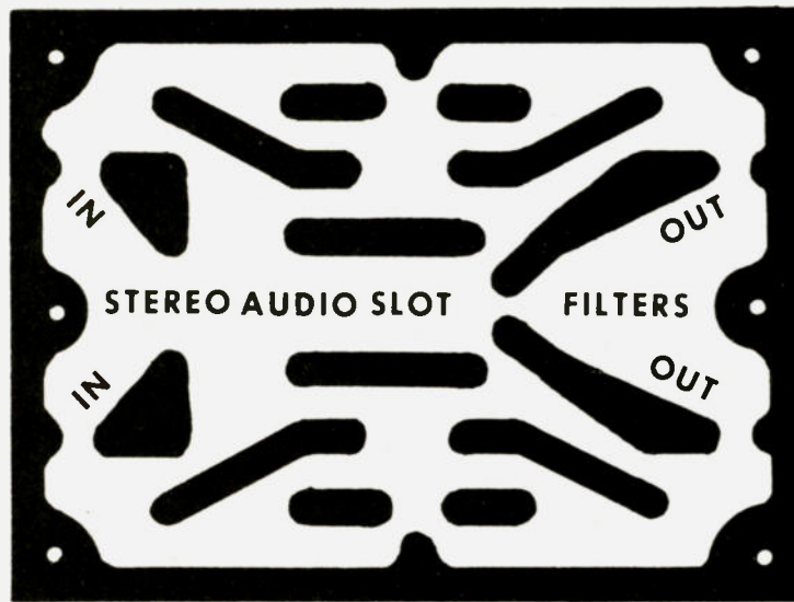
Fig. 2. Copper foil pattern.
