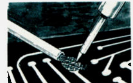
With D5, you can shape or web the wick for greater absorbency
