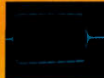
Keyed Waveform Shows detail of CW keying. Use to monitor the quality of your CW note. (Photo shows ideal waveform produced by TS-B205.)
