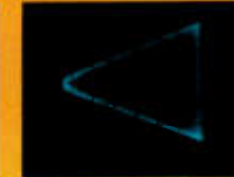
Trapezoid (TS-B20S w/ TL-922) Shows linearity of power amplifier. Used primarily for testing.
