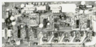
SCAP Autopatch Board
