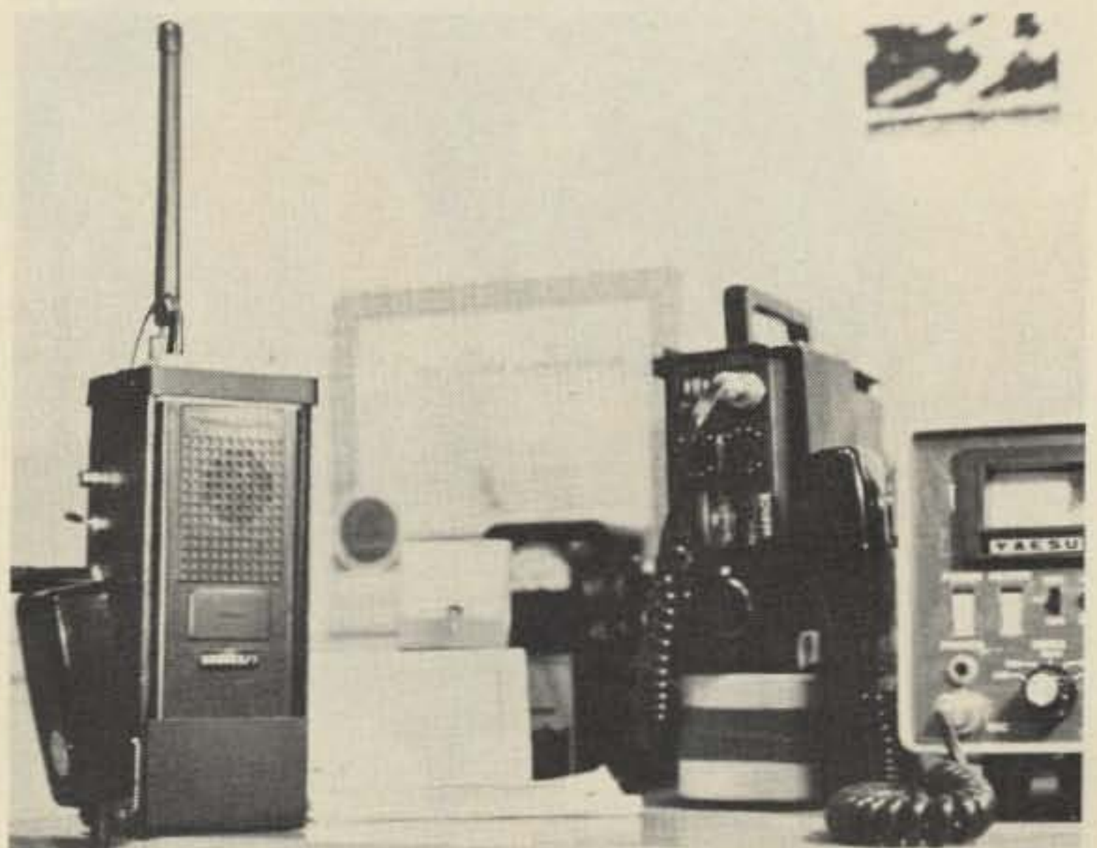
Photo 3. Close-up of talkie with author's other ham gonk. Rubber ducky installed; microphone on its bracket.
