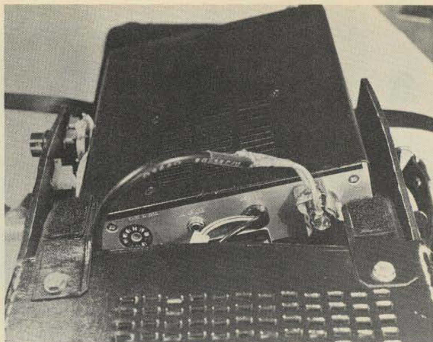
Close-up of transceiver rear panel with coax connector.
