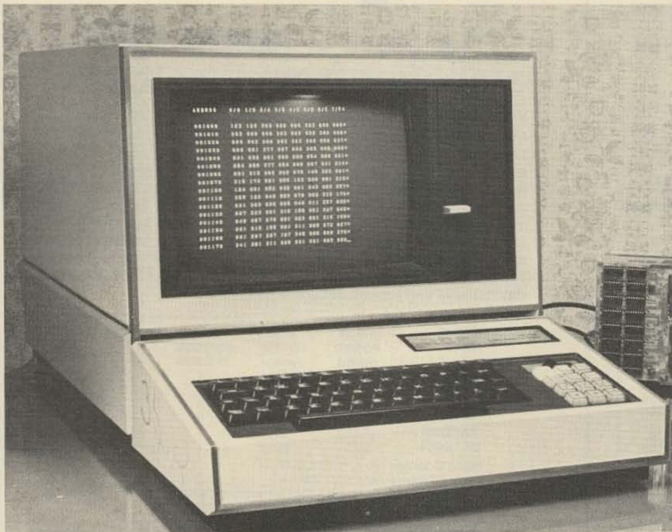
Photo 1. The RCA 70/752 Video Data Terminal has a hidden door to the right of the screen concealing controls for the display and alignment of the character generator. The keyboard can be moved up to one foot away from the display.
