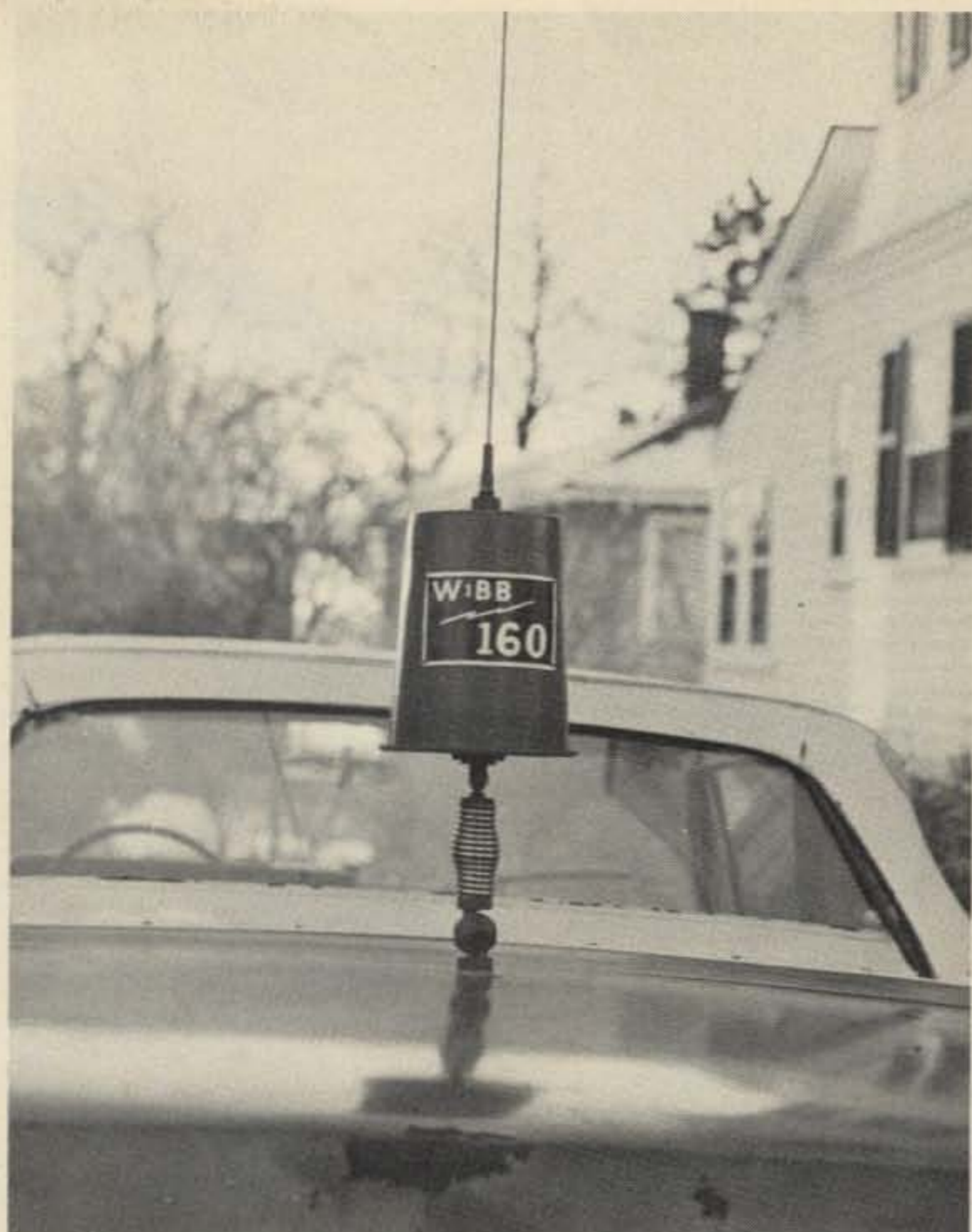
Whip antenna mounted on W1BB's auto. The loading coil is covered with a plastic trash can. Stew worked mobile on 160 meters for over 25 years, using both AM phone and CW.
