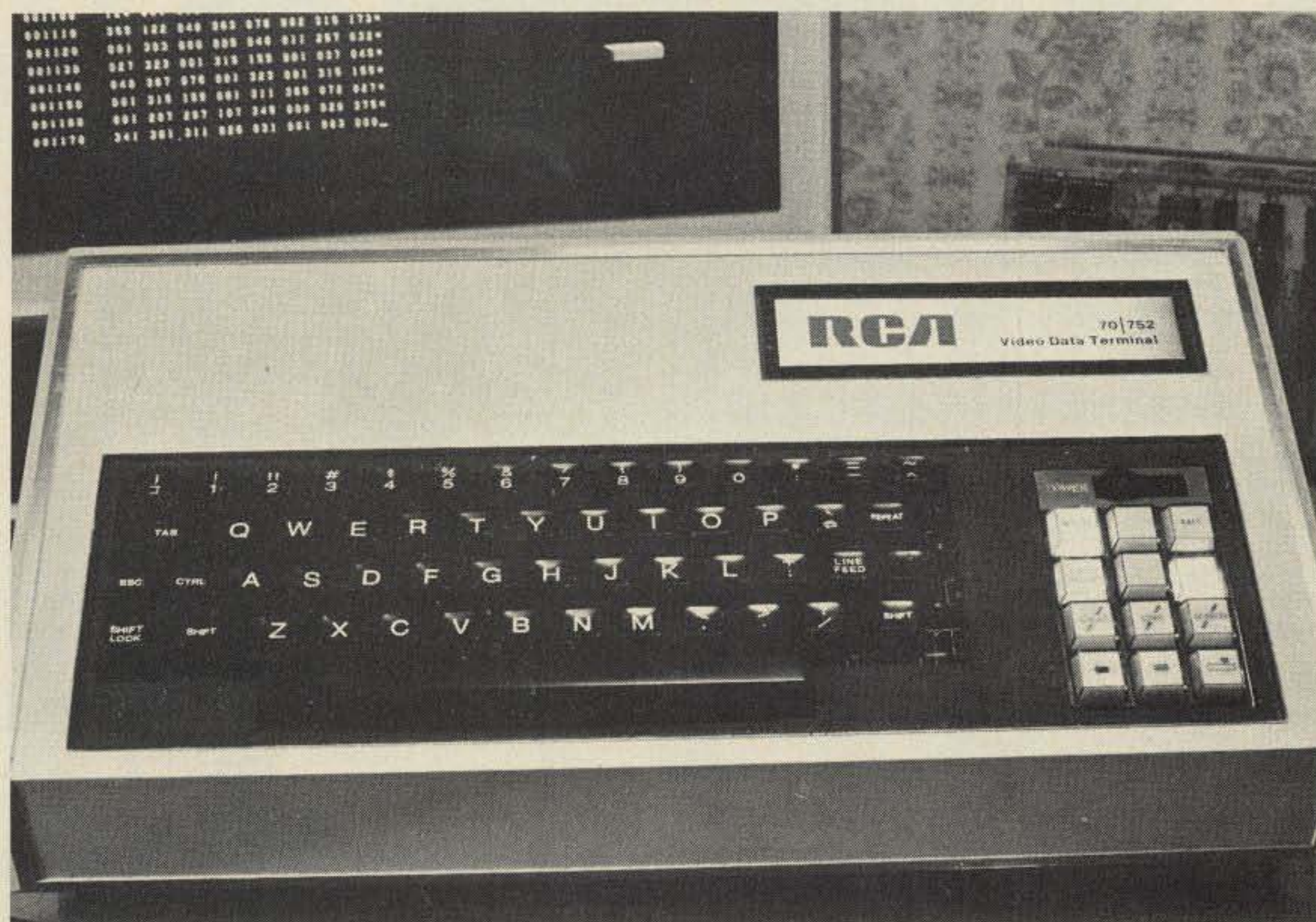
Photo 2. The mechanical keyboard was replaced by an electronic keyboard. The cursor and editing controls are on the right side of the control console.
