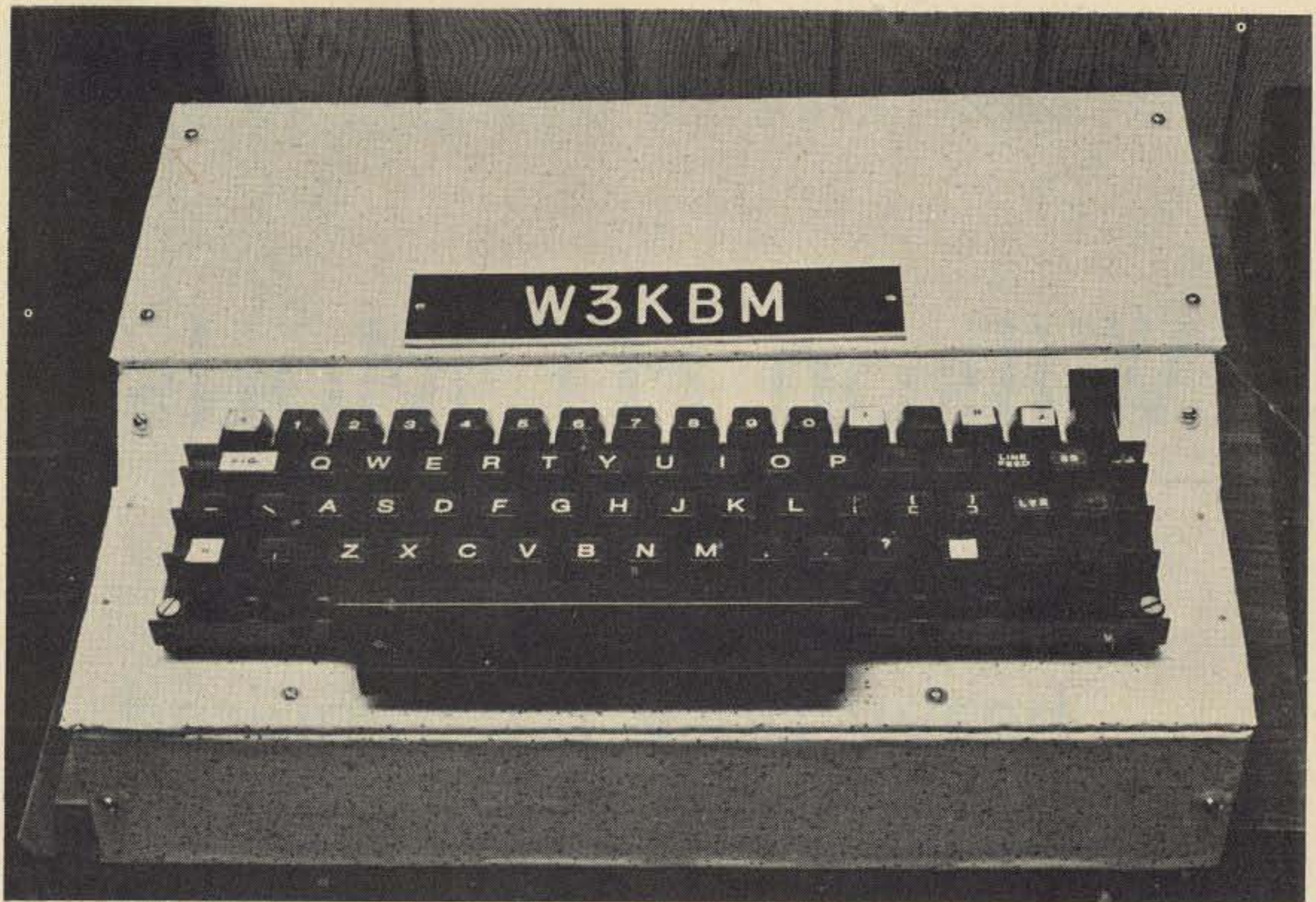
Finished keyboard. Black rectangle in upper right hand corner of small slanted panel is the LED figures/letter indicator. Note that some of the keyboard characters graphics such as the # sign had to be added so they appear on their own key. Also note that, as with most of these keyboards, most of the keys, particularly the numbers row, had upper case symbols above the numbers. They were blacked out with the aid of a resist pen. This accounts for the clean uncluttered look of the keys.
