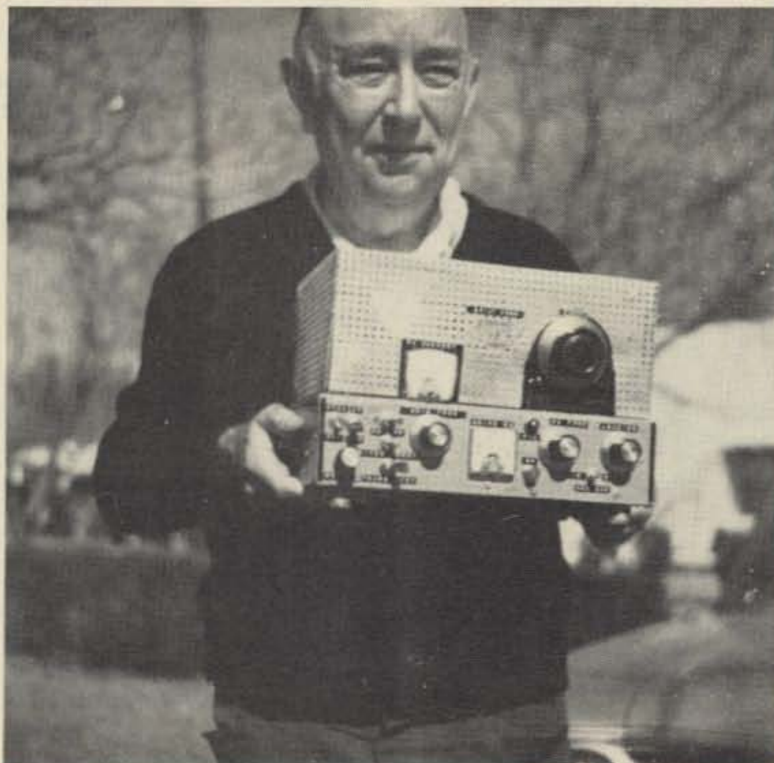
John Conner holds his home brew transmitter built from his old TV.
