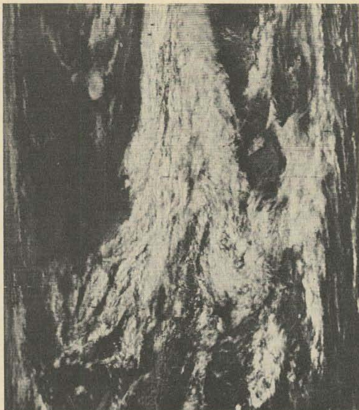
Fig. 5. NOAA 4 picture readout as received with the omni antenna system and displayed on the author's CRT monitor (the latter is described in the 73 Weather Satellite Handbook). The portion of the pass photographed extends from Hudson's Bay in the north, south to the central United States. Lake Superior is faintly visible in the lower left of the picture with the lower Great Lakes covered by a massive frontal system that wraps around from the central U.S. up the east coast of the U.S. and southern Canada. Extremely heavy rain was falling as this picture was received, indicating that the antenna performs effectively under adverse weather conditions. The satellite signal remained full quieting until it reached the latitude of central Mexico.
