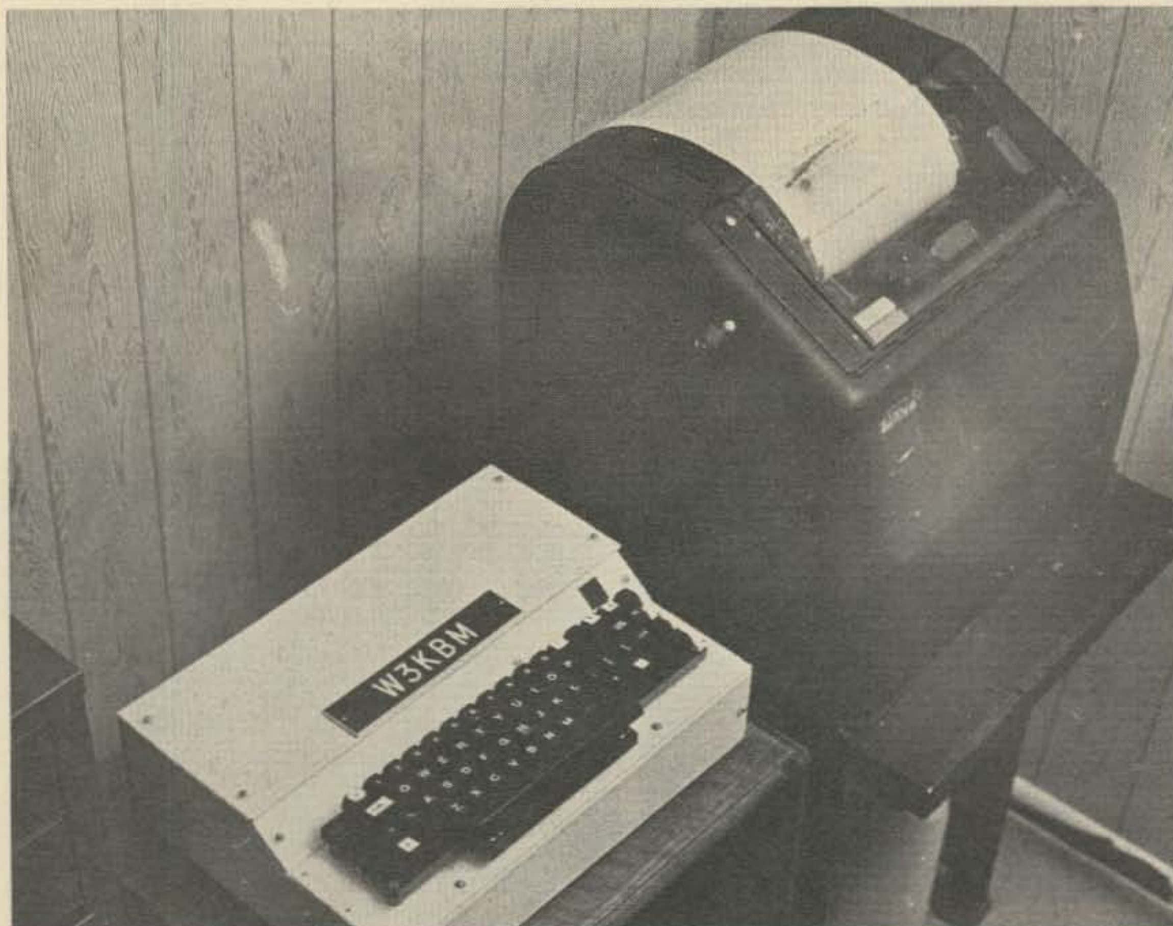
The keyboard with the RTTY machine that it serves.
