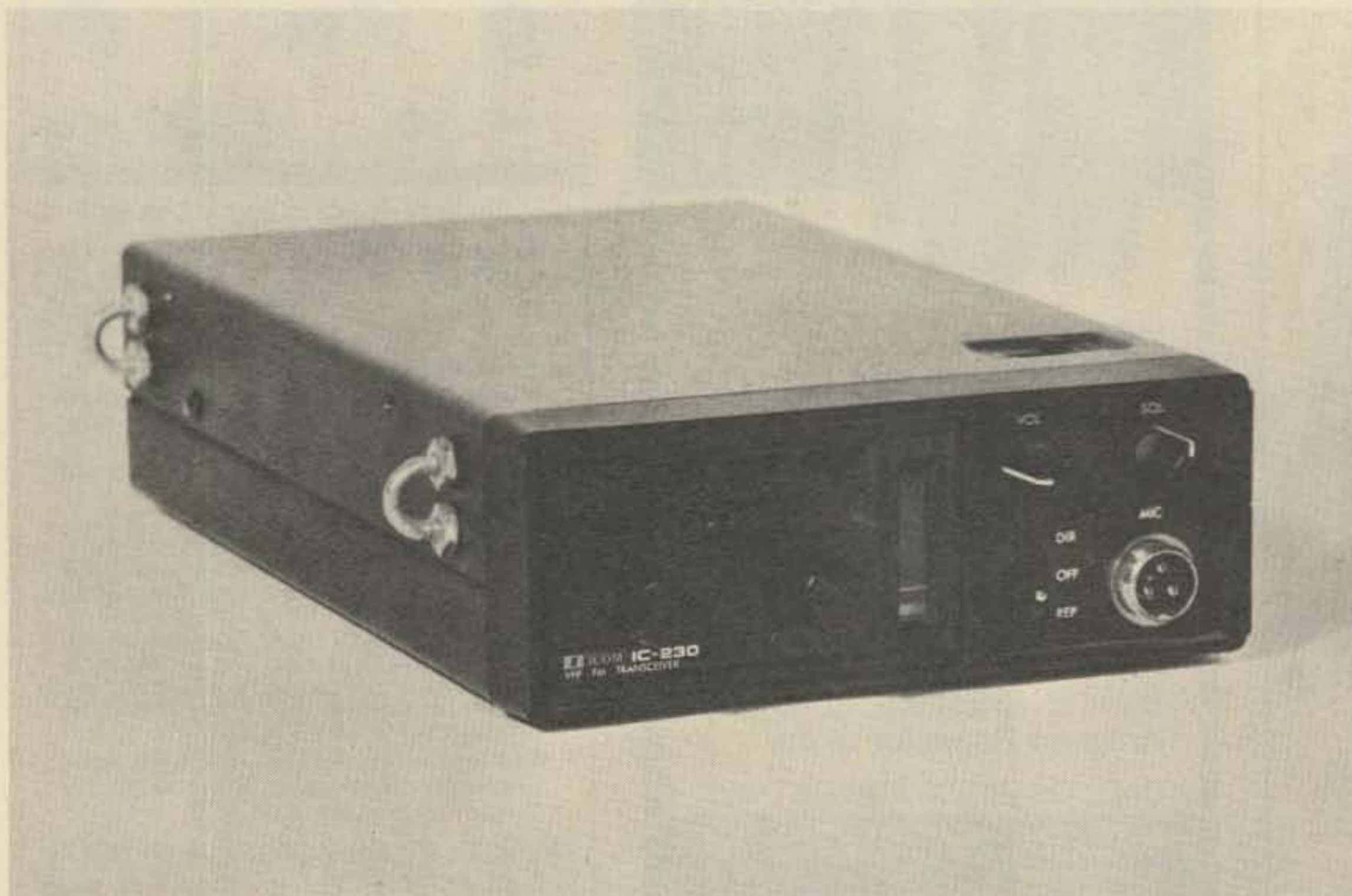
Front view of the IC-230, showing location of the "normal-split" frequency switch. Moving the toggle to the right increases the frequency shown on the front panel by 15 kHz.
