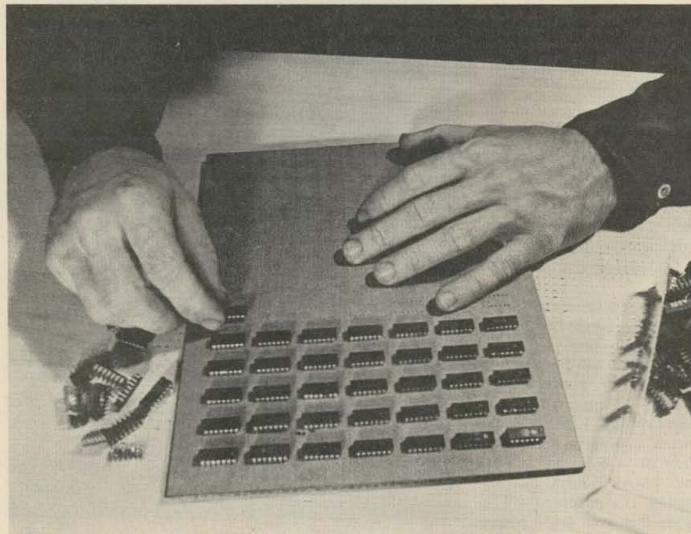
After all the holes have been punched, the graph paper is removed from the cardboard and the chips are inserted.
