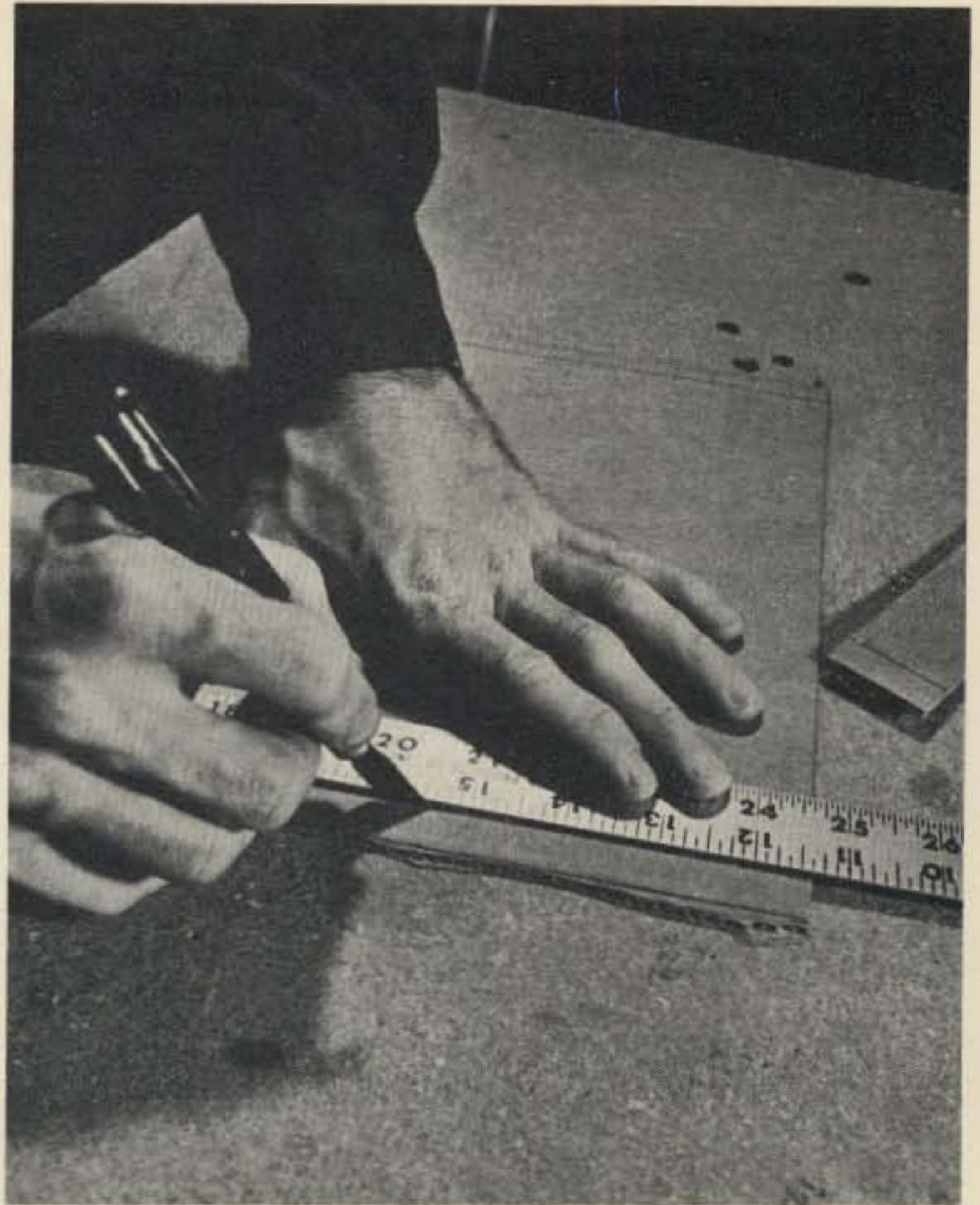
Use a metal ruler or yardstick and a knife to cut a piece of cardboard to the desired size.
