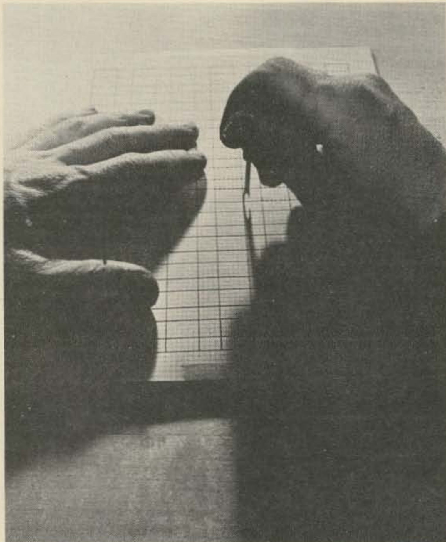
After the graph paper is properly ruled, it is cut to the same size as the cardboard and attached to it with masking tape. Then, each of the seven intersections on the segments of the horizontal lines measuring six spaces in length are punched. The tool shown in use is called a Seam Ripper, normally used in sewing.
