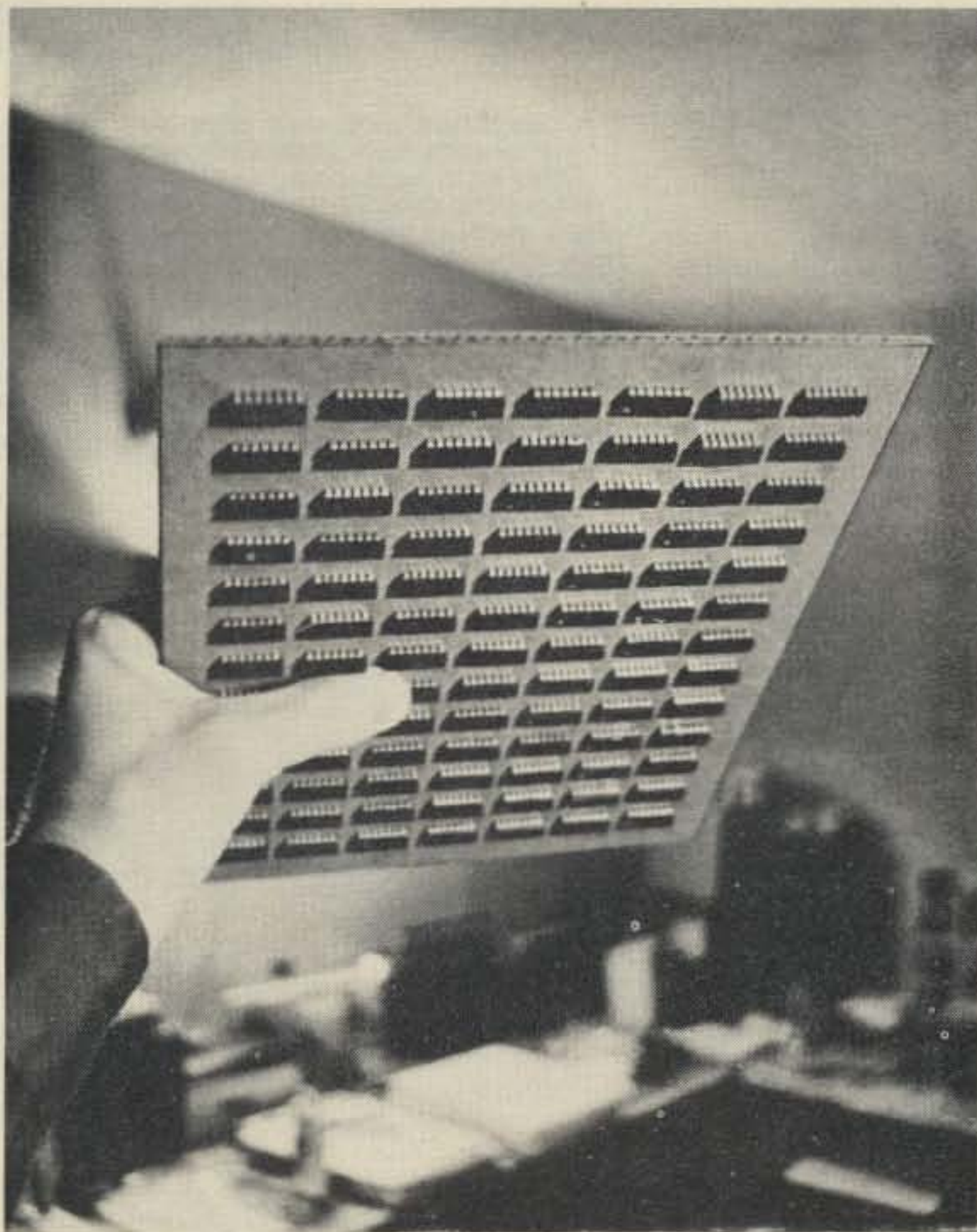
This fully populated board is being held upside down to show that the cardboard will hold the chips quite securely.
