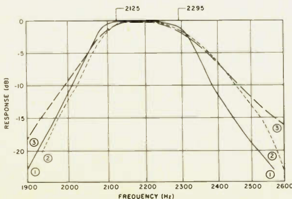
Fig. 9. Response of two LC filters and one active filter.
