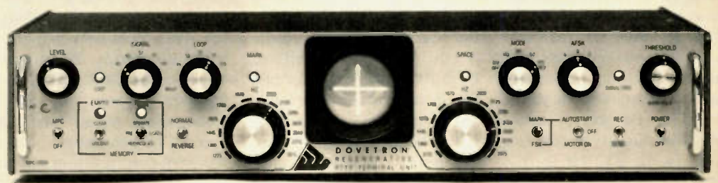
Photo 5. The Dovetron MPC-1000R is the Rolls Royce of terminal units. Some of the special features of the unit are electronic speed conversion, signal regeneration, a character memory up to 200 characters, error correction to erase misspelled words, Tee Dee inhibit, and variable character rate. Front panel controls permit "signal" and "loop" speed selections of 60, 67, 75, 100 wpm Baudot and 110 baud ASCII. (Photo courtesy of Dovetron.)
