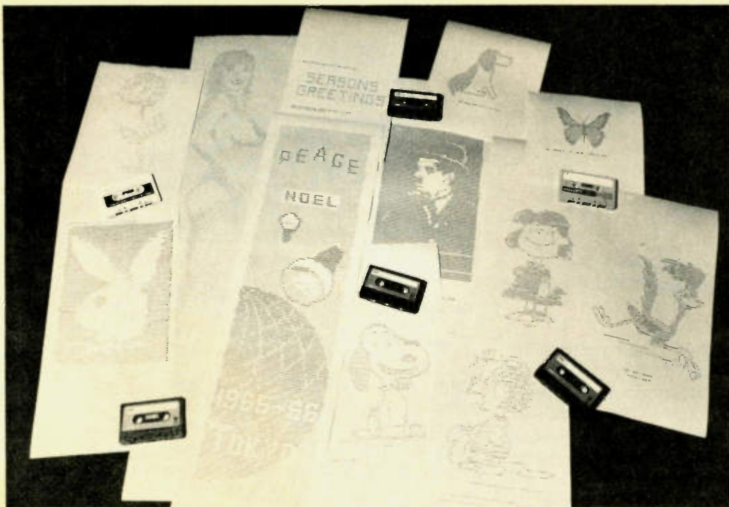
Photo 8. Shown here is a small sampling of some of the RTTY pictures that are exchanged on the ham bands. The small uncomplicated pictures require approximately 10 minutes to reproduce at 60 wpm, while some of the large pictures with overlining can require an hour or more. The RTTY Journal sponsors an annual RTTY art contest for those interested in this facet of RTTY. The pictures were stored on the cassettes shown in the photo. (Photo by Anthony R. Donaldson.)
