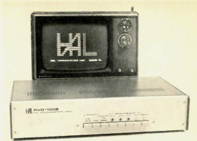
Photo 7. The RVD-1005 visual display unit is the modern answer to the teleprinter. The unit accepts demodulated Baudot signals at 60, 66, 75, and 100 wpm and displays the information on 25 lines with 40 characters per line. (Photo courtesy of Hal Communications Corporation.)
