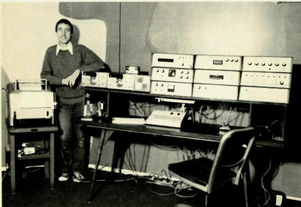
Photo 1. The author and friends. The basic RTTY equipment includes a Model 15 teleprinter, an ST-6 demodulator, and an AFSK modulator. The amenities include an electronic keyboard; a CRT RTTY tuning indicator; a UT-4 for signal regeneration and electronic speed conversion; a digital date, time, and message generator for the Selcal and W-R-U system; and a cassette tape recorder for storing and transmitting data. (Photo by Anthony R. Donaldson.)
