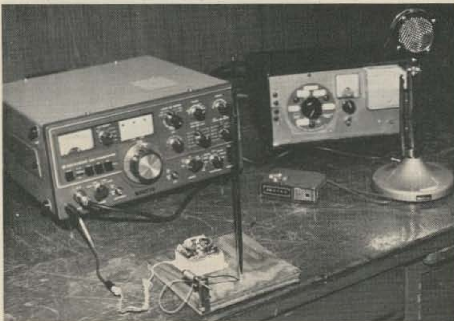
Fig. 6. Broadcaster (with cover removed) connected to antenna coil and whip antenna.
