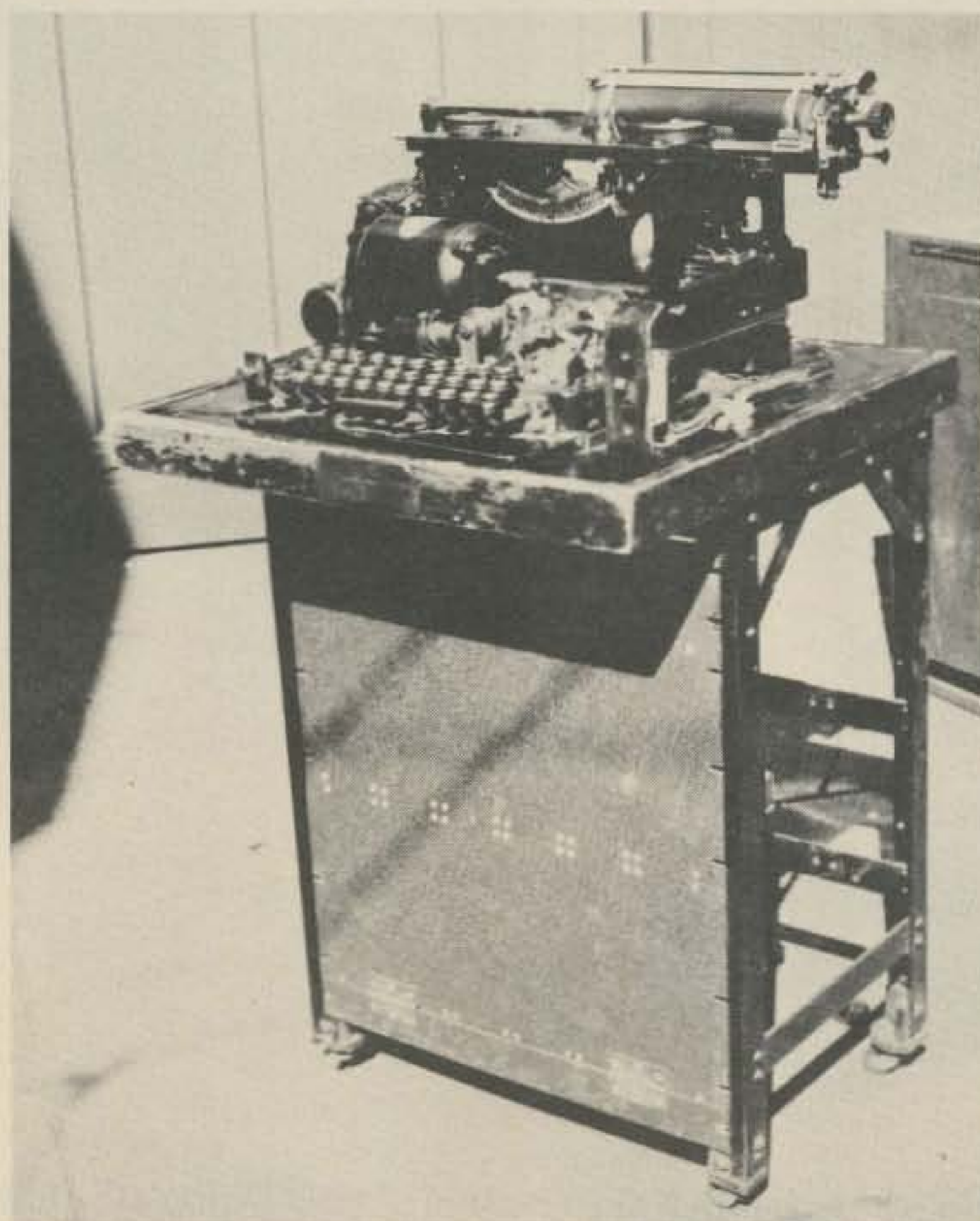
The old Model 12 "warhorse" Teletype machine... the printer that got amateur radio teletype started back in 1946.
