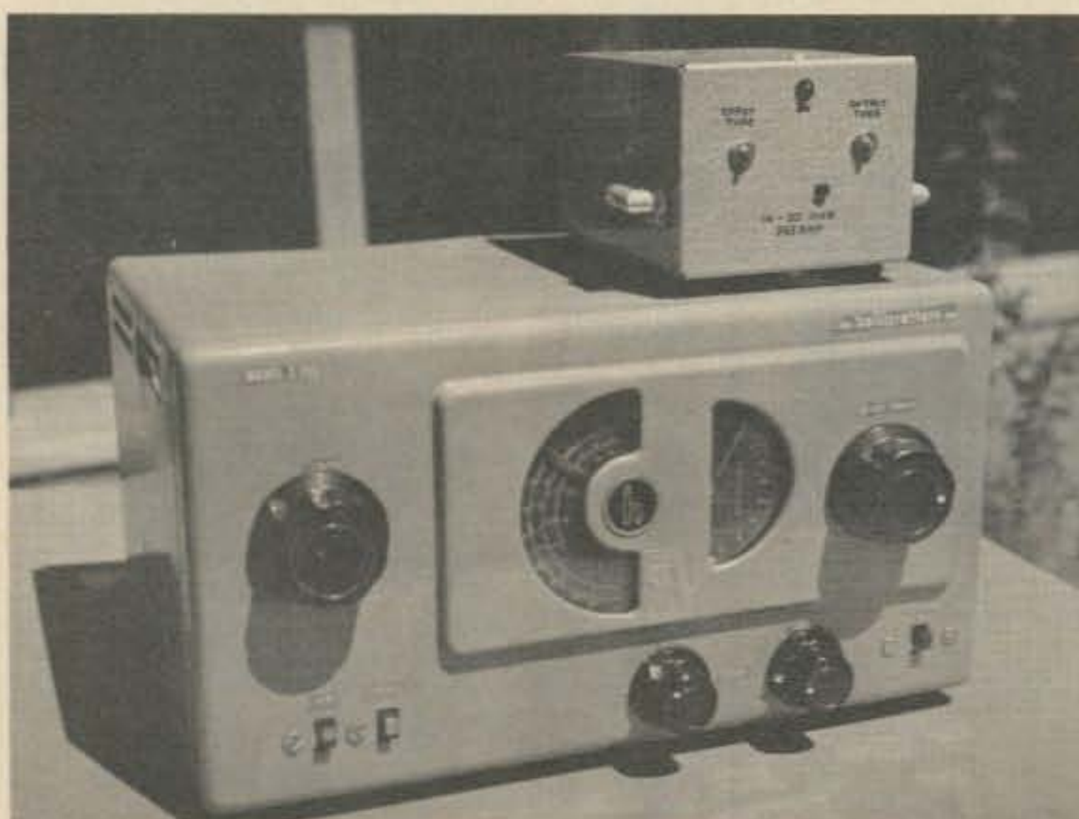
Hallicrafters S38C after resurrection, with FET preamp atop.
