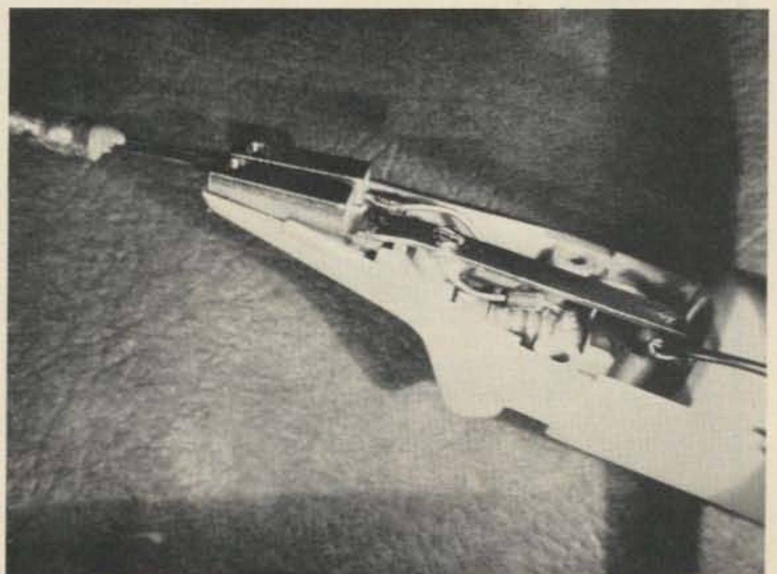
Interior view of iron, showing diode used to slightly drop lamp voltage.
