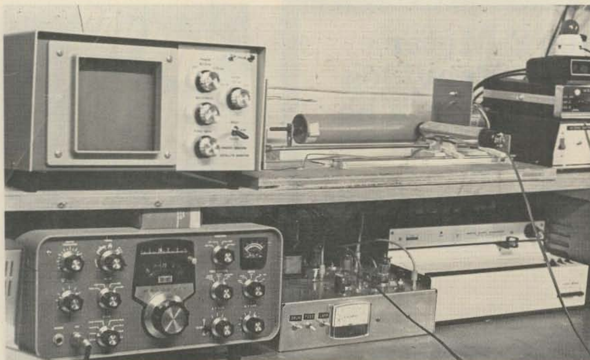
Fig. 6. The author's satellite station, where the monitor (upper right) and FAX display systems are integrated into a single display system. The actual FAX recorder is on the upper shelf to the right of the monitor. The lamp driver and drum amplifier circuits are on the chassis on the lower shelf next to the SB102. To the right of this chassis is a chart recorder (Heathkit), which records satellite signal levels during unattended station operation.
