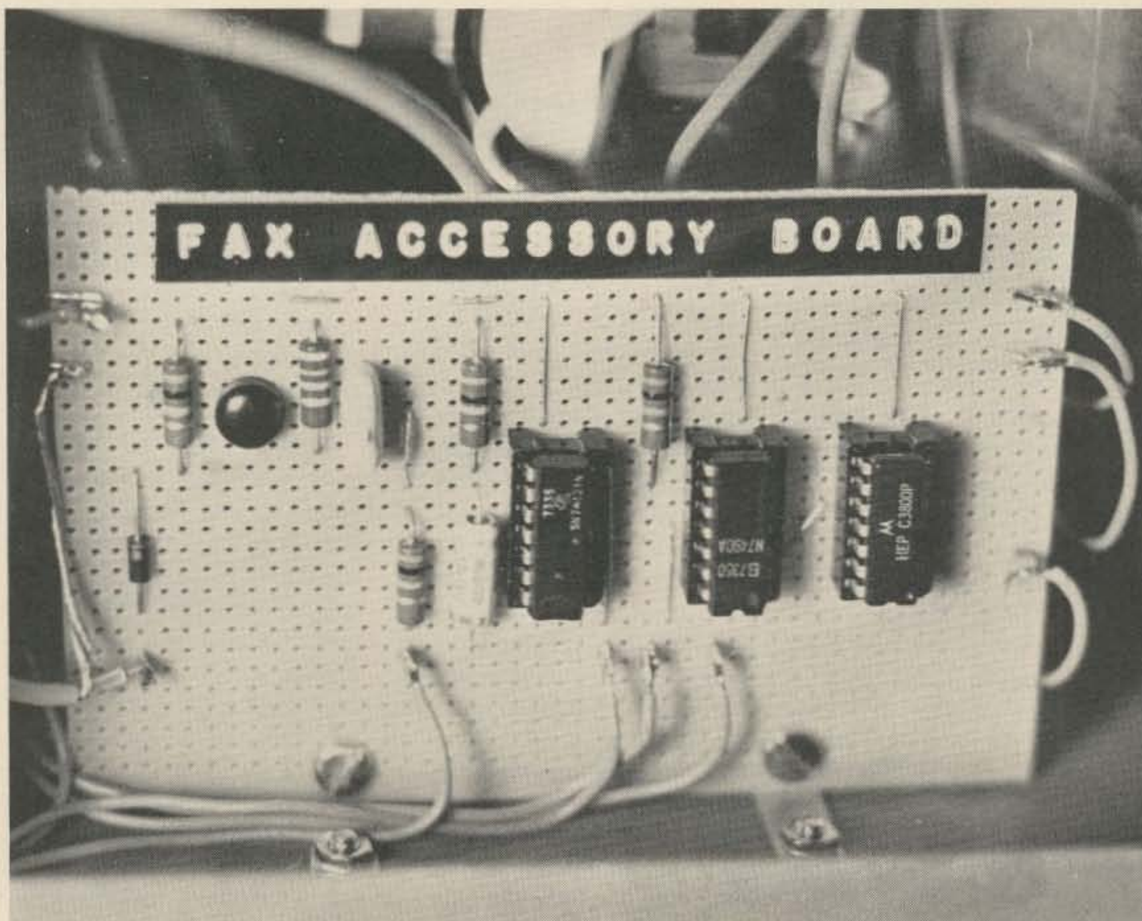
Fig. 1. Accessory FAX module installed in one of the author's multimode weather satellite monitors. A small piece of perforated board with 0.1 inch hole spacing accommodates the ICs and discrete components. Wiring the module itself takes about an hour and can be added to the monitor during or after construction.
