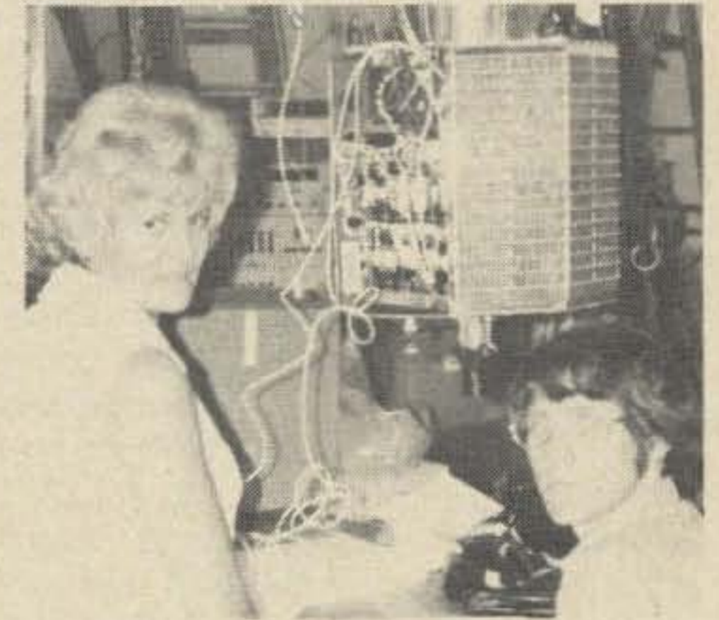
Marie Marr (AMSAT aerospace technician) and Jan King W3GEY A-O-B project manager prepare AMSAT-OSCAR B for solar simulation test.
